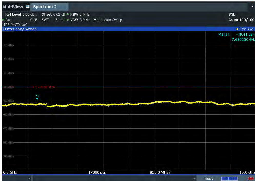
Plot 7-202. Conducted Spurious Emission at Antenna Port (75MHz Total Bandwidth 16QAM - Mid Channel, 6.5G ~ 15GHz)
