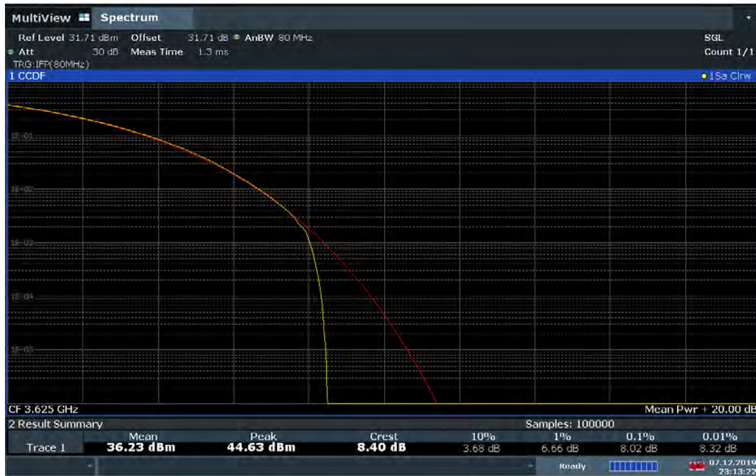
Plot 7-189. Common mode PAR Plot (75MHz Total Bandwidth QPSK - Mid Channel)
