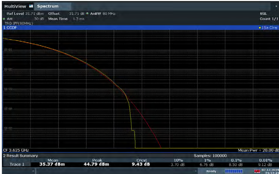
Plot 7-190. Common mode PAR Plot (75MHz Total Bandwidth 16QAM - Mid Channel)
