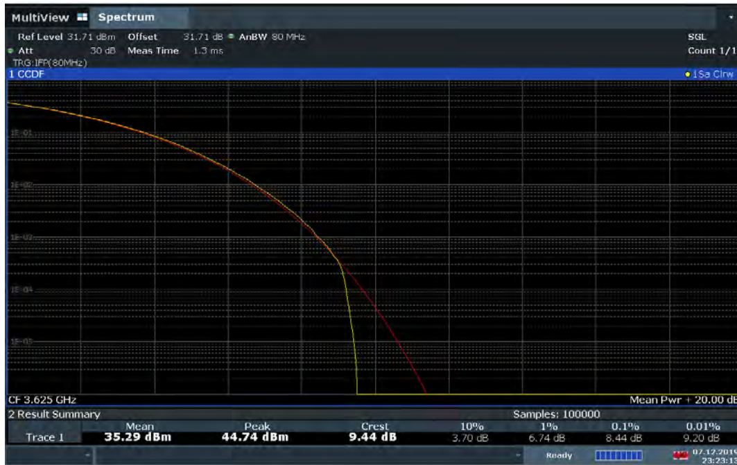
Plot 7-191. Common mode PAR Plot (75MHz Total Bandwidth 64QAM - Mid Channel)
