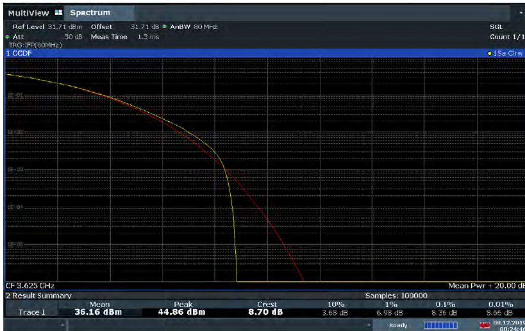
Plot 7-192. Common mode PAR Plot (75MHz Total Bandwidth 256QAM - Mid Channel)
