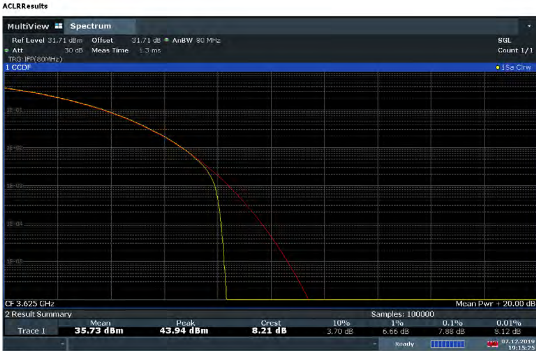
Plot 7-185. Common mode PAR Plot (65MHz Total Bandwidth QPSK - Mid Channel)
