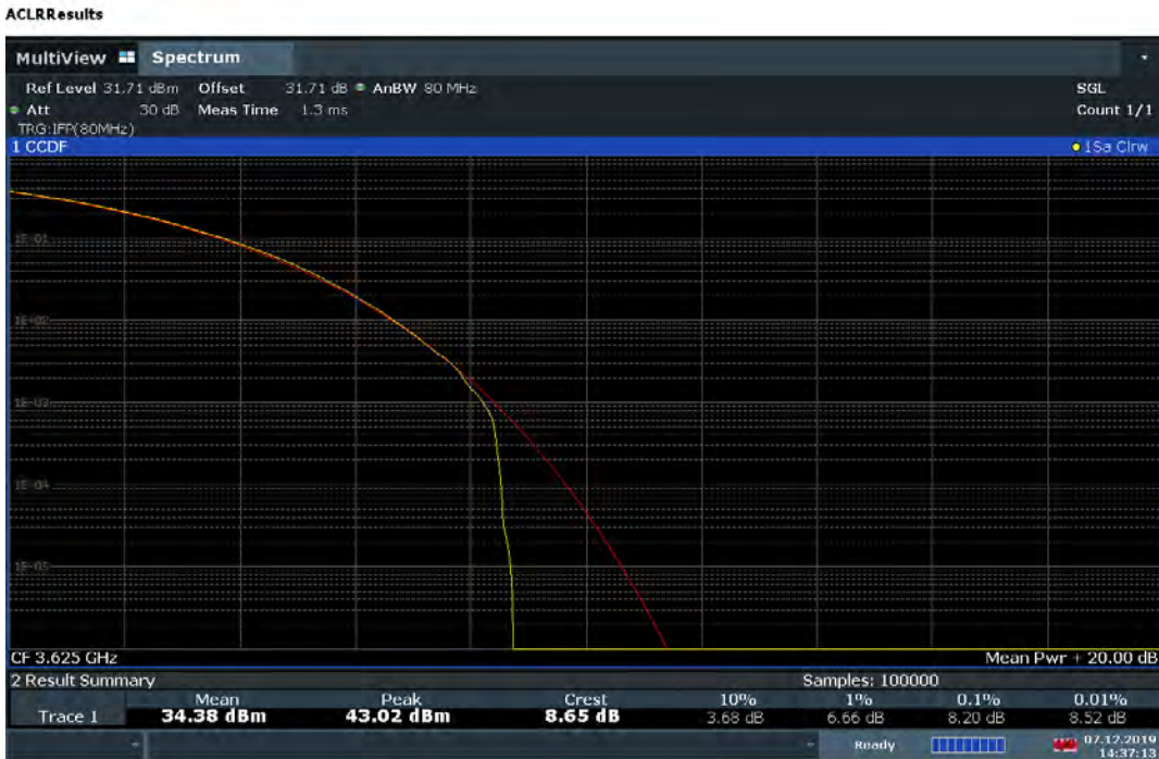
Plot 7-178. Common mode PAR Plot (45MHz Total Bandwidth 16QAM - Mid Channel)
