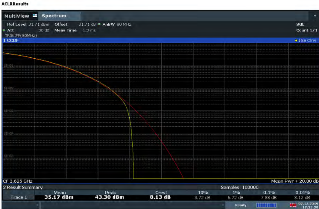
Plot 7-182. Common mode PAR Plot (55MHz Total Bandwidth 16QAM - Mid Channel)
