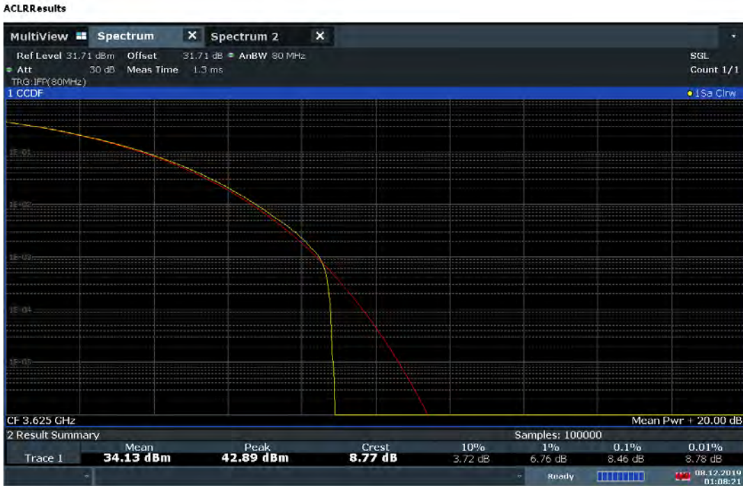
Plot 7-177. Common mode PAR Plot (45MHz Total Bandwidth QPSK - Mid Channel)
