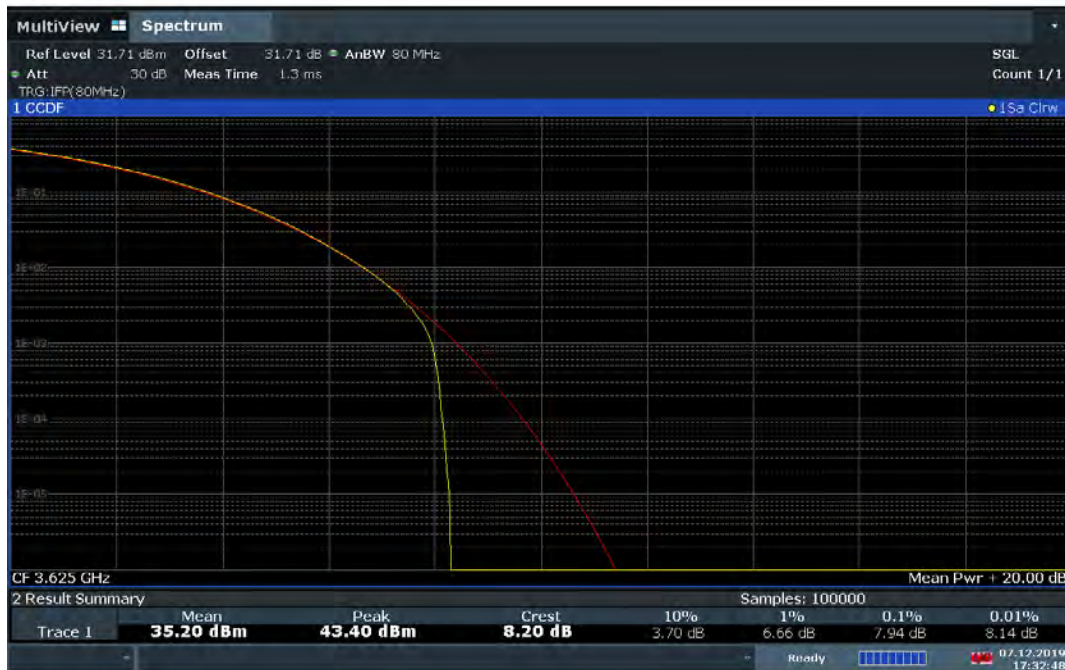
Plot 7-184. Common mode PAR Plot (55MHz Total Bandwidth 256QAM - Mid Channel)
