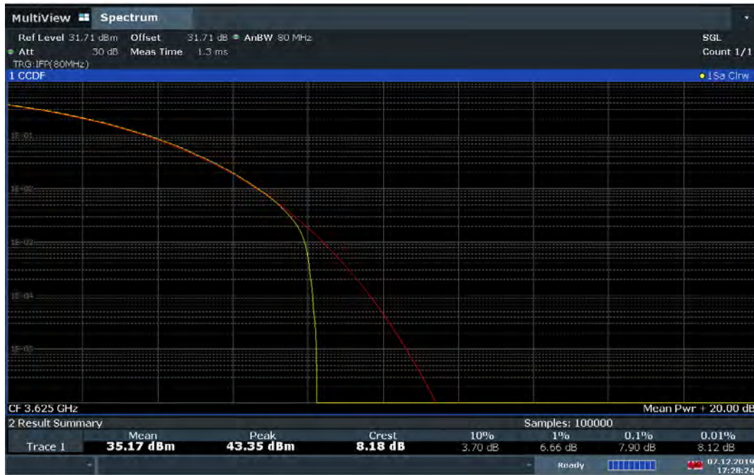
Plot 7-183. Common mode PAR Plot (55MHz Total Bandwidth 64QAM - Mid Channel)
