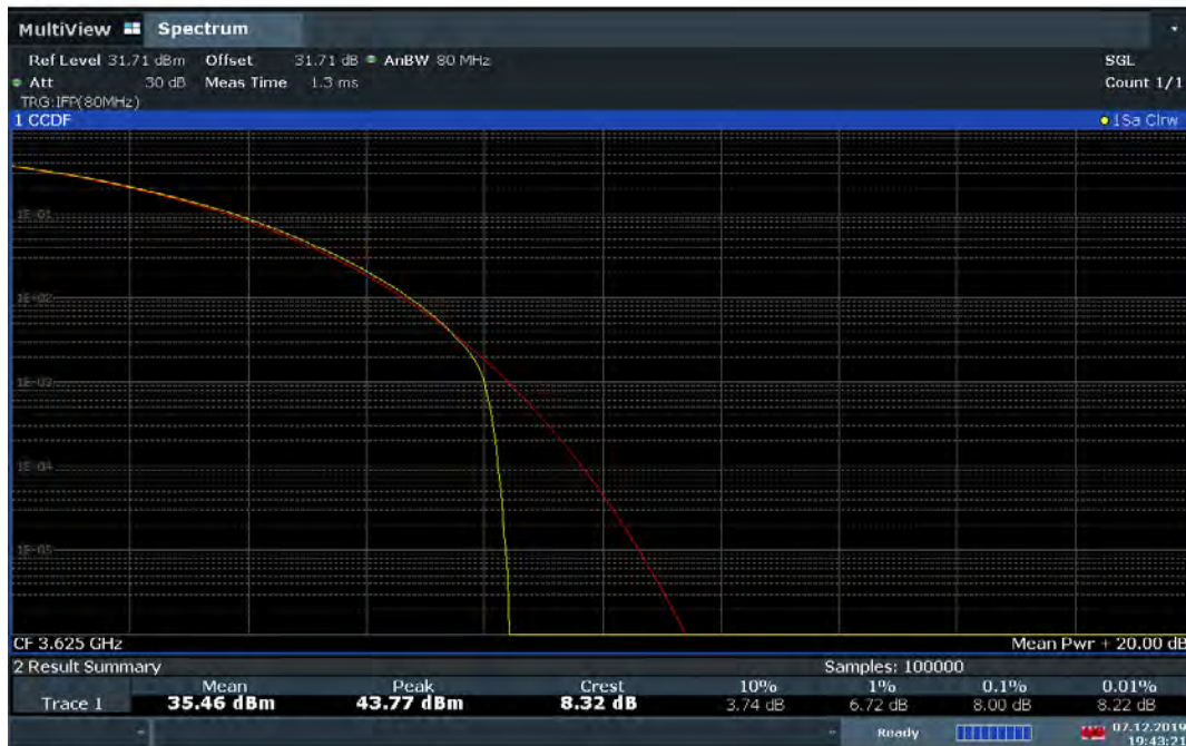
Plot 7-188. Common mode PAR Plot (65MHz Total Bandwidth 256QAM - Mid Channel)
