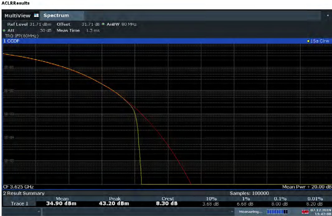
Plot 7-181. Common mode PAR Plot (55MHz Total Bandwidth QPSK - Mid Channel)
