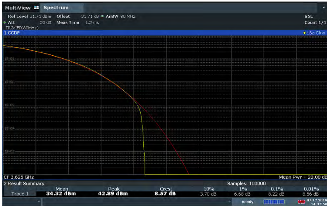
Plot 7-179. Common mode PAR Plot (45MHz Total Bandwidth 64QAM - Mid Channel)
