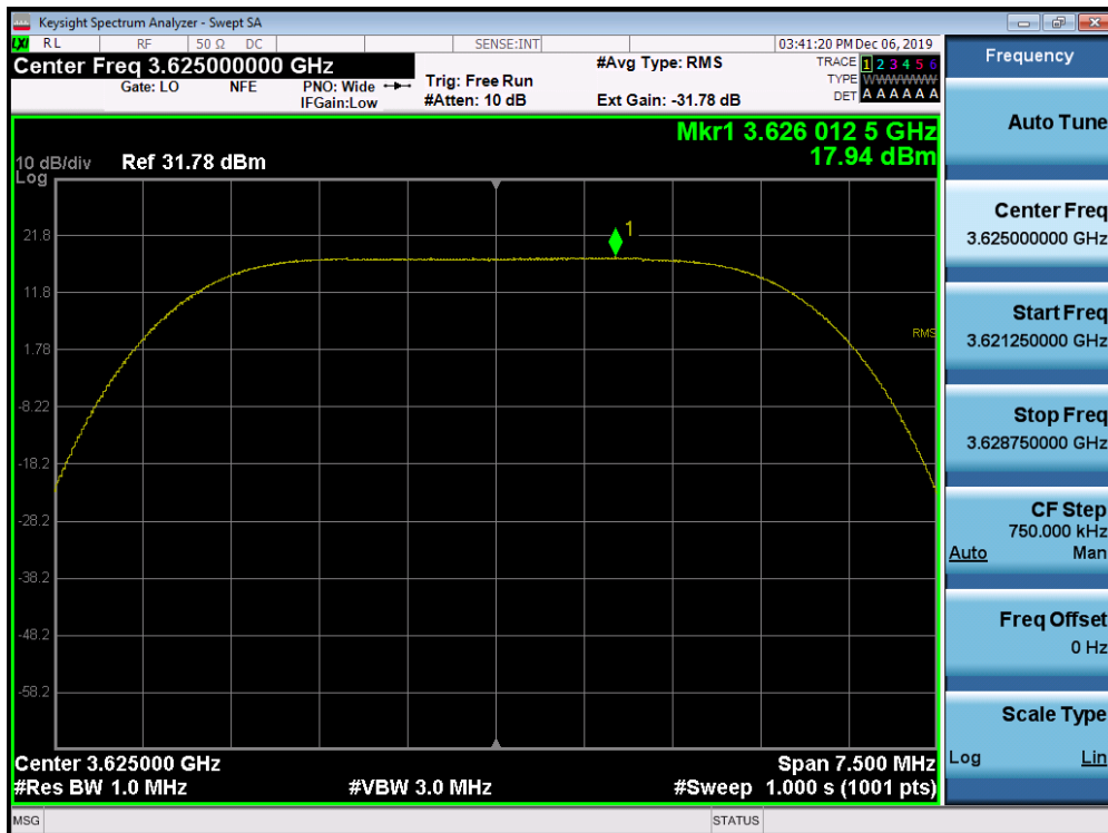
Plot 7-90. Peak Power Spectral Density Plot (1CC Configuration 5MHz 256QAM - Mid Channel) Port 01
