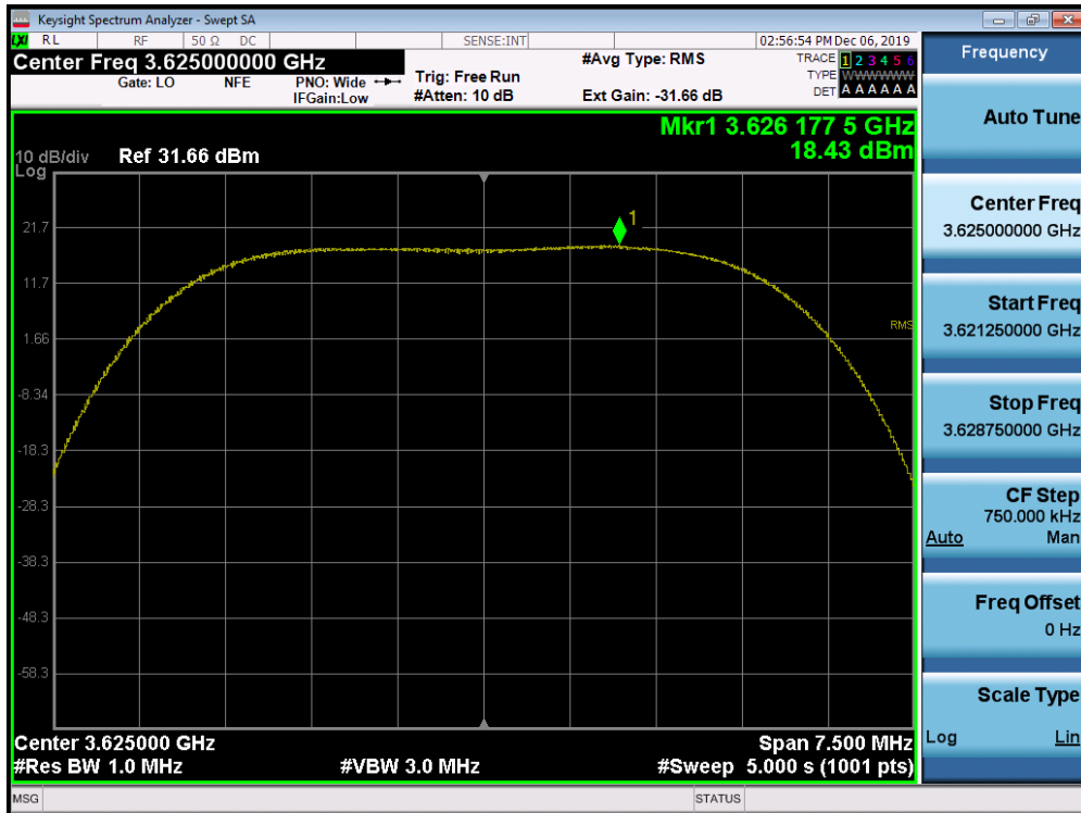
Plot 7-84. Peak Power Spectral Density Plot (1CC Configuration 5MHz 16QAM - Mid Channel) Port 03
