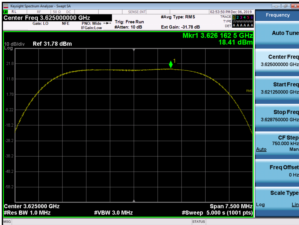
Plot 7-82. Peak Power Spectral Density Plot (1CC Configuration 5MHz 16QAM - Mid Channel) Port 01
