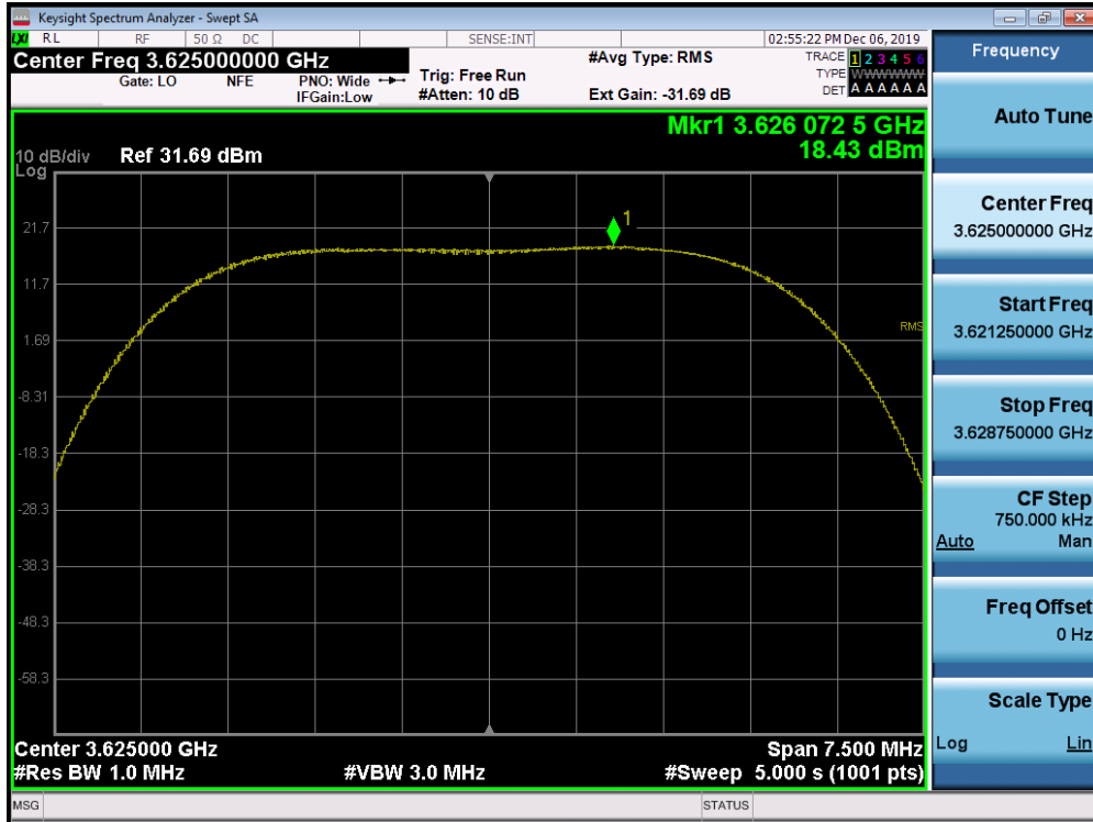
Plot 7-83. Peak Power Spectral Density Plot (1CC Configuration 5MHz 16QAM - Mid Channel) Port 02
