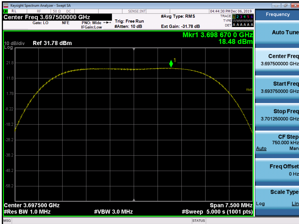
Plot 7-98. Peak Power Spectral Density Plot (1CC Configuration 5MHz 16QAM - High Channel) Port 01
