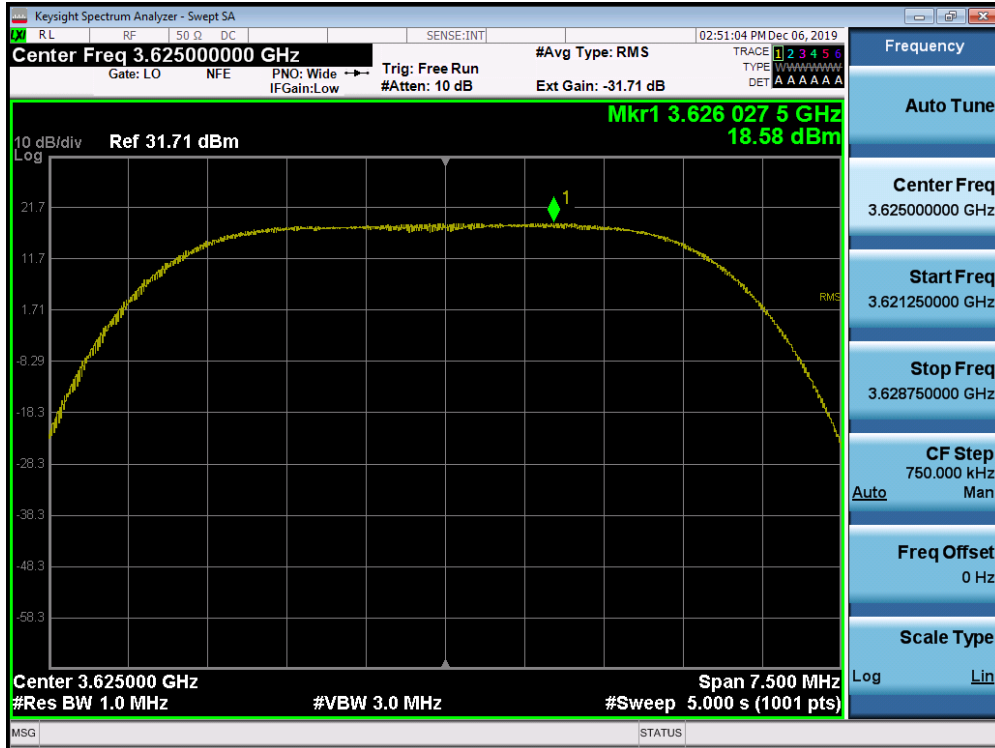
Plot 7-81. Peak Power Spectral Density Plot (1CC Configuration 5MHz 16QAM - Mid Channel) Port 00
