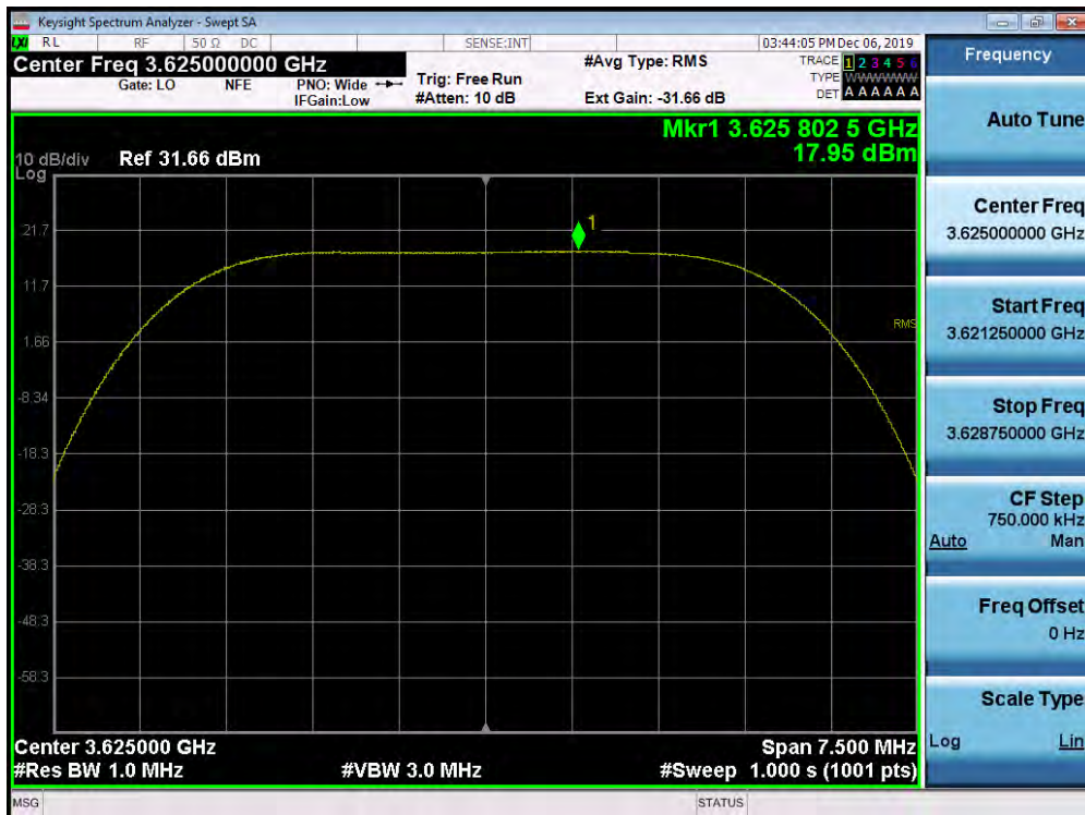
Plot 7-92. Peak Power Spectral Density Plot (1CC Configuration 5MHz 256QAM - Mid Channel) Port 03
