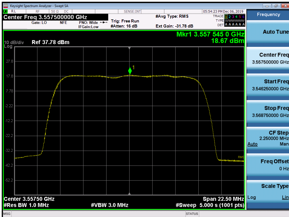
Plot 7-114. Peak Power Spectral Density Plot (1CC Configuration 15MHz 16QAM - Low Channel) Port 01
