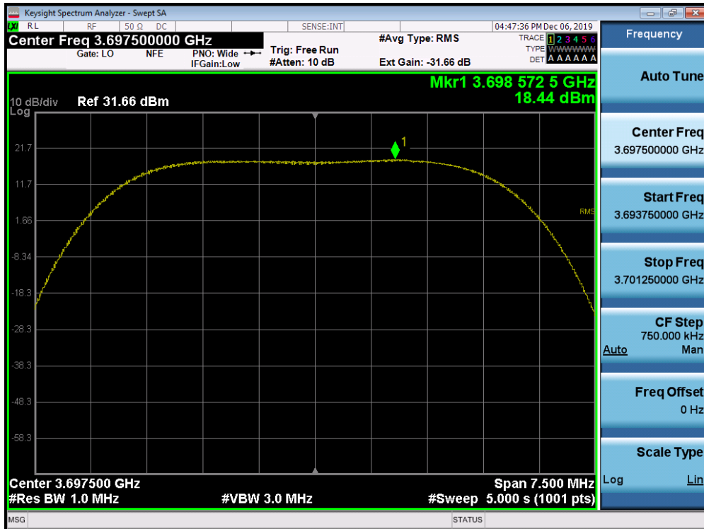
Plot 7-100. Peak Power Spectral Density Plot (1CC Configuration 5MHz 16QAM - High Channel) Port 03
