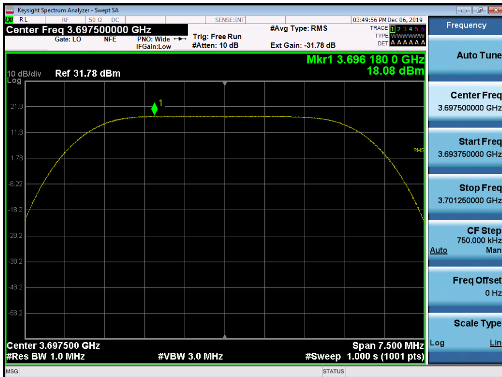
Plot 7-102. Peak Power Spectral Density Plot (1CC Configuration 5MHz 64QAM - High Channel) Port 01
