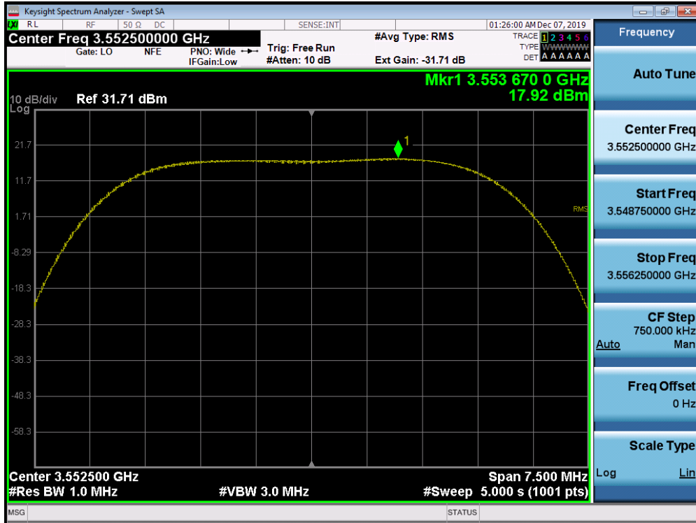
Plot 7-65. Peak Power Spectral Density Plot (1CC Configuration 5MHz 16QAM - Low Channel) Port 00
