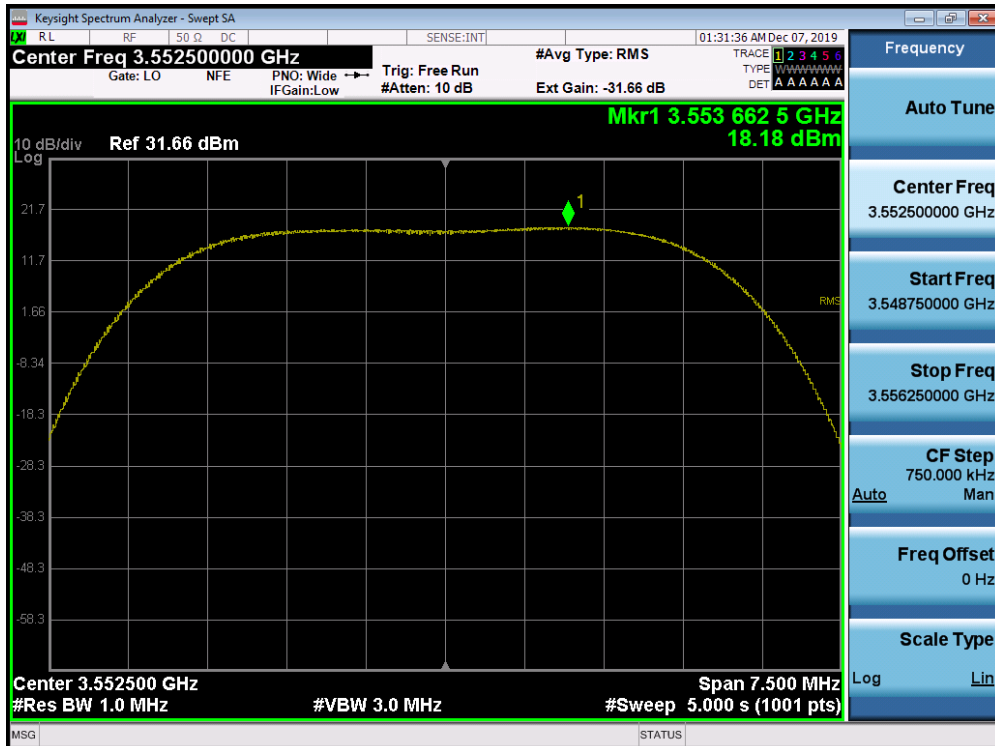
Plot 7-68. Peak Power Spectral Density Plot (1CC Configuration 5MHz 16QAM - Low Channel) Port 03
