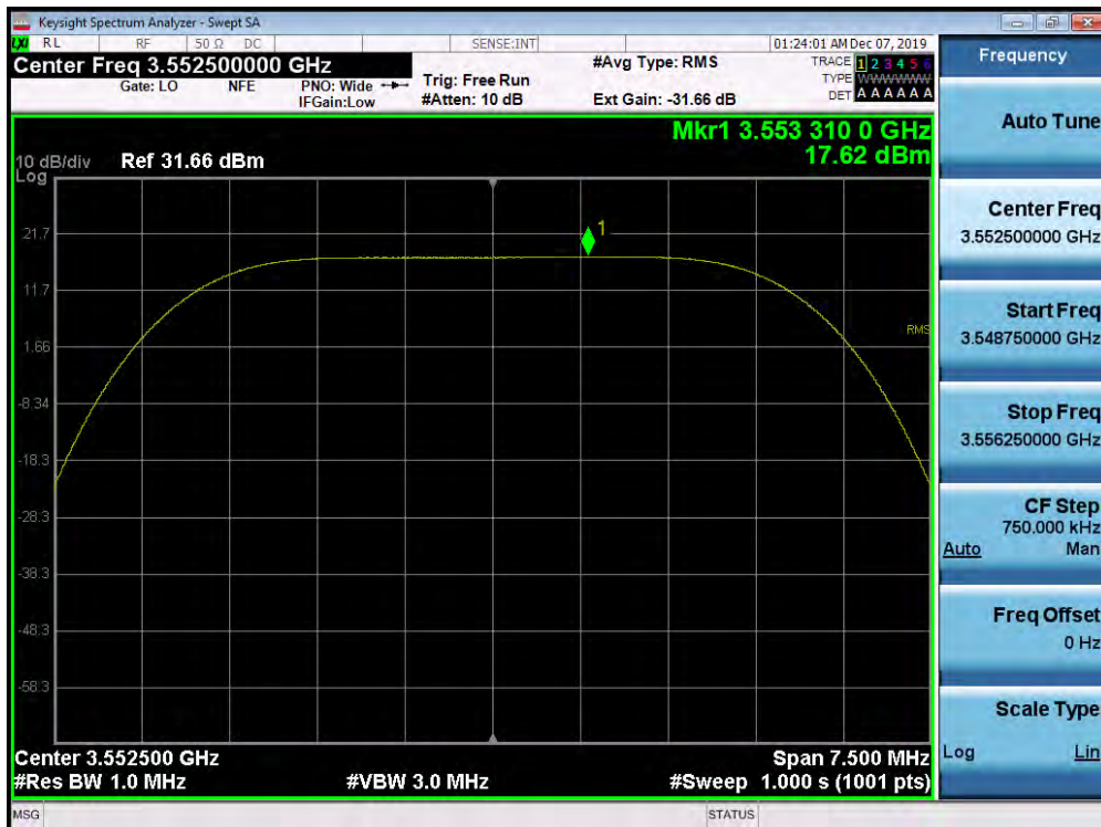
Plot 7-64. Peak Power Spectral Density Plot (1CC Configuration 5MHz QPSK - Low Channel) Port 03
