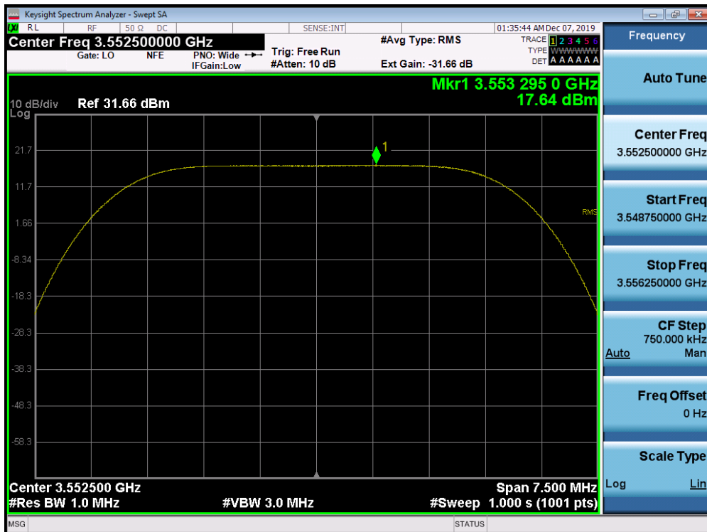
Plot 7-72. Peak Power Spectral Density Plot (1CC Configuration 5MHz 64QAM - Low Channel) Port 03
