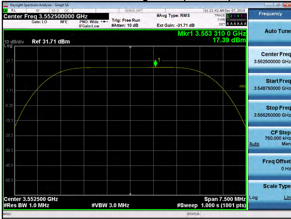
Plot 7-61. Peak Power Spectral Density Plot (1CC Configuration 5MHz QPSK - Low Channel) Port 00
