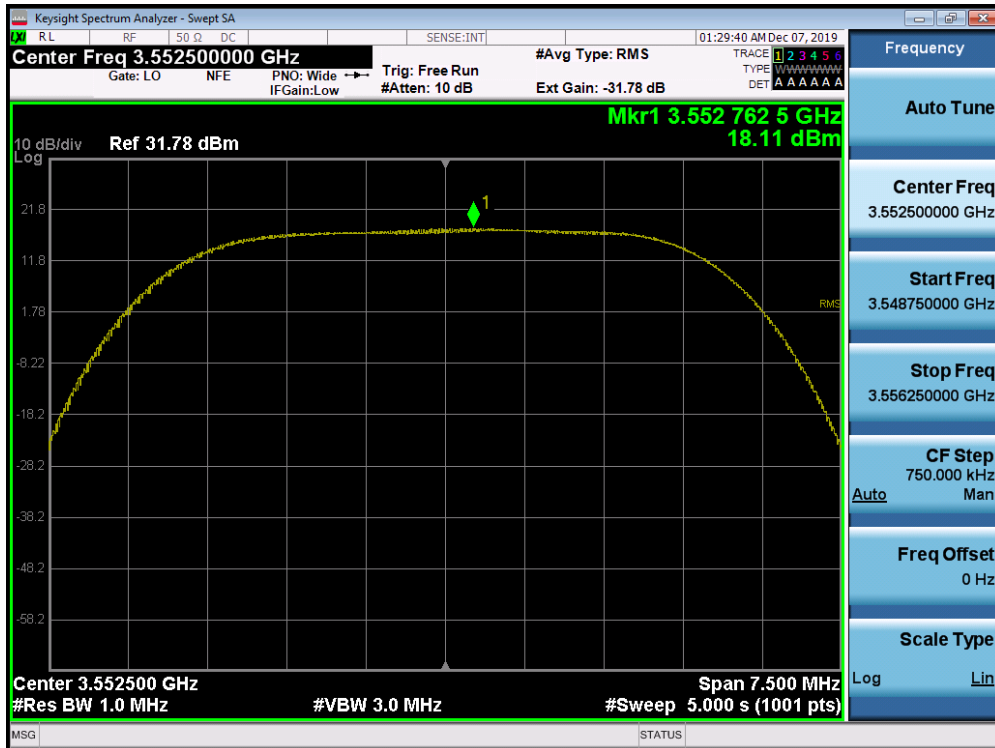
Plot 7-66. Peak Power Spectral Density Plot (1CC Configuration 5MHz 16QAM - Low Channel) Port 01
