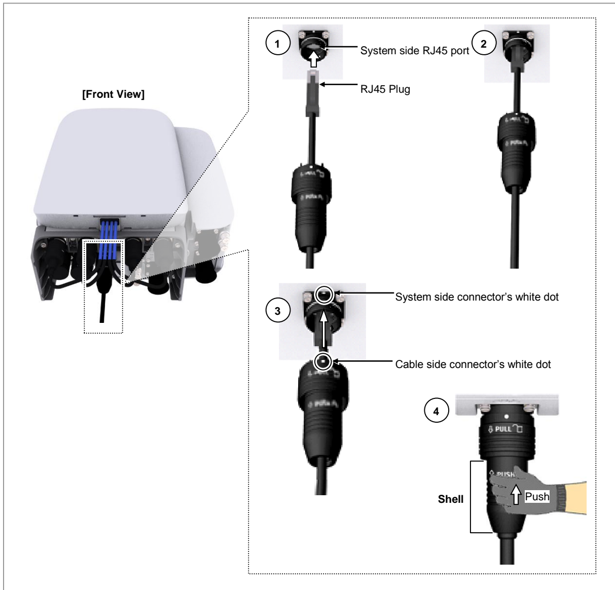
Figure 114. Connecting UDA Cable (4)
