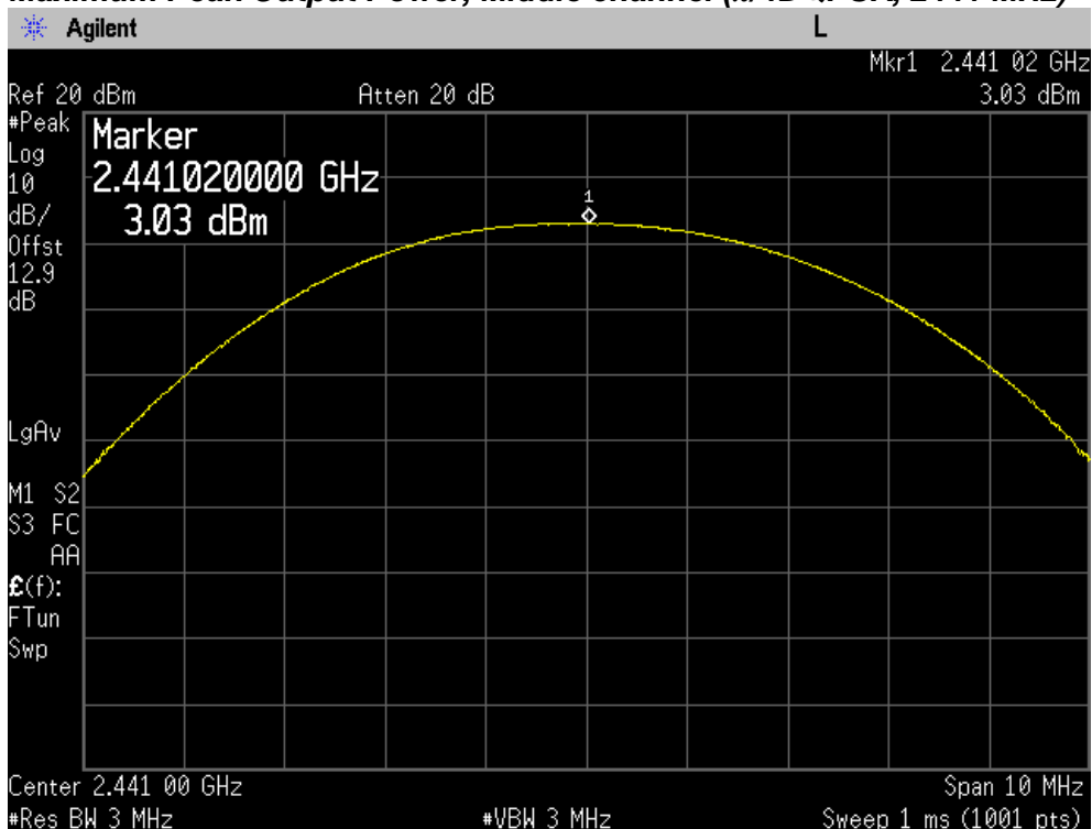
Maximum Peak Output Power, Middle channel ( \pi/4 DQPSK, 2441 MHz)
