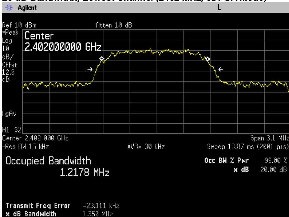
20 dB Bandwidth, Lowest Channel (2402 MHz, 8DPSK Mode)
