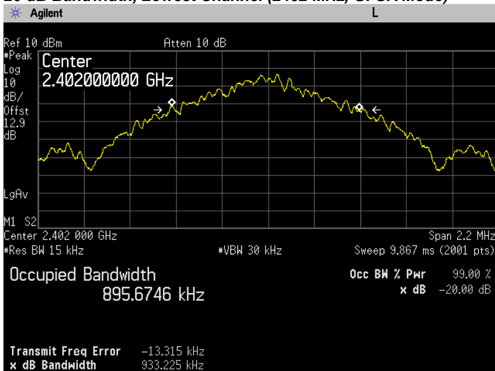
20 dB Bandwidth, Lowest Channel (2402 MHz, GFSK Mode)
