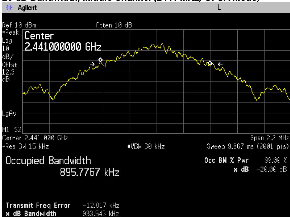
20 dB Bandwidth, Middle Channel (2441 MHz, GFSK Mode)
