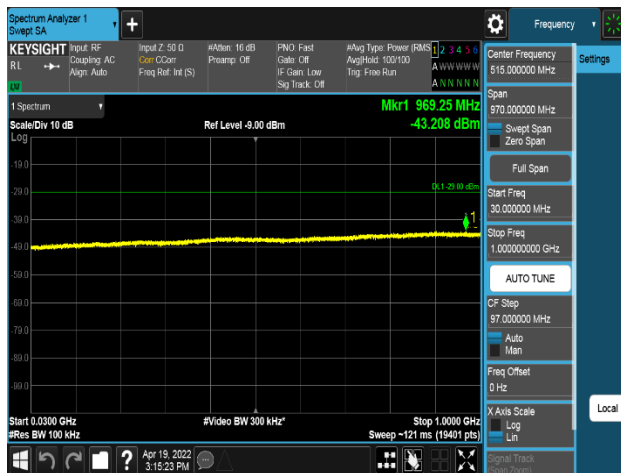
Plot 8-435. Conducted Spurious Emission Plot 30 MHz to 1 GHz (AWS_NR_1C_5M_4TX_64QAM - High Channel, Port 0)
