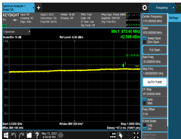
Plot 8-421. Conducted Spurious Emission Plot 30 MHz to 1 GHz (PCS_DSS_2C_10M + 15M_4TX_QPSK - Mid Channel, Port 0)
