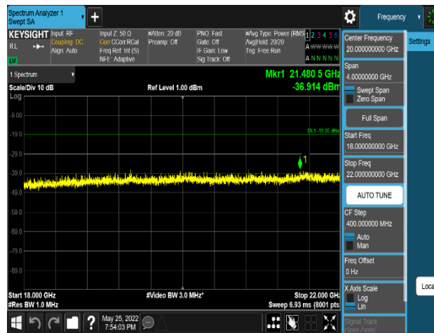
Plot 8-446. Conducted Spurious Emission Plot 18 GHz to 22 GHz (AWS_DSS_5:5_1C_20M_4TX_256QAM - High Channel, Port 0)
