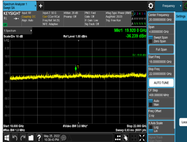
Plot 8-439. Conducted Spurious Emission Plot 18 GHz to 22 GHz (AWS_NR_1C_5M_4TX_64QAM - High Channel, Port 0)
