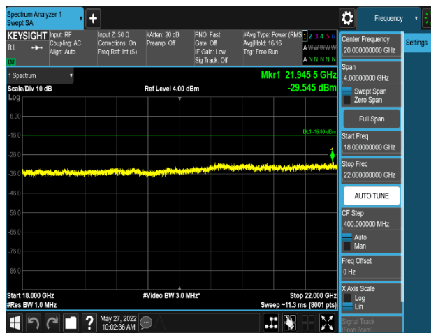
Plot 8-432. Peak To Average Power Ratio Plot 18 GHz to 22 GHz (PCS_NR_2C_5M + 5M_Non-Contiguous_4TX_QPSK - Mid Channel, Port 0)
