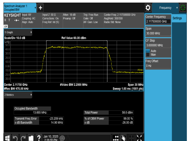
Plot 8-6. Occupied Bandwidth Plot (LTE_B66_1C_15M_16QAM - Low Channel, Port 1)
