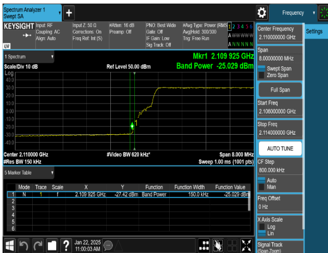
Plot 8-49. Band Edge Emission Summary Data Plot (LTE_B66_1C_15M_64QAM - Low Edge, Port 3)
