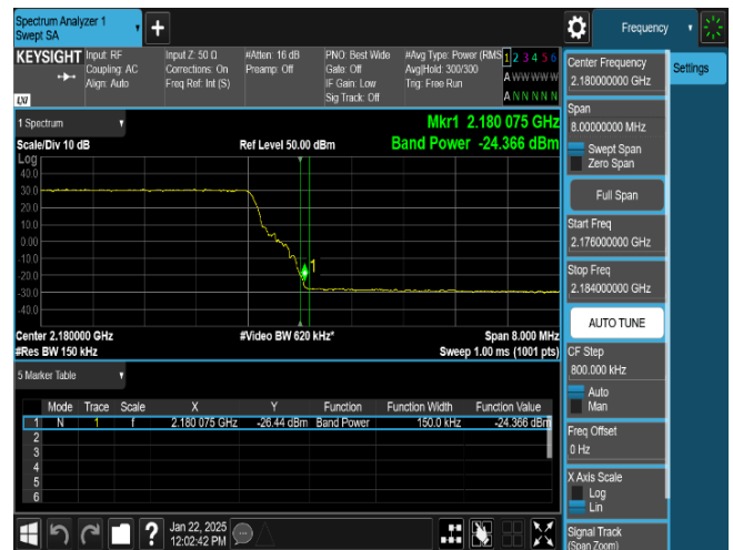
Plot 8-50. Band Edge Emission Summary Data Plot (LTE_B66_1C_15M_256QAM - High Edge, Port 0)
