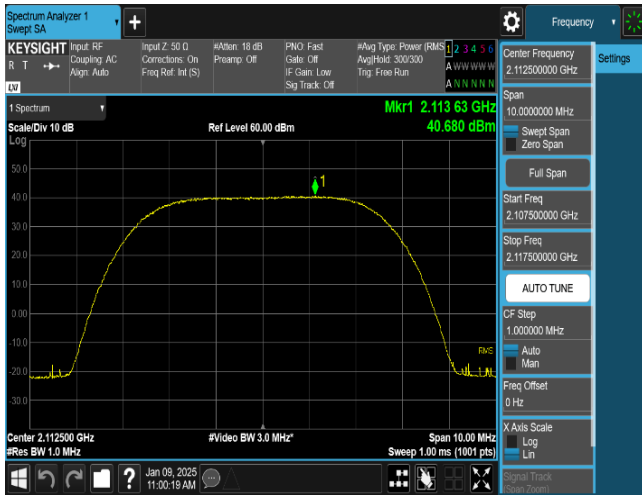
Plot 8-23. Equivalent Radiated Power Plot (LTE_B66_1C_5M_16QAM - Low Channel, Port 0)
