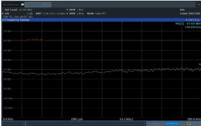
Plot 8-79. Conducted Spurious Emission Plot 9 kHz to 150 kHz (B5_1C_5M_QPSK - Low Channel, Port 0)
