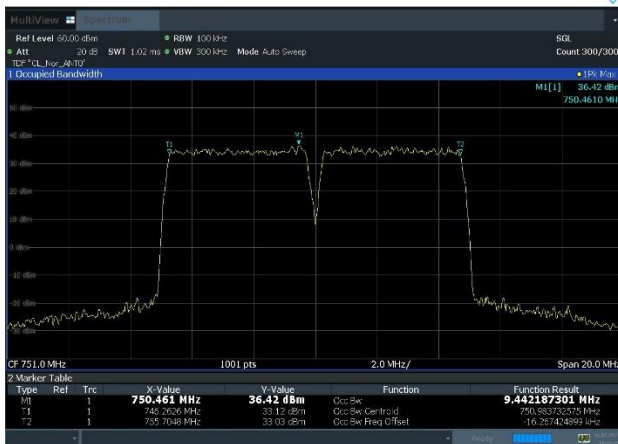
Plot 8-5. Occupied Bandwidth Plot (n13_2C_5M+5M_QPSK - Mid Channel, Port 0)
