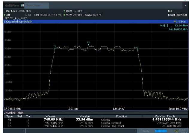
Plot 8-2. Occupied Bandwidth Plot (n13_1C_5M_16QAM - Low Channel, Port 0)
