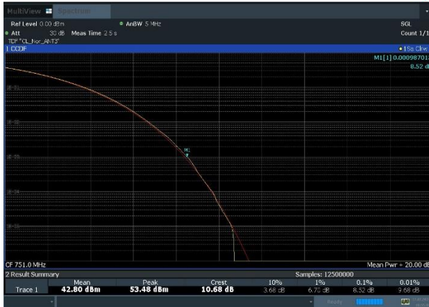
Plot 8-37. Peak To Average Power Ratio Plot (n13_1C_5M_64QAM - Mid Channel, Port 3)
