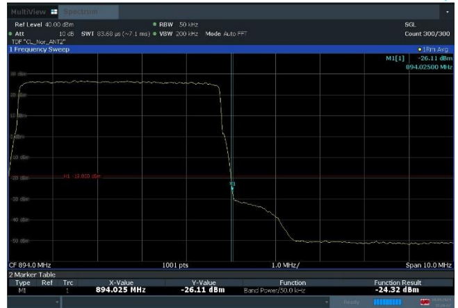
Plot 8-52. Band Edge Emission Summary Data Plot (n5_1C_5M_64QAM - High edge, Port 2)
