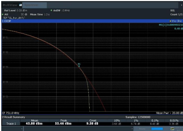
Plot 8-39. Peak To Average Power Ratio Plot (n13_2C_5M+5M_16QAM - Mid Channel, Port 1)
