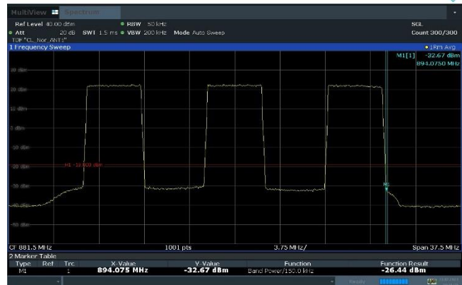
Plot 8-60. Band Edge Emission Summary Data Plot (Multi band operation n13_1C_10M + n5_3C_5M+5M+5M_QPSK - 2 nd carrier High Edge, Port 1)
