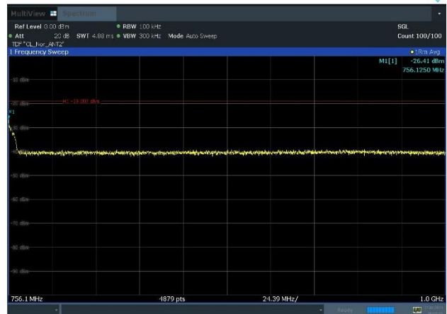
Plot 8-64. Conducted Spurious Emission Plot 756.1 MHz to 1 GHz (n13_1C_5M_256QAM - High Channel, Port 2)
