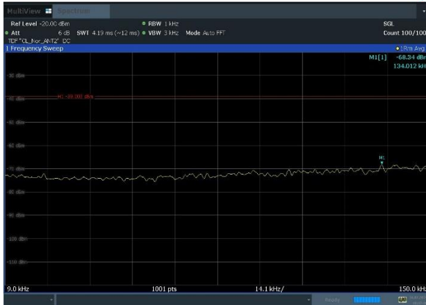
Plot 8-73. Conducted Spurious Emission Plot 9 kHz to 150 kHz (n13_2C_5M+5M_QPSK - Mid Channel, Port 2)
