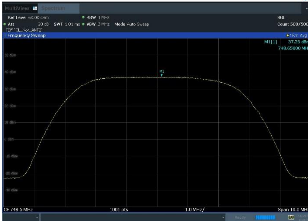
Plot 8-15. Equivalent Radiated Power Plot (n13_1C_5M_16QAM - Low Channel, Port 2)
