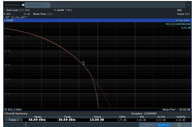
Plot 8-40. Peak To Average Power Ratio Plot (B5_1C_5M_256QAM - High Channel, Port 1)
