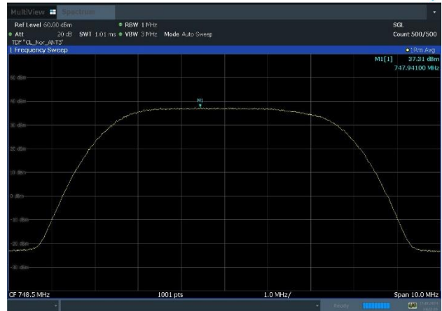
Plot 8-16. Equivalent Radiated Power Plot (n13_1C_5M_16QAM - Low Channel, Port 3)
