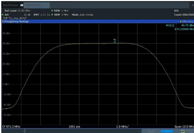
Plot 8-27. Equivalent Radiated Power Plot (B5_1C_5M_16QAM - Low Channel, Port 2)
