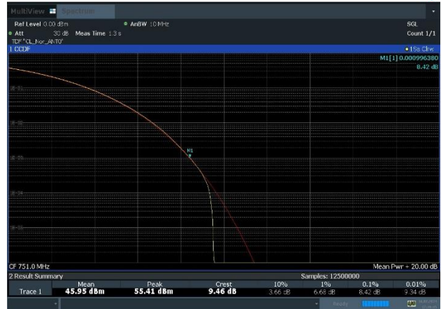
Plot 8-38. Peak To Average Power Ratio Plot (n13_1C_10M_64QAM - Mid Channel, Port 0)
