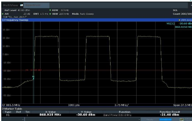
Plot 8-59. Band Edge Emission Summary Data Plot (Multi band operation n13_1C_10M + n5_3C_5M+5M+5M_QPSK - 2 nd carrier Low Edge, Port 1)
