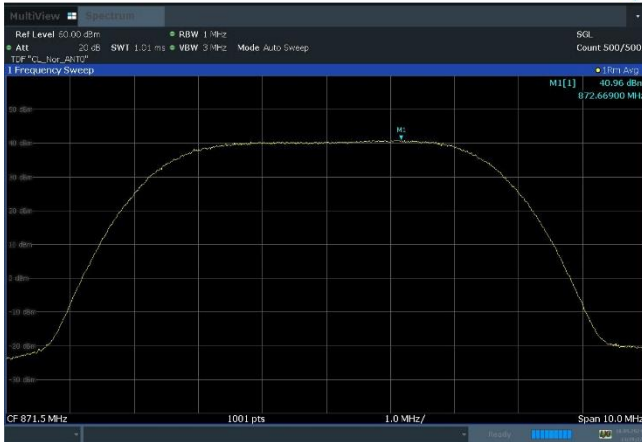
Plot 8-25. Equivalent Radiated Power Plot (B5_1C_5M_16QAM - Low Channel, Port 0)
