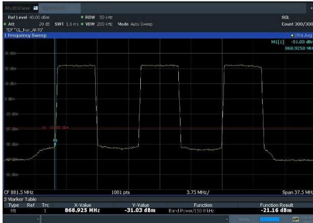
Plot 8-55. Band Edge Emission Summary Data Plot (n5_3NC_5M+5M+5M_QPSK - Low edge, Port 0)
