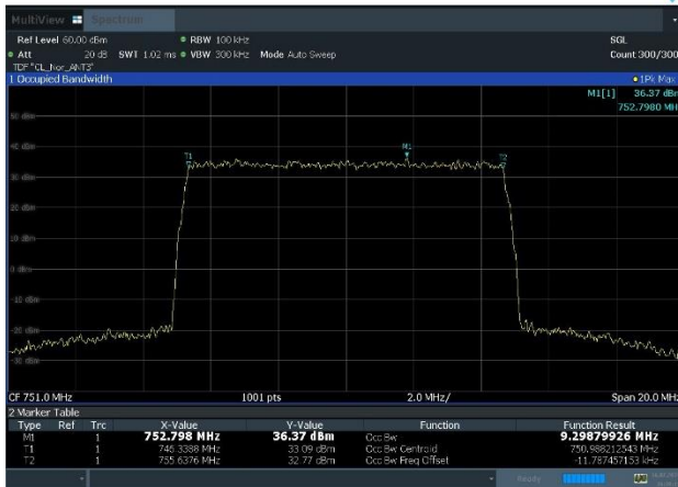
Plot 8-3. Occupied Bandwidth Plot (n13_1C_10M_QPSK - Mid Channel, Port 3)
