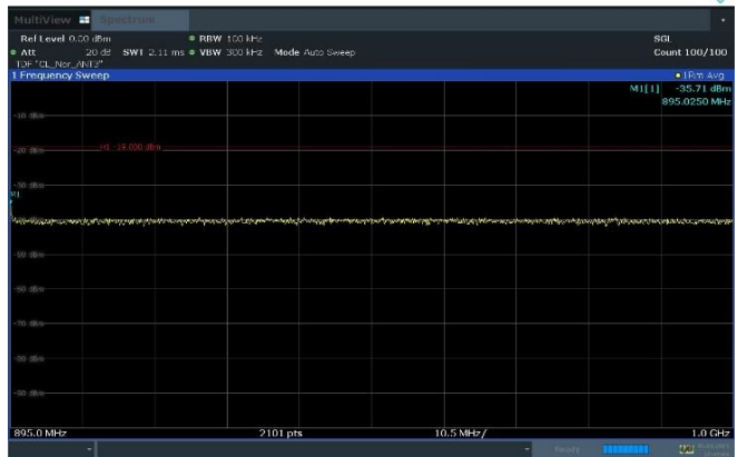
Plot 8-20. Conducted Spurious Emission Plot 895 MHz to 1 GHz (n5_1C_25M_4T_256QAM - Mid Channel, Port 3)
