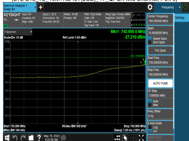
Plot 8-799. Conducted Spurious Emission Plot 735 MHz to 745.9 MHz (LTE B13_1C_10M+NB-IoT(2GB)_4T_QPSK-Mid Channel, Port 0)
