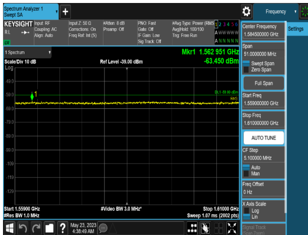
Plot 8-814. Conducted Spurious Emission Plot 1 559 MHz to 1 610 MHz (Multi-Band_LTE B13_2C_5M+5M+DSS B(n)5_1C_10M+NR n5_1C_10M+LTE B5_1C_5M_4T_QPSK-Middle+Low Channel, Port 2)
