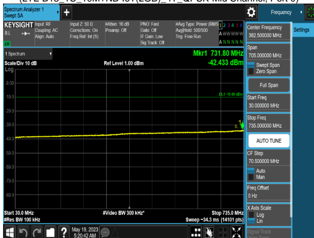
Plot 8-798. Conducted Spurious Emission Plot 30 MHz to 735 MHz (LTE B13_1C_10M+NB-IoT(2GB)_4T_QPSK-Mid Channel, Port 0)
