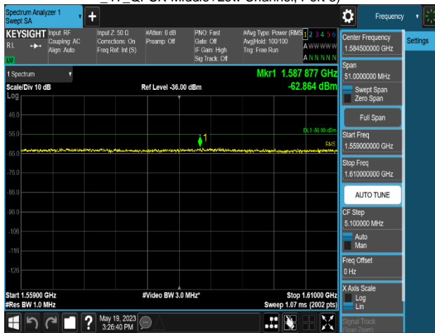
Plot 8-810. Conducted Spurious Emission Plot 1 559 MHz to 1 610 MHz (LTE B13_1C_10M_4T_QPSK-Middle Channel, Port 1)
