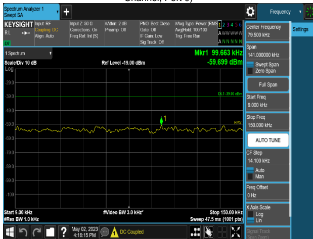
Plot 8-742. Conducted Spurious Emission Plot 9 kHz to 150 kHz (MSR 2C_DSS B(n)5_1C_10M+NR n5_1C_15M_4T_16QAM - Middle Channel, Port 0)
