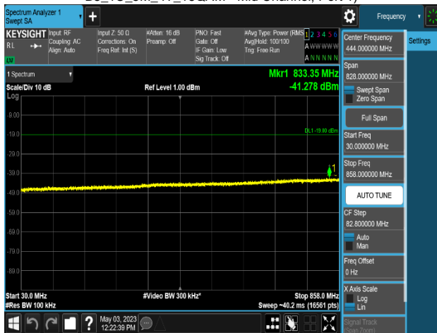
Plot 8-756. Conducted Spurious Emission Plot 30 MHz to 858 MHz (MSR 3C_DSS B(n)5_1C_10M+NR n5_1C_5M+LTE B5_1C_5M_4T_16QAM - Mid Channel, Port 1)
