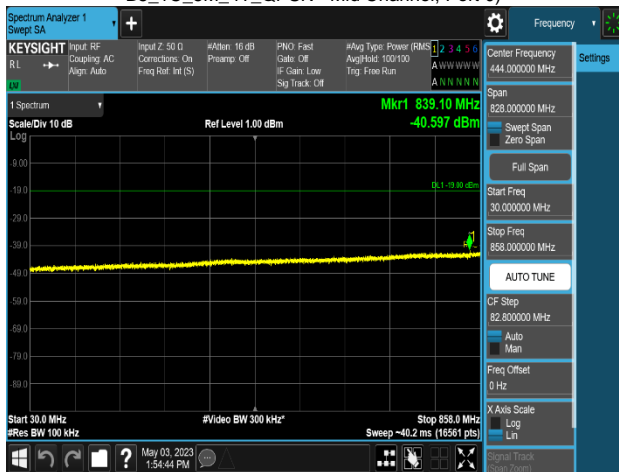
Plot 8-768. Conducted Spurious Emission Plot 30 MHz to 858 MHz (MSR 3NC_DSS B(n)5_1C_10M+NR n5_1C_5M+LTE B5_1C_5M_4T_QPSK - Mid Channel, Port 0)
