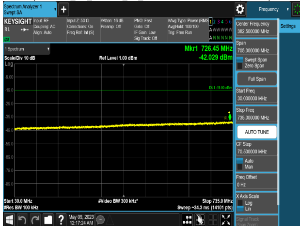
Plot 8-786. Conducted Spurious Emission Plot 30 MHz to 735 MHz (LTE B13_2C_5M+5M_4T_QPSK - Middle Channel, Port 0)
