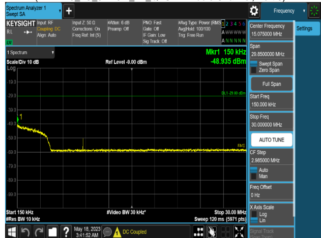
Plot 8-791. Conducted Spurious Emission Plot 150 kHz to 30 MHz (LTE B13_1C_5M+NB-IoT(1B)_4T_QPSK-High Channel, Port 0)
