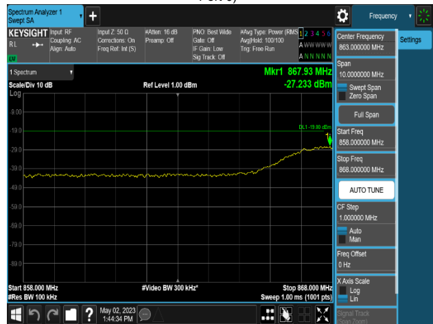
Plot 8-733. Conducted Spurious Emission Plot 858 MHz to 868 MHz (MSR 2NC_NR n5_1C_5M+LTE B5_1C_5M_4T_QPSK - Mid Channel, Port 0)
