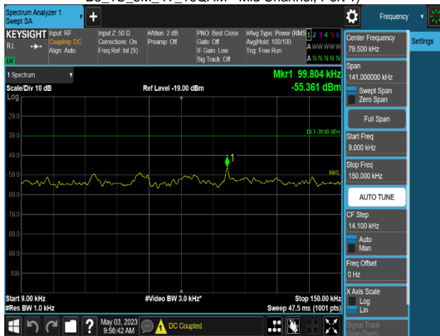
Plot 8-760. Conducted Spurious Emission Plot 9 kHz to 150 kHz (MSR 3C_DSS B(n)5_1C_10M+NR n5_1C_10M+LTE B5_1C_5M_4T_16QAM - Mid Channel, Port 0)
