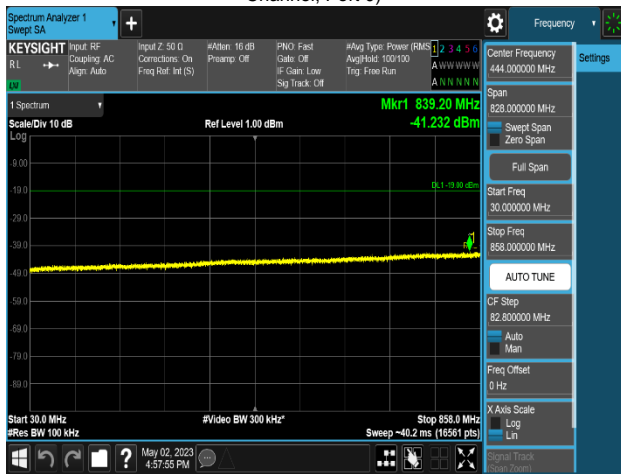
Plot 8-738. Conducted Spurious Emission Plot 30 MHz to 858 MHz (MSR 2C_DSS B(n)5_1C_10M+NR n5_1C_5M_4T_QPSK - Low Channel, Port 0)
