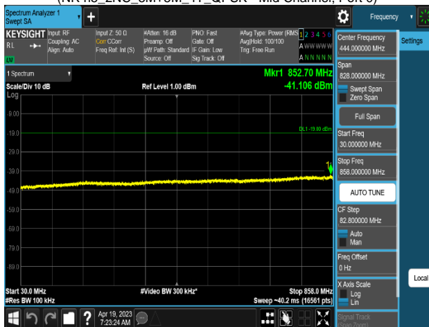
Plot 8-696. Conducted Spurious Emission Plot 30 MHz to 858 MHz (NR n5_2NC_5M+5M_4T_QPSK - Mid Channel, Port 0)
