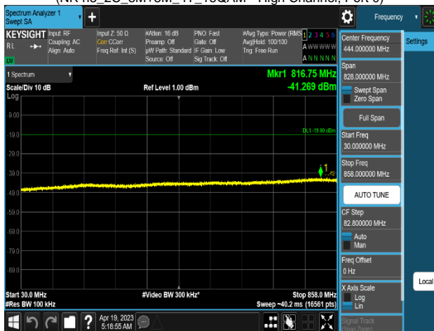
Plot 8-684. Conducted Spurious Emission Plot 30 MHz to 858 MHz (NR n5_2C_5M+5M_4T_16QAM - High Channel, Port 0)
