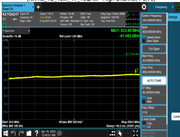
Plot 8-678. Conducted Spurious Emission Plot 30 MHz to 858 MHz (NR n5_1C_15M_4T_16QAM - High Channel, Port 0)
