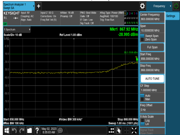
Plot 8-715. Conducted Spurious Emission Plot 858 MHz to 868 MHz (MSR 2NC_DSS B(n)5_1C_10M+LTE B5_1C_5M_4T_QPSK - Middle Channel, Port 0)
