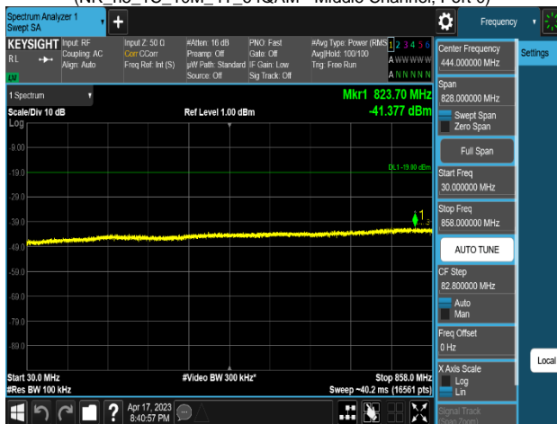
Plot 8-672. Conducted Spurious Emission Plot 30 MHz to 858 MHz (NR_n5_1C_10M_4T_64QAM - Middle Channel, Port 0)
