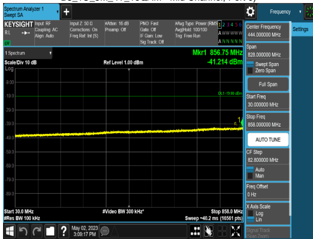
Plot 8-726. Conducted Spurious Emission Plot 30 MHz to 858 MHz (MSR 3C_DSS B(n)5_1C_10M+NR n5_1C_10M+LTE B5_1C_5M_4T_16QAM - Mid Channel, Port 0)
