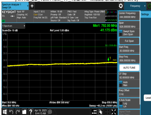
Plot 8-690. Conducted Spurious Emission Plot 30 MHz to 858 MHz (NR n5_2C_10M+15M_4T_16QAM - Middle Channel, Port 0)
