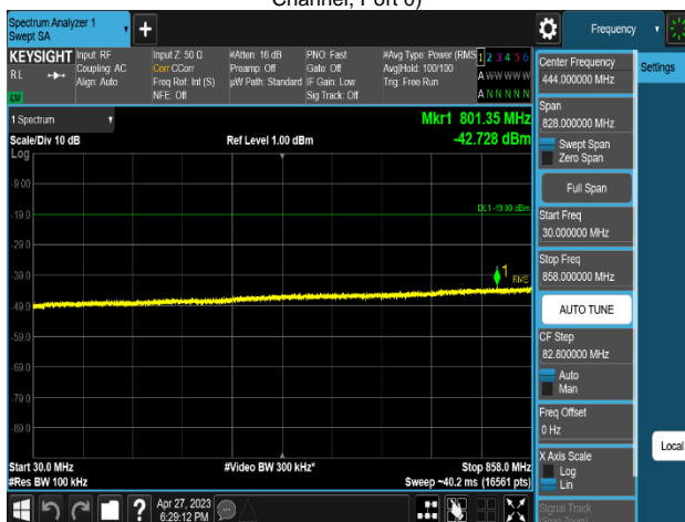
Plot 8-702. Conducted Spurious Emission Plot 30 MHz to 858 MHz (MSR 2C_DSS B(n)5_1C_10M+LTE B5_1C_5M_4T_QPSK - High Channel, Port 0)
