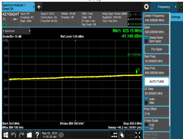
Plot 8-720. Conducted Spurious Emission Plot 30 MHz to 858 MHz (MSR 2C_NR n5_1C_5M+LTE B5_1C_5M_4T_QPSK - Low Channel, Port 0)
