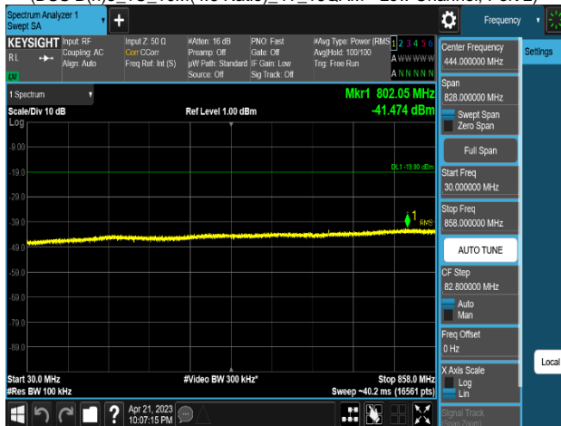
Plot 8-648. Conducted Spurious Emission Plot 30 MHz to 858 MHz (DSS B(n)5_1C_10M(4:6 Ratio)_4T_16QAM - Low Channel, Port 2)
