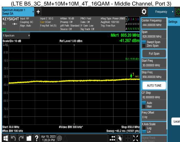
Plot 8-636. Conducted Spurious Emission Plot 30 MHz to 858 MHz (LTE B5_3C_5M+10M+10M_4T_16QAM - Middle Channel, Port 3)
