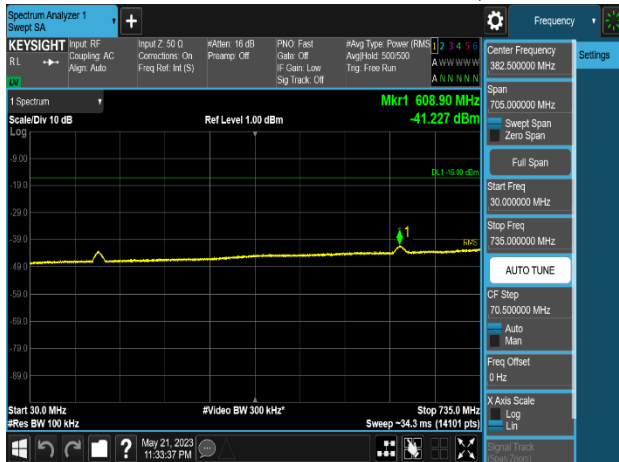
Plot 8-605. Conducted Spurious Emission Plot 30 MHz to 735 MHz (Multi-Band_LTE_B13_1C_10M+NB-IoT(2GB)+LTE_B5_10M_1C _2T_QPSK-Middle+Low Channel, Port 1)
