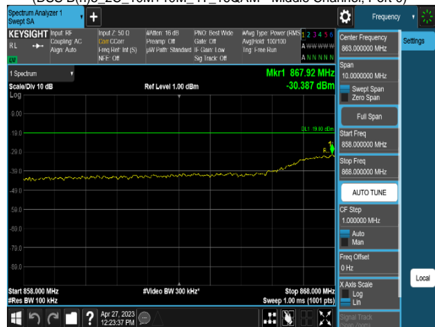
Plot 8-655. Conducted Spurious Emission Plot 858 MHz to 868 MHz
