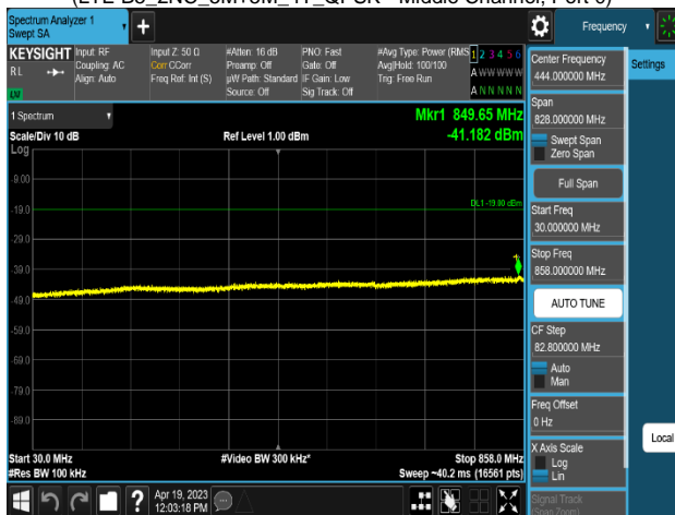
Plot 8-642. Conducted Spurious Emission Plot 30 MHz to 858 MHz
