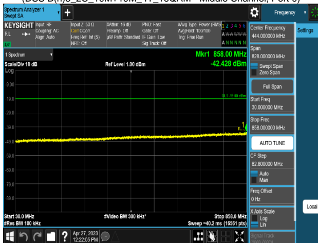
Plot 8-654. Conducted Spurious Emission Plot 30 MHz to 858 MHz
