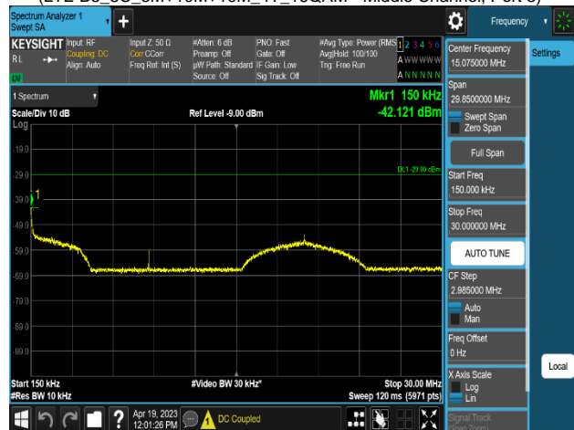
Plot 8-641. Conducted Spurious Emission Plot 150 kHz to 30 MHz
