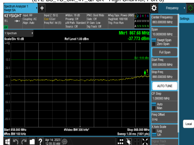
Plot 8-619. Conducted Spurious Emission Plot 858 MHz to 868 MHz (LTE B5_1C_5M_4T_QPSK - High Channel, Port 3)
