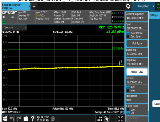
Plot 8-630. Conducted Spurious Emission Plot 30 MHz to 858 MHz (LTE B5_2C_5M+5M_4T_16QAM - Middle Channel, Port 1)
