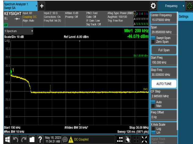
Plot 8-592. Conducted Spurious Emission Plot 150 kHz to 30 MHz
