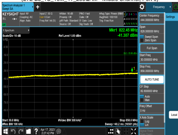
Plot 8-624. Conducted Spurious Emission Plot 30 MHz to 858 MHz (LTE B5_1C_10M_4T_256QAM - Middle Channel, Port 0)
