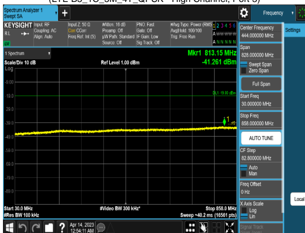
Plot 8-618. Conducted Spurious Emission Plot 30 MHz to 858 MHz (LTE B5_1C_5M_4T_QPSK - High Channel, Port 3)
