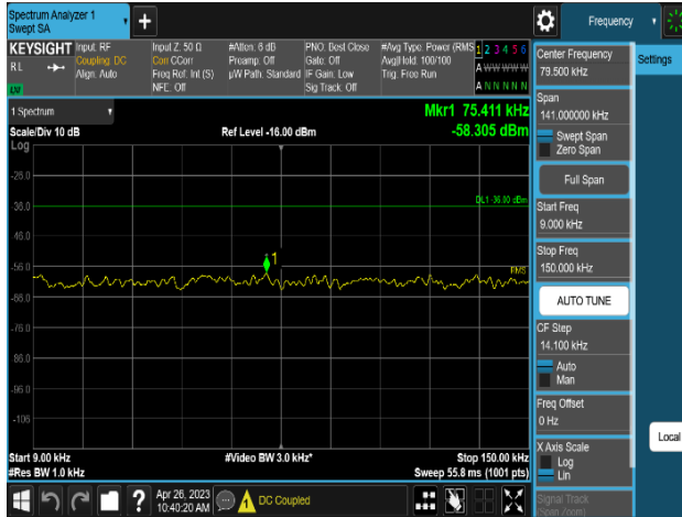
Plot 8-537. Conducted Spurious Emission Plot 9 kHz to 150 kHz (MSR 2C_DSS B(n)5_1C_10M+NR n5_1C_5M_2T_QPSK - Low Channel, Port 0)
