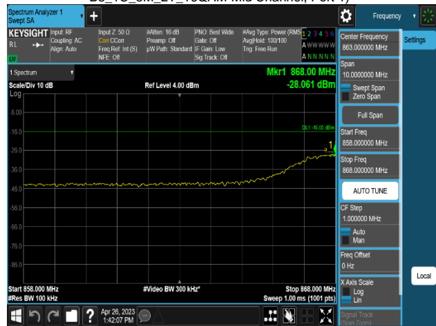
Plot 8-564. Conducted Spurious Emission Plot 858 MHz to 868 MHz (MSR 3C_DSS B(n)5_1C_10M+NR n5_1C_10M+LTE B5_1C_5M_2T_16QAM-Mid Channel, Port 1)
