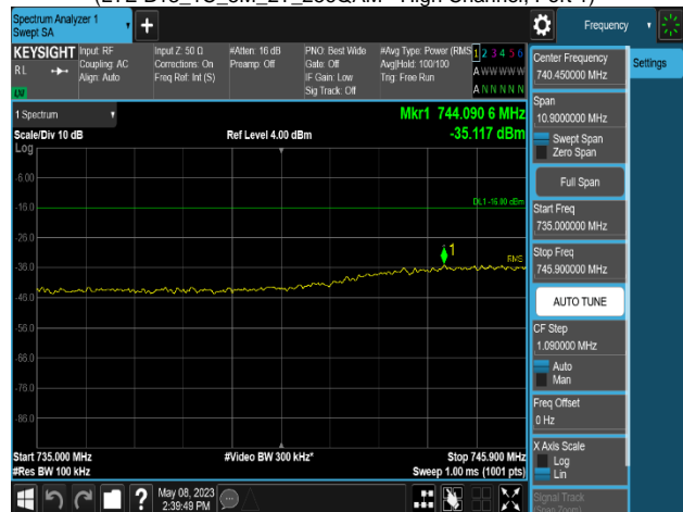
Plot 8-576. Conducted Spurious Emission Plot 735 MHz to 745.9 MHz (LTE B13_1C_5M_2T_256QAM - High Channel, Port 1)
