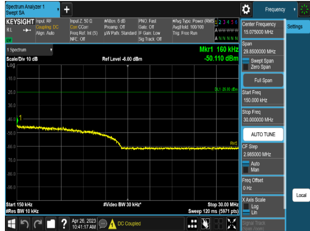
Plot 8-538. Conducted Spurious Emission Plot 150 kHz to 30 MHz (MSR 2C_DSS B(n)5_1C_10M+NR n5_1C_5M_2T_QPSK - Low Channel, Port 0)
