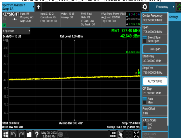
Plot 8-581. Conducted Spurious Emission Plot 30 MHz to 735 MHz (LTE B13_1C_10M_2T_64QAM - Middle Channel, Port 0)
