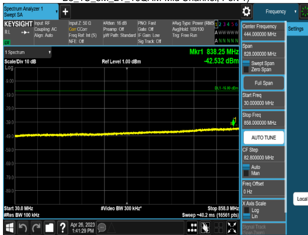
Plot 8-563. Conducted Spurious Emission Plot 30 MHz to 858 MHz (MSR 3C_DSS B(n)5_1C_10M+NR n5_1C_10M+LTE B5_1C_5M_2T_16QAM-Mid Channel, Port 1)
