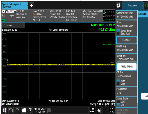
Plot 8-523. Conducted Spurious Emission Plot 895 MHz to 1 GHz (MSR 2C_NR n5_1C_5M+LTE B5_1C_5M_2T_16QAM-Middle Channel, Port 0)
