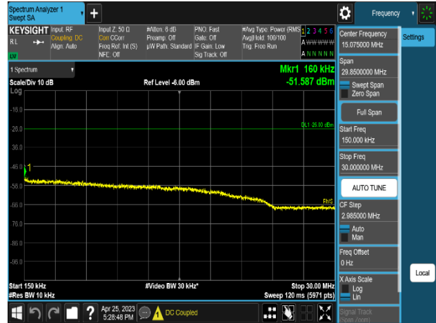
Plot 8-544. Conducted Spurious Emission Plot 150 kHz to 30 MHz (MSR 2C_DSS B(n)5_1C_10M+NR n5_1C_15M_2T_16QAM-Mid Channel, Port 0)
