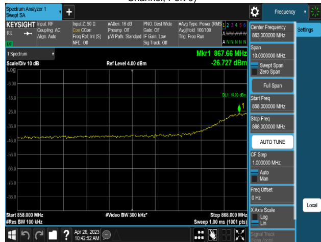
Plot 8-540. Conducted Spurious Emission Plot 858 MHz to 868 MHz (MSR 2C_DSS B(n)5_1C_10M+NR n5_1C_5M_2T_QPSK - Low Channel, Port 0)
