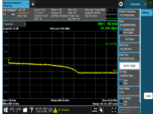
Plot 8-556. Conducted Spurious Emission Plot 150 kHz to 30 MHz (MSR 3C_DSS B(n)5_1C_10M+NR n5_1C_5M+LTE B5_1C_5M_2T_16QAM-Middle Channel, Port 0)
