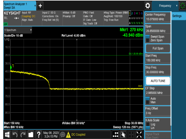
Plot 8-580. Conducted Spurious Emission Plot 150 kHz to 30 MHz (LTE B13_1C_10M_2T_64QAM - Middle Channel, Port 0)
