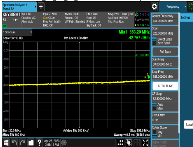
Plot 8-557. Conducted Spurious Emission Plot 30 MHz to 858 MHz (MSR 3C_DSS B(n)5_1C_10M+NR n5_1C_5M+LTE B5_1C_5M_2T_16QAM-Middle Channel, Port 0)
