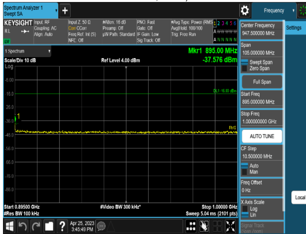
Plot 8-529. Conducted Spurious Emission Plot 895 MHz to 1 GHz (MSR 3C_NR n5_2C_10M+10M+LTE B5_1C_5M_2T_QPSK-Mid Channel, Port 0)
