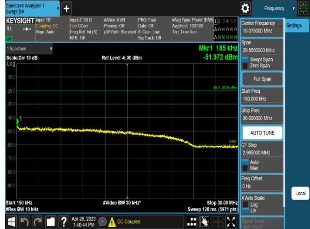
Plot 8-562. Conducted Spurious Emission Plot 150 kHz to 30 MHz (MSR 3C_DSS B(n)5_1C_10M+NR n5_1C_10M+LTE B5_1C_5M_2T_16QAM-Mid Channel, Port 1)
