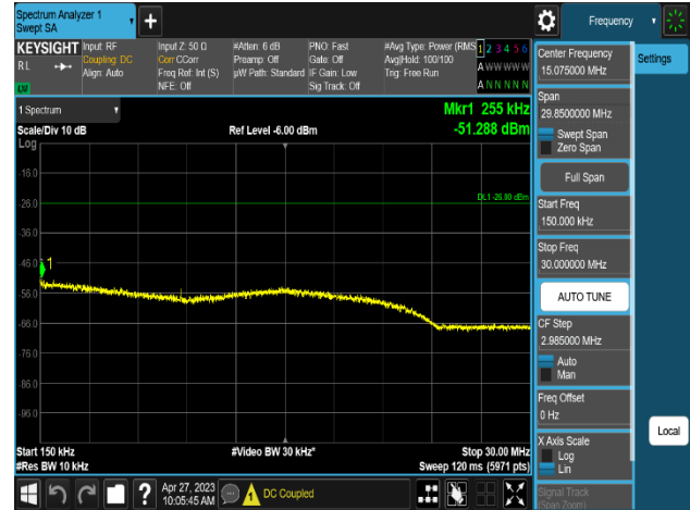
Plot 8-568. Conducted Spurious Emission Plot 150 kHz to 30 kHz (MSR 3NC_DSS B(n)5_1C_10M+NR n5_1C_5M+LTE B5_1C_5M_2T_QPSK-Mid Channel, Port 0)
