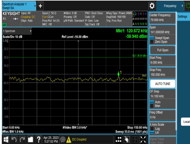
Plot 8-543. Conducted Spurious Emission Plot 9 kHz to 150 kHz (MSR 2C_DSS B(n)5_1C_10M+NR n5_1C_15M_2T_16QAM-Mid Channel, Port 0)
