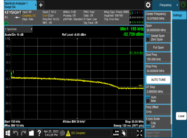
Plot 8-526. Conducted Spurious Emission Plot 150 kHz to 30 MHz (MSR 3C_NR n5_2C_10M+10M+LTE B5_1C_5M_2T_QPSK-Mid Channel, Port 0)
