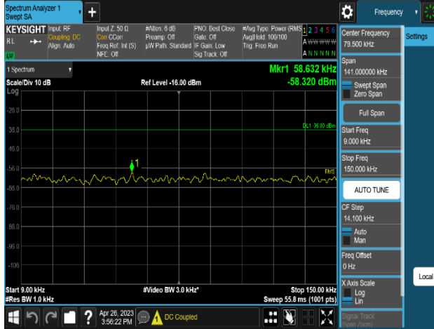
Plot 8-555. Conducted Spurious Emission Plot 9 kHz to 150 kHz (MSR 3C_DSS B(n)5_1C_10M+NR n5_1C_5M+LTE B5_1C_5M_2T_16QAM-Middle Channel, Port 0)
