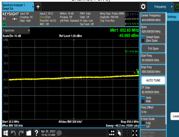
Plot 8-539. Conducted Spurious Emission Plot 30 MHz to 858 MHz (MSR 2C_DSS B(n)5_1C_10M+NR n5_1C_5M_2T_QPSK - Low Channel, Port 0)
