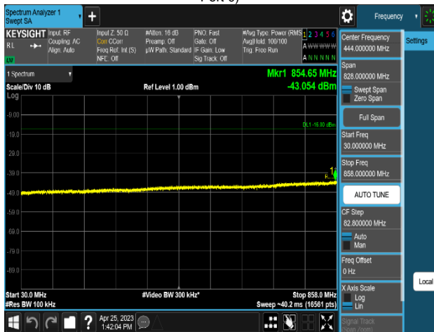
Plot 8-521. Conducted Spurious Emission Plot 30 MHz to 858 MHz (MSR 2C_NR n5_1C_5M+LTE B5_1C_5M_2T_16QAM-Middle Channel, Port 0)
