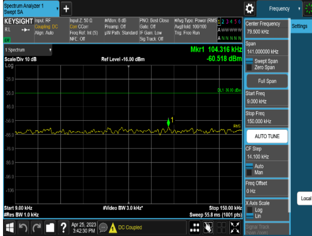
Plot 8-525. Conducted Spurious Emission Plot 9 kHz to 150 kHz (MSR 3C_NR n5_2C_10M+10M+LTE B5_1C_5M_2T_QPSK-Mid Channel, Port 0)
