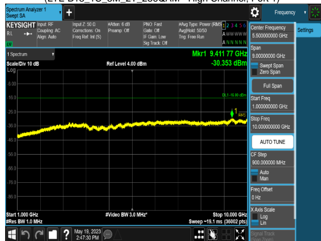
Plot 8-578. Conducted Spurious Emission Plot 1 GHz to 10 GHz (LTE B13_1C_5M_2T_256QAM - High Channel, Port 1)
