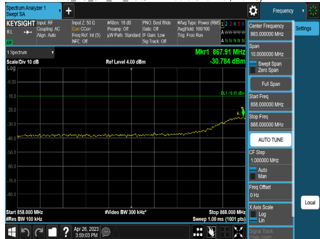
Plot 8-558. Conducted Spurious Emission Plot 858 MHz to 868 MHz (MSR 3C_DSS B(n)5_1C_10M+NR n5_1C_5M+LTE B5_1C_5M_2T_16QAM-Middle Channel, Port 0)
