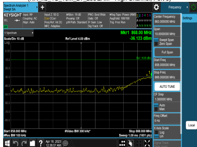
Plot 8-474. Conducted Spurious Emission Plot 858 MHz to 868 MHz (NR_n5_1C_10M_2T_256QAM - High Channel, Port 0)
