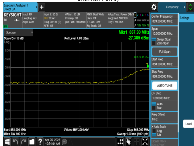
Plot 8-516. Conducted Spurious Emission Plot 858 MHz to 868 MHz (MSR 2NC_DSS B(n)5_1C_10M+LTE B5_1C_5M_2T_QPSK-Mid Channel, Port 0)
