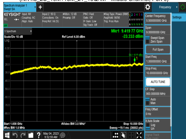
Plot 8-494. Conducted Spurious Emission Plot 1 GHz to 10 GHz (NR n5_2C_10M+15M_2T_16QAM - Middle Channel, Port 0)
