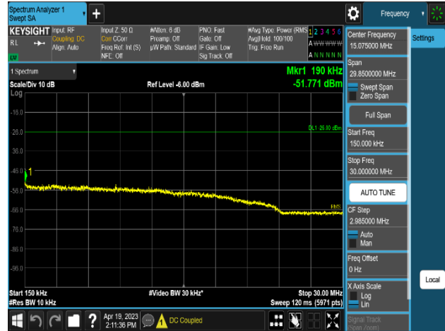
Plot 8-490. Conducted Spurious Emission Plot 150 kHz to 30 MHz (NR n5_2C_10M+15M_2T_16QAM - Middle Channel, Port 0)
