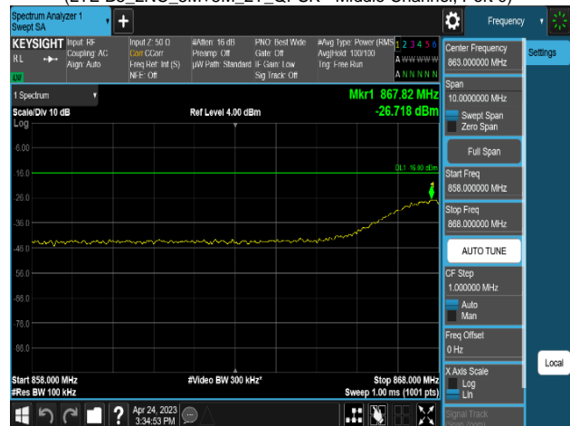
Plot 8-450. Conducted Spurious Emission Plot 858 MHz to 868 MHz (LTE B5_2NC_5M+5M_2T_QPSK - Middle Channel, Port 0)
