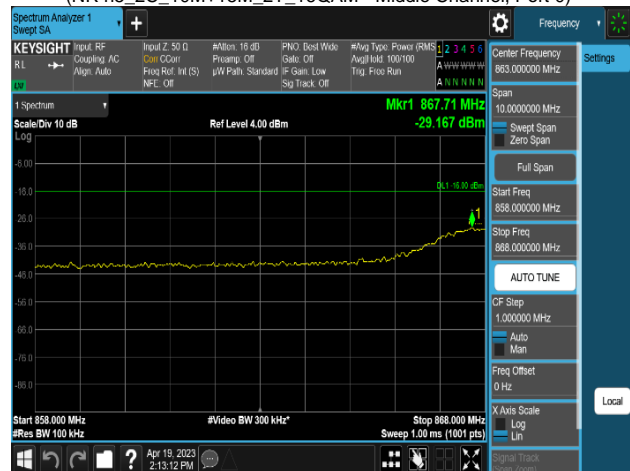
Plot 8-492. Conducted Spurious Emission Plot 858 MHz to 868 MHz (NR n5_2C_10M+15M_2T_16QAM - Middle Channel, Port 0)
