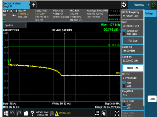
Plot 8-502. Conducted Spurious Emission Plot 150 kHz to 30 MHz (MSR 2C_DSS B(n)5_1C_10M+LTE B5_1C_5M_2T_QPSK - High Channel, Port 0)
