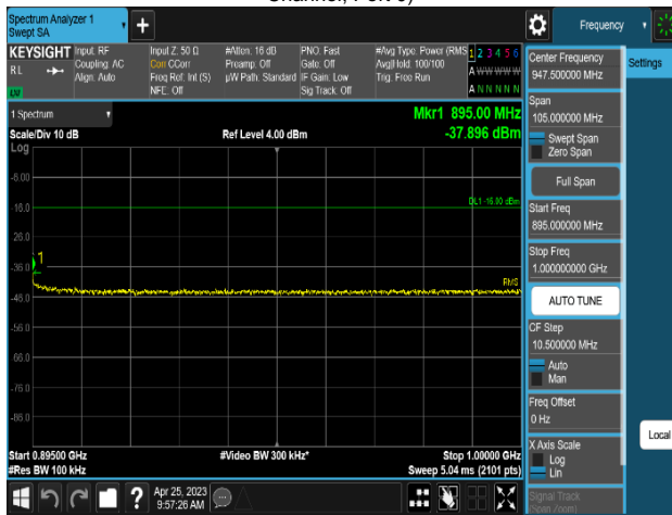
Plot 8-505. Conducted Spurious Emission Plot 895 MHz to 1 GHz (MSR 2C_DSS B(n)5_1C_10M+LTE B5_1C_5M_2T_QPSK - High Channel, Port 0)
