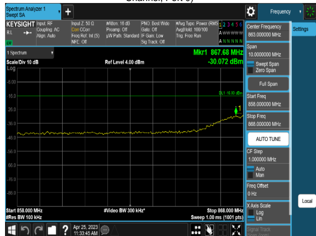
Plot 8-510. Conducted Spurious Emission Plot 858 MHz to 868 MHz (MSR 3C_DSS B(n)5_2C_10M+10M+LTE B5_1C_5M_2T_QPSK-Mid Channel, Port 0)
