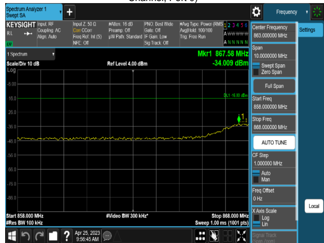
Plot 8-504. Conducted Spurious Emission Plot 858 MHz to 868 MHz (MSR 2C_DSS B(n)5_1C_10M+LTE B5_1C_5M_2T_QPSK - High Channel, Port 0)
