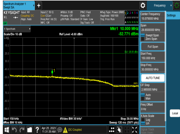
Plot 8-508. Conducted Spurious Emission Plot 150 kHz to 30 MHz (MSR 3C_DSS B(n)5_2C_10M+10M+LTE B5_1C_5M_2T_QPSK-Mid Channel, Port 0)
