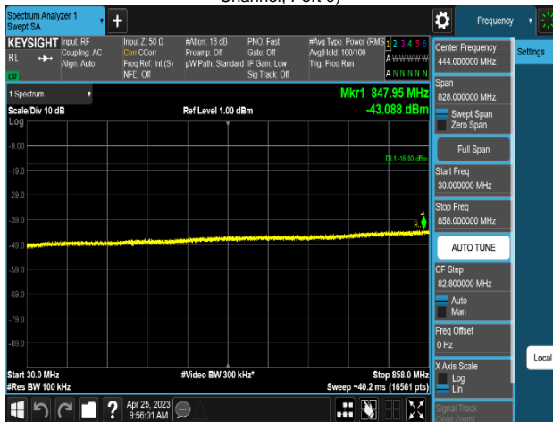
Plot 8-503. Conducted Spurious Emission Plot 30 MHz to 858 MHz (MSR 2C_DSS B(n)5_1C_10M+LTE B5_1C_5M_2T_QPSK - High Channel, Port 0)
