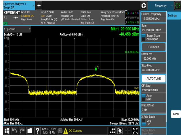
Plot 8-496. Conducted Spurious Emission Plot 150 kHz to 30 MHz (NR n5_2NC_5M+5M_2T_QPSK - Middle Channel, Port 0)
