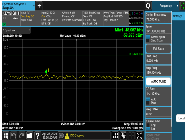
Plot 8-513. Conducted Spurious Emission Plot 9 kHz to 150 kHz (MSR 2NC_DSS B(n)5_1C_10M+LTE B5_1C_5M_2T_QPSK-Mid Channel, Port 0)
