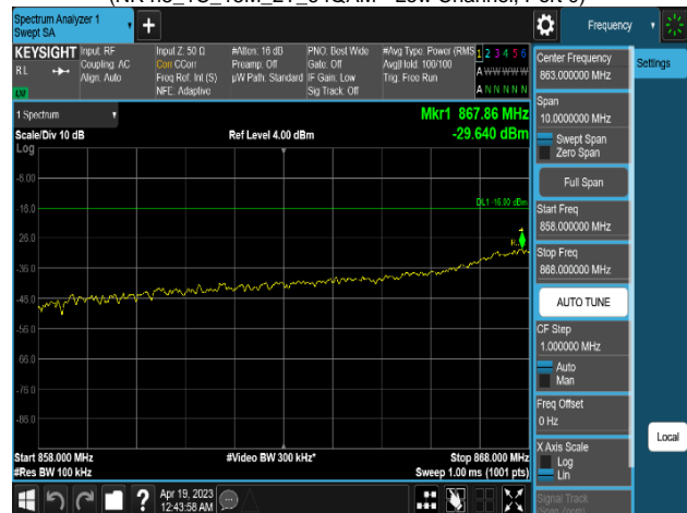
Plot 8-480. Conducted Spurious Emission Plot 858 MHz to 868 MHz (NR n5_1C_15M_2T_64QAM - Low Channel, Port 0)
