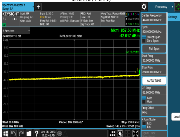
Plot 8-509. Conducted Spurious Emission Plot 30 MHz to 858 MHz (MSR 3C_DSS B(n)5_2C_10M+10M+LTE B5_1C_5M_2T_QPSK-Mid Channel, Port 0)
