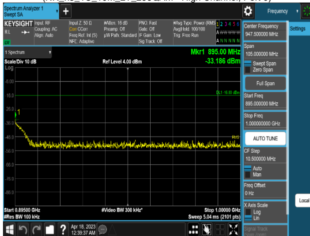
Plot 8-475. Conducted Spurious Emission Plot 895 MHz to 1 GHz (NR_n5_1C_10M_2T_256QAM - High Channel, Port 0)
