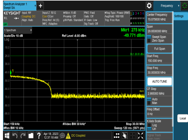
Plot 8-472. Conducted Spurious Emission Plot 150 kHz to 30 MHz (NR_n5_1C_10M_2T_256QAM - High Channel, Port 0)
