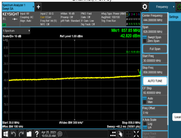
Plot 8-515. Conducted Spurious Emission Plot 30 MHz to 858 MHz (MSR 2NC_DSS B(n)5_1C_10M+LTE B5_1C_5M_2T_QPSK-Mid Channel, Port 0)
