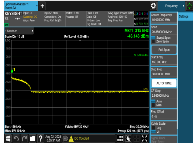
Plot 8-466. Conducted Spurious Emission Plot 150 kHz to 30 MHz (NR n5_1C_5M_2T_64QAM - Low Channel, Port 1)
