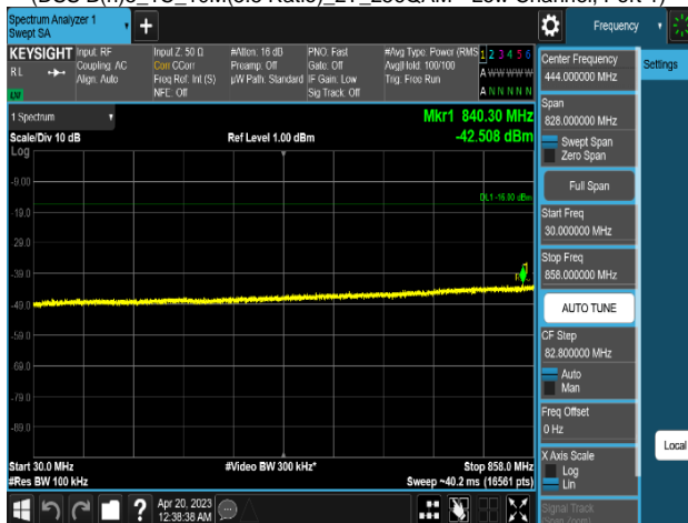
Plot 8-455. Conducted Spurious Emission Plot 30 MHz to 858 MHz
