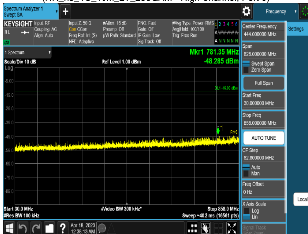
Plot 8-473. Conducted Spurious Emission Plot 30 MHz to 858 MHz (NR_n5_1C_10M_2T_256QAM - High Channel, Port 0)
