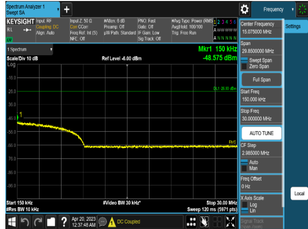
Plot 8-454. Conducted Spurious Emission Plot 150 kHz to 30 MHz
