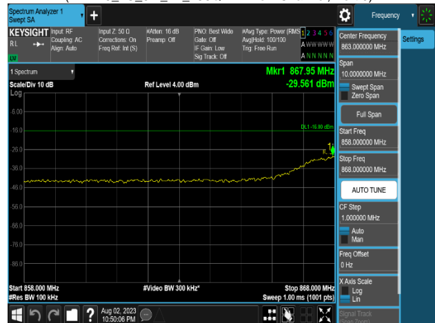
Plot 8-426. Conducted Spurious Emission Plot 858 MHz to 868 MHz (LTE B5_1C_5M_2T_256QAM - Low Channel, Port 0)
