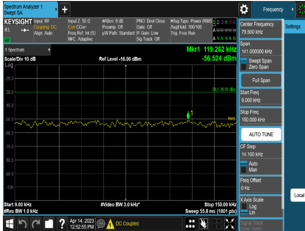
Plot 8-429. Conducted Spurious Emission Plot 9 kHz to 150 kHz (LTE B5_1C_10M_2T_16QAM - High Channel, Port 0)
