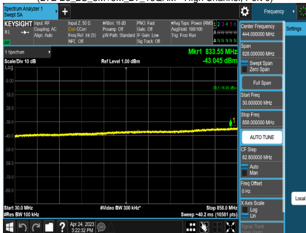
Plot 8-437. Conducted Spurious Emission Plot 30 MHz to 858 MHz (LTE B5_2C_5M+5M_2T_16QAM - High Channel, Port 0)
