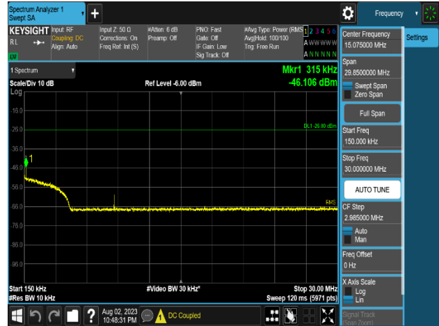
Plot 8-424. Conducted Spurious Emission Plot 150 kHz to 30 MHz (LTE B5_1C_5M_2T_256QAM - Low Channel, Port 0)
