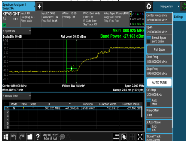
Plot 8-387. Band Edge Emission Summary Data Plot (MSR 2NC_DSS B(n)5_1C_10M+LTE B5_1C_5M_QPSK - Low Channel_4T, Port 0)
