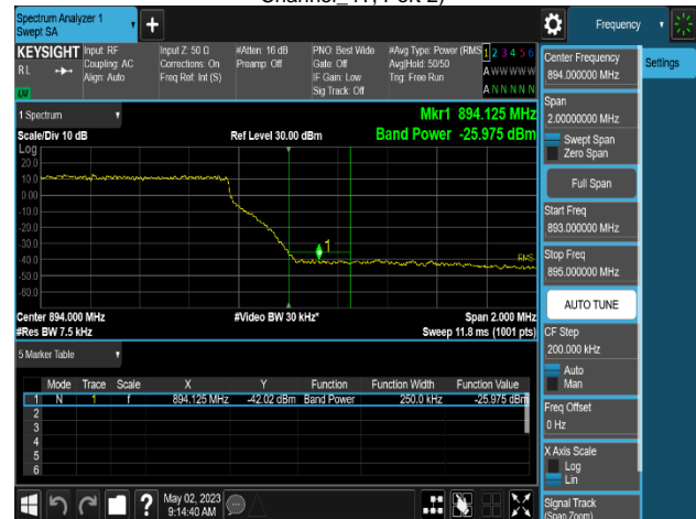
Plot 8-390. Band Edge Emission Summary Data Plot (MSR 3C_DSS B(n)5_2C_10M+10M+LTE B5_1C_5M_QPSK - High Channel_4T, Port 3)
