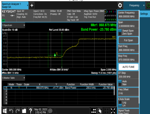
Plot 8-395. Band Edge Emission Summary Data Plot (MSR 3C_NR n5_2C_10M+10M+LTE B5_1C_5M_QPSK - Low Channel_4T, Port 2)
