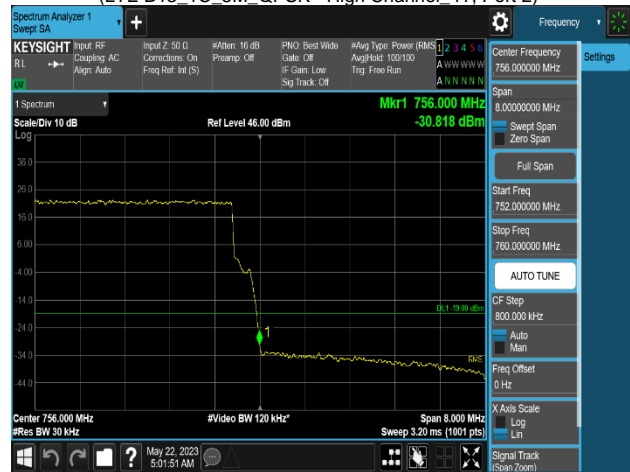
Plot 8-412. Band Edge Emission Summary Data Plot (LTE B13_1C_10M_256QAM - High Channel_4T, Port 1)
