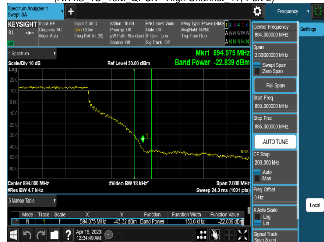
Plot 8-378. Band Edge Emission Summary Data Plot (NR n5_1C_15M_16QAM - High Channel_4T, Port 0)
