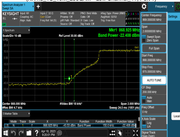
Plot 8-377. Band Edge Emission Summary Data Plot (NR n5_1C_15M_QPSK - Low Channel_4T, Port 2)
