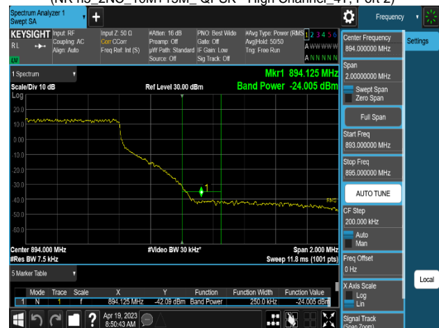
Plot 8-384. Band Edge Emission Summary Data Plot (NR n5_2C_10M+15M_16QAM - High Channel_4T, Port 2)
