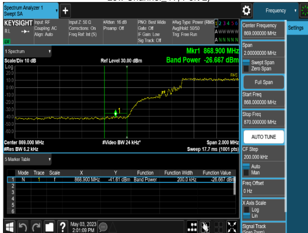
Plot 8-405. Band Edge Emission Summary Data Plot (MSR 3NC_DSS B(n)5_1C_10M+NR n5_1C_5M+LTE B5_1C_5M_QPSK - Low Channel_4T, Port 1)
