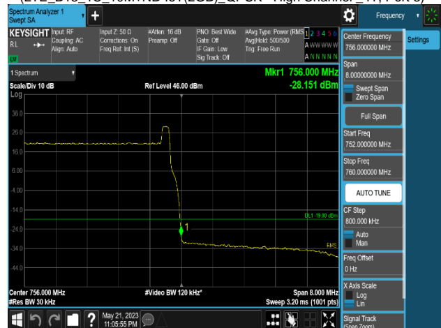
Plot 8-420. Band Edge Emission Summary Data Plot (Multi-Band_LTE B13_1C_10M+B5_1C_10M_QPSK - High Channel _4T, Port 3)
