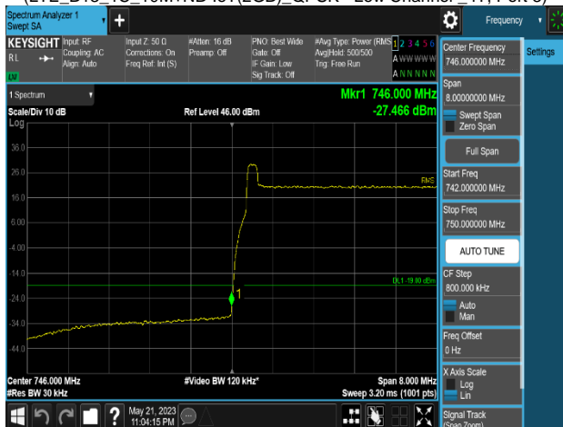
Plot 8-419. Band Edge Emission Summary Data Plot (Multi-Band_LTE B13_1C_10M+B5_1C_10M_QPSK - Low Channel _4T, Port 3)
