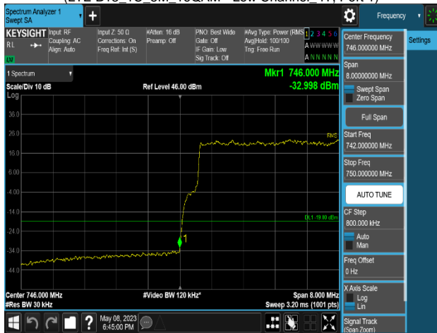
Plot 8-411. Band Edge Emission Summary Data Plot (LTE B13_1C_10M_16QAM - Low Channel_4T, Port 2)
