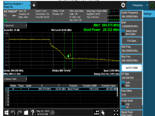
Plot 8-400. Band Edge Emission Summary Data Plot (MSR 2NC_DSS B(n)5_1C_10M+NR n5_1C_5M_QPSK - High Channel_4T, Port 2)
