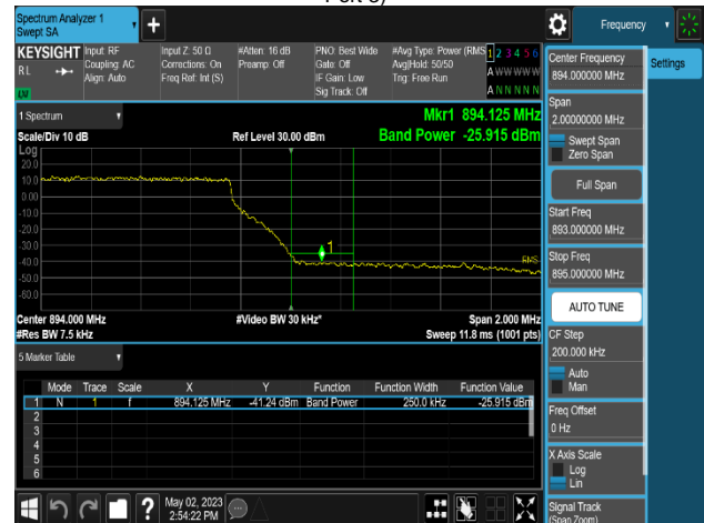
Plot 8-396. Band Edge Emission Summary Data Plot (MSR 3C_NR n5_2C_10M+10M+LTE B5_1C_5M_QPSK - High Channel_4T, Port 2)
