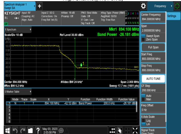
Plot 8-406. Band Edge Emission Summary Data Plot (MSR 3NC_DSS B(n)5_1C_10M+NR n5_1C_5M+LTE B5_1C_5M_QPSK - High Channel_4T, Port 2)
