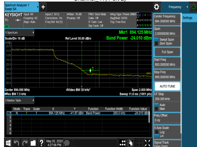
Plot 8-402. Band Edge Emission Summary Data Plot (MSR 2C_DSS B(n)5_1C_10M+NR n5_1C_15M_16QAM - High Channel_4T, Port 1)
