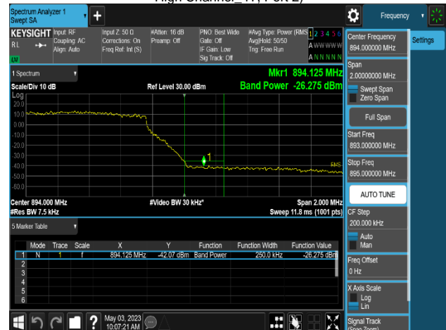
Plot 8-408. Band Edge Emission Summary Data Plot (MSR 3C_DSS B(n)5_2C_10M+10M+LTE B5_1C_5M_16QAM - High Channel_4T, Port 2)
