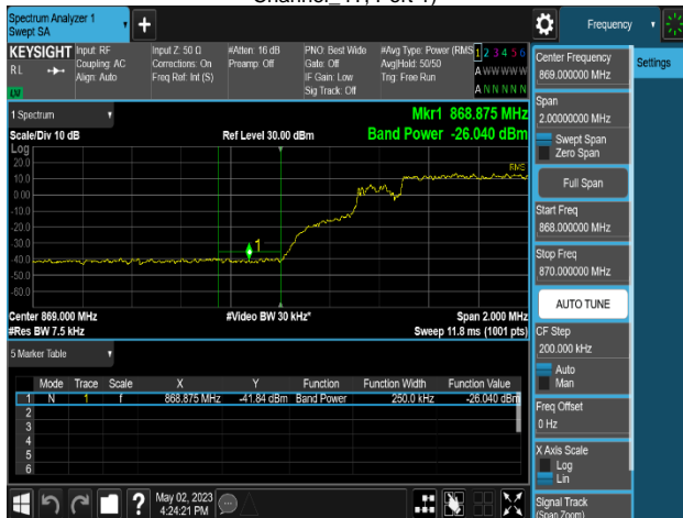
Plot 8-401. Band Edge Emission Summary Data Plot (MSR 2C_DSS B(n)5_1C_10M+NR n5_1C_15M_16QAM - Low Channel_4T, Port 1)
