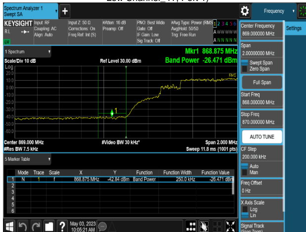
Plot 8-407. Band Edge Emission Summary Data Plot (MSR 3C_DSS B(n)5_1C_10M+NR n5_1C_10M+LTE B5_1C_5M_16QAM - Low Channel_4T, Port 2)
