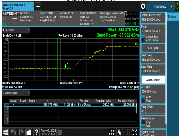
Plot 8-389. Band Edge Emission Summary Data Plot (MSR 3C_DSS B(n)5_2C_10M+10M+LTE B5_1C_5M_16QAM - Low Channel_4T, Port 1)
