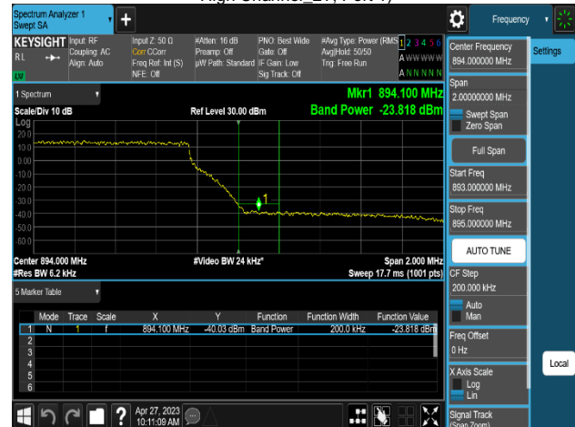
Plot 8-340. Band Edge Emission Summary Data Plot (MSR 3NC_DSS B(n)5_1C_10M+NR n5_1C_5M+LTE B5_1C_5M_QPSK - High Channel_2T, Port 1)
