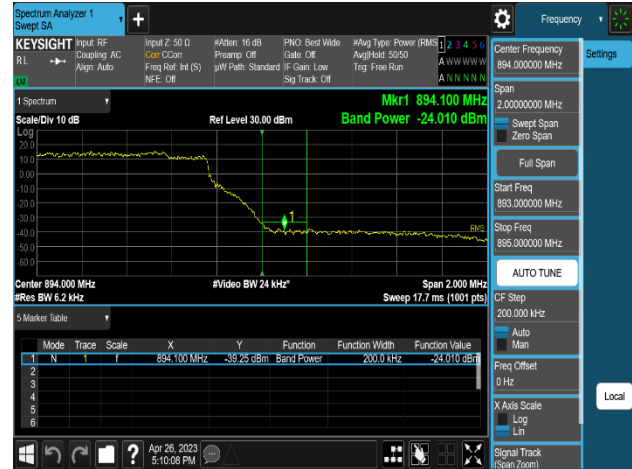
Plot 8-338. Band Edge Emission Summary Data Plot (MSR 3C_DSS B(n)5_1C_10M+NR n5_1C_5M+LTE B5_1C_5M_16QAM - High Channel_2T, Port 1)
