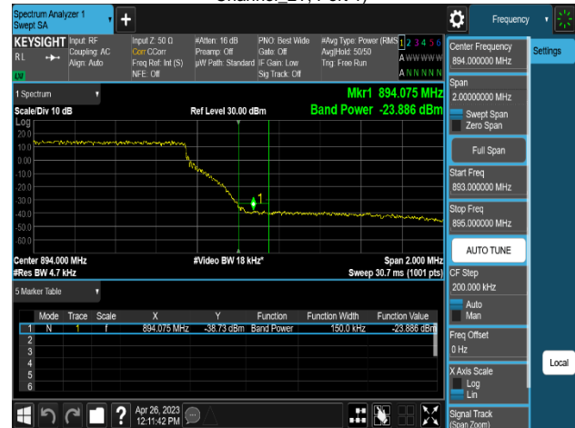
Plot 8-334. Band Edge Emission Summary Data Plot (MSR 2NC_DSS B(n)5_1C_10M+NR n5_1C_5M_QPSK - High Channel_2T, Port 1)
