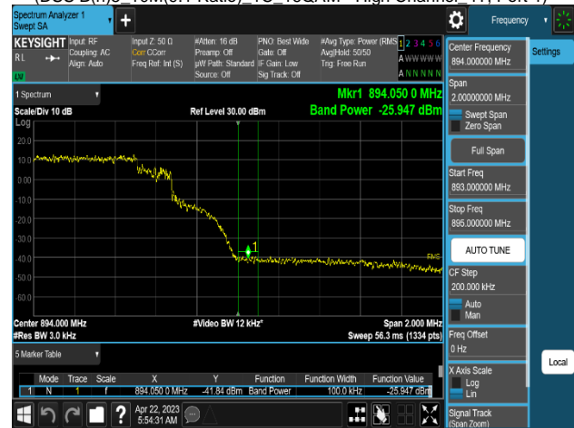
Plot 8-370. Band Edge Emission Summary Data Plot (DSS B(n)5_10M(8:2 Ratio)_1C_256QAM - High Channel 4T, Port 1)
