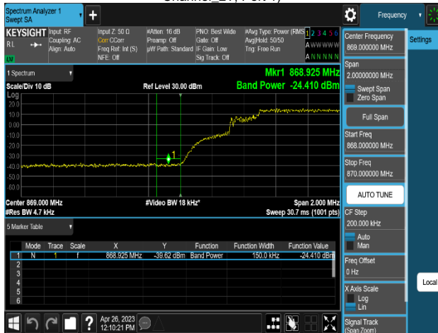
Plot 8-333. Band Edge Emission Summary Data Plot (MSR 2NC_DSS B(n)5_1C_10M+NR n5_1C_5M_QPSK - Low Channel_2T, Port 1)
