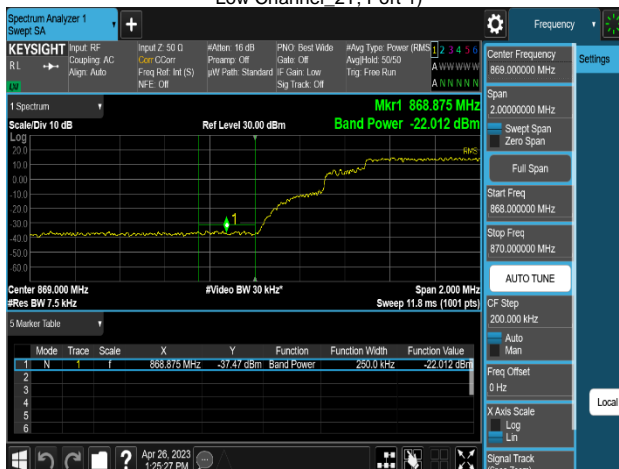
Plot 8-341. Band Edge Emission Summary Data Plot (MSR 3C_DSS B(n)5_1C_10M+NR n5_1C_10M+LTE B5_1C_5M_QPSK - Low Channel_2T, Port 1)
