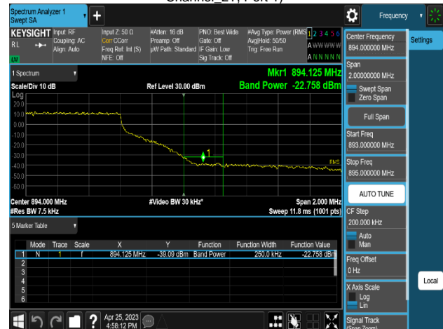
Plot 8-336. Band Edge Emission Summary Data Plot (MSR 2C_DSS B(n)5_1C_10M+NR n5_1C_15M_QPSK - High Channel_2T, Port 1)
