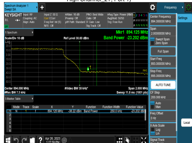
Plot 8-342. Band Edge Emission Summary Data Plot (MSR 3C_DSS B(n)5_2C_10M+10M+LTE B5_1C_5M_QPSK - High Channel_2T, Port 1)
