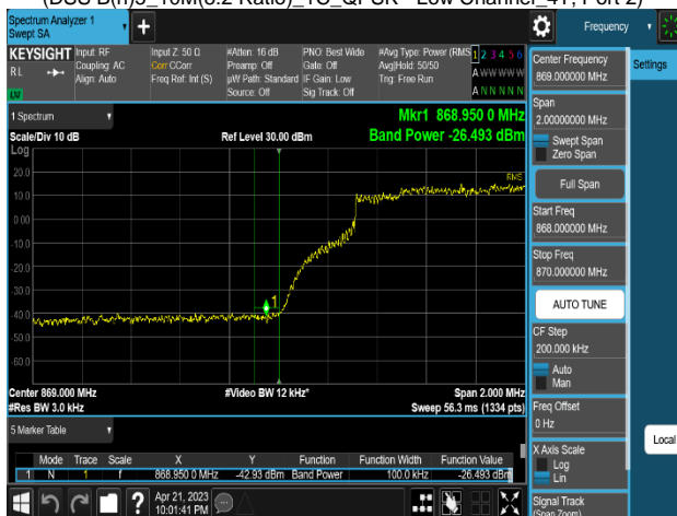
Plot 8-371. Band Edge Emission Summary Data Plot (DSS B(n)5_10M(4:6 Ratio)_1C_16QAM - Low Channel 4T, Port 2)
