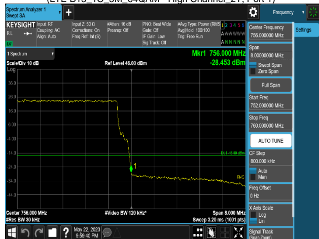
Plot 8-346. Band Edge Emission Summary Data Plot (LTE B13_1C_10M_256QAM - High Channel_2T, Port 1)
