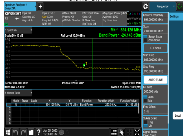
Plot 8-324. Band Edge Emission Summary Data Plot (MSR 3C_DSS B(n)5_2C_10M+10M+LTE B5_1C_5M_16QAM - High Channel_2T, Port 1)
