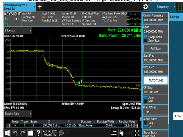
Plot 8-360. Band Edge Emission Summary Data Plot (LTE B5_1C_10M_256QAM - High Channel_4T, Port 2)
