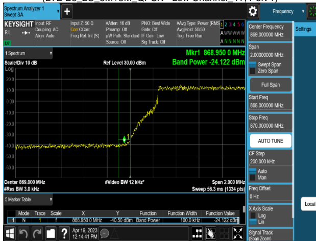
Plot 8-363. Band Edge Emission Summary Data Plot (LTE B5_2NC_5M+5M_QPSK - Low Channel_2T, Port 0)
