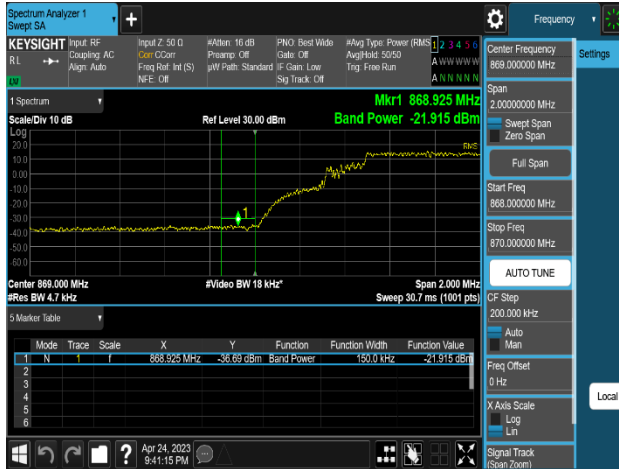
Plot 8-319. Band Edge Emission Summary Data Plot (MSR 2C_DSS B(n)5_1C_10M+LTE B5_1C_5M_QPSK - Low Channel_2T, Port 0)
