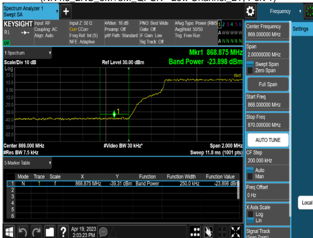
Plot 8-317. Band Edge Emission Summary Data Plot (NR n5_2C_10M+15M_QPSK - Low Channel_2T, Port 1)
