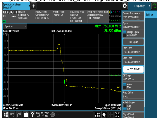
Plot 8-352. Band Edge Emission Summary Data Plot (B13_10M(LTE)+NB-IoT(2GB)_1C_QPSK - High Channel _2T, Port 0)
