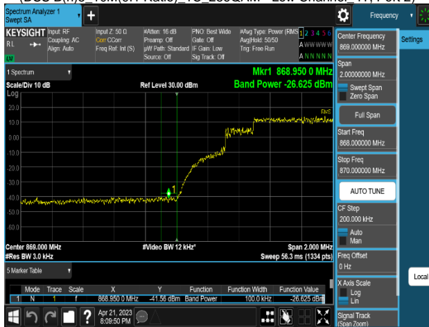
Plot 8-369. Band Edge Emission Summary Data Plot (DSS B(n)5_10M(8:2 Ratio)_1C_QPSK - Low Channel 4T, Port 2)
