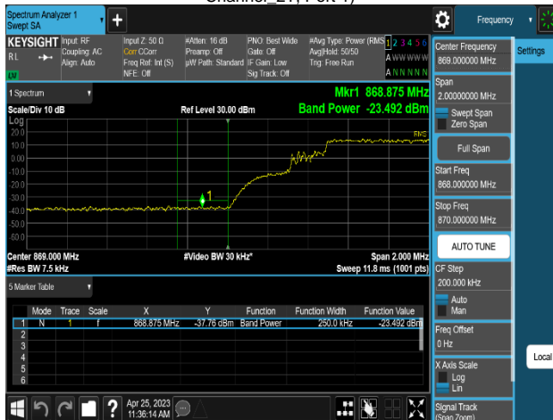
Plot 8-323. Band Edge Emission Summary Data Plot (MSR 3C_DSS B(n)5_2C_10M+10M+LTE B5_1C_5M_QPSK - Low Channel_2T, Port 1)
