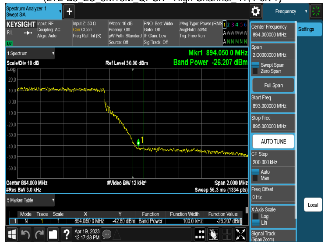
Plot 8-364. Band Edge Emission Summary Data Plot (LTE B5_2NC_5M+5M_QPSK - High Channel_4T, Port 3)
