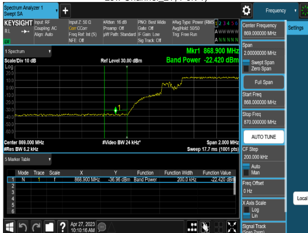
Plot 8-339. Band Edge Emission Summary Data Plot (MSR 3NC_DSS B(n)5_1C_10M+NR n5_1C_5M+LTE B5_1C_5M_QPSK - Low Channel_2T, Port 1)
