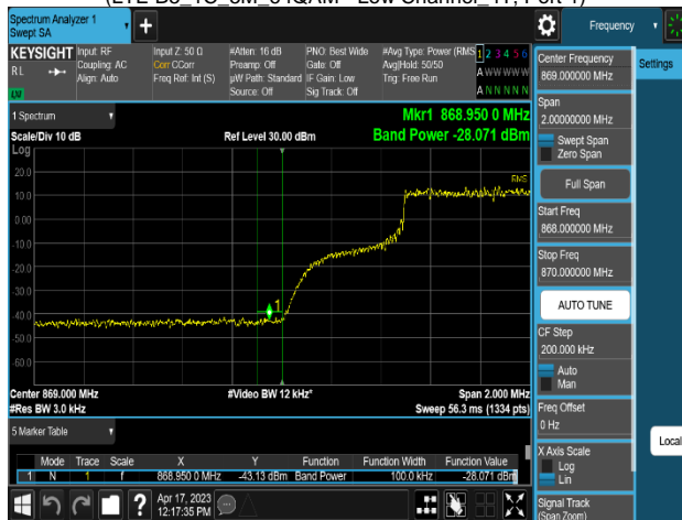
Plot 8-359. Band Edge Emission Summary Data Plot (LTE B5_1C_10M_16QAM - Low Channel_4T, Port 1)
