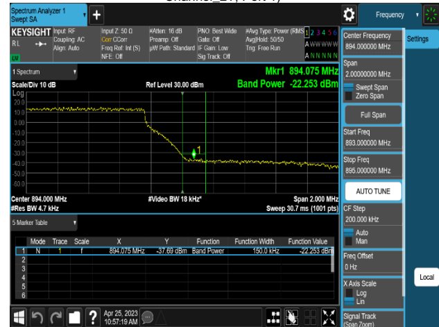
Plot 8-322. Band Edge Emission Summary Data Plot (MSR 2NC_DSS B(n)5_1C_10M+LTE B5_1C_5M_QPSK - High Channel_2T, Port 1)
