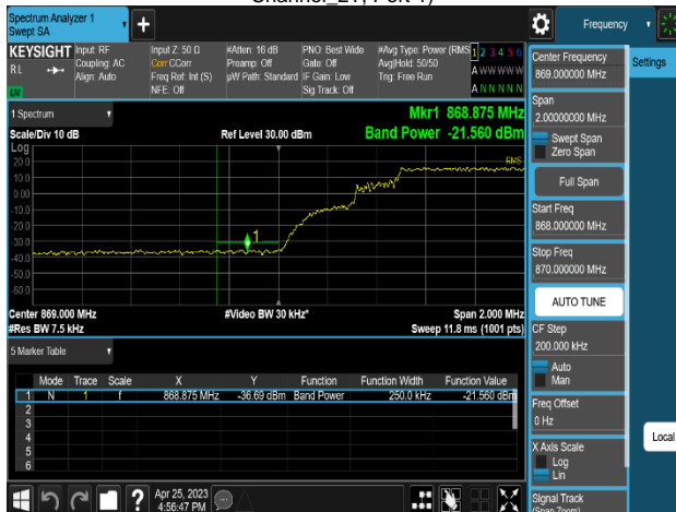
Plot 8-335. Band Edge Emission Summary Data Plot (MSR 2C_DSS B(n)5_1C_10M+NR n5_1C_15M_QPSK - Low Channel_2T, Port 1)
