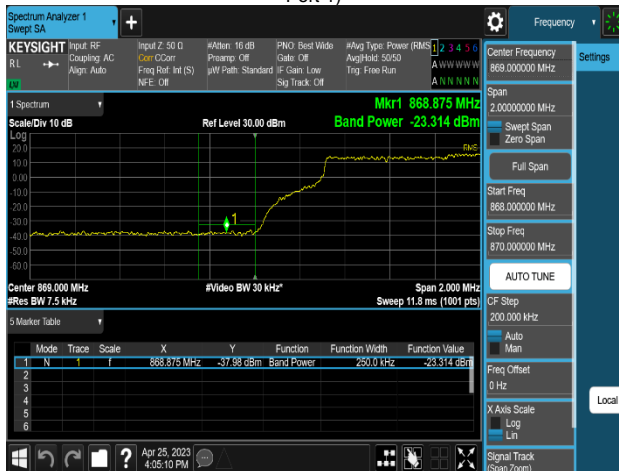
Plot 8-329. Band Edge Emission Summary Data Plot (MSR 3C_NR n5_2C_10M+10M+LTE B5_1C_5M_16QAM - Low Channel_2T, Port 1)
