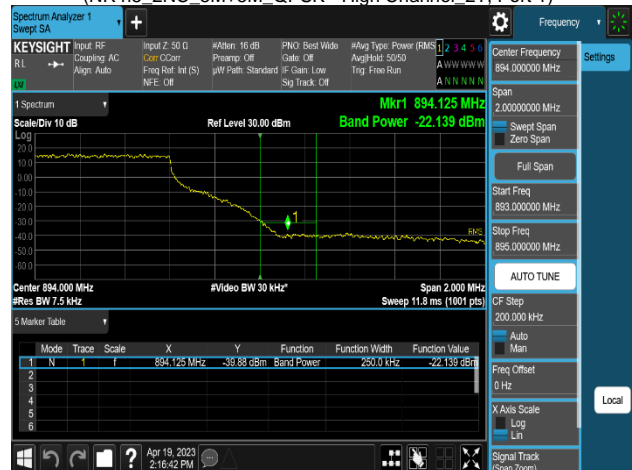
Plot 8-318. Band Edge Emission Summary Data Plot (NR n5_2C_10M+15M_16QAM - High Channel_2T, Port 1)
