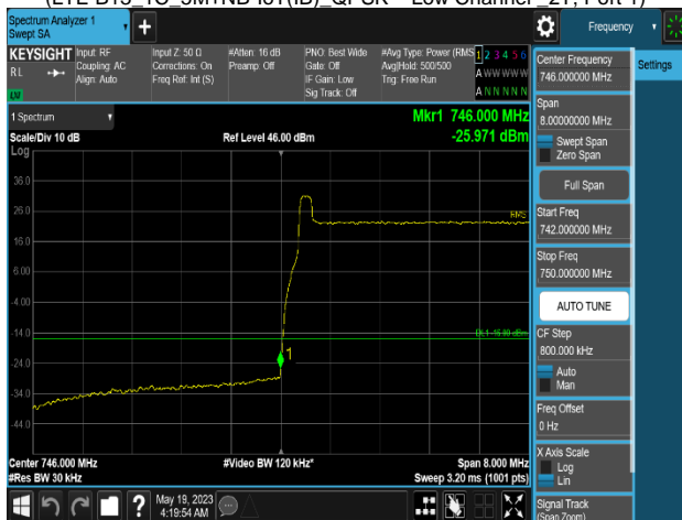
Plot 8-351. Band Edge Emission Summary Data Plot (B13_10M(LTE)+NB-IoT(2GB)_1C_QPSK - Low Channel _2T, Port 0)
