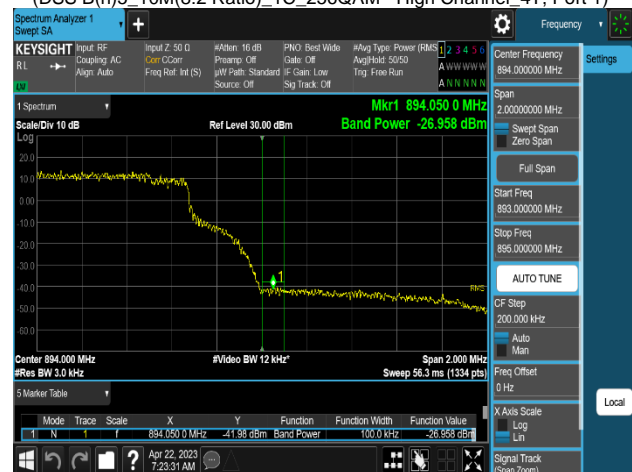
Plot 8-372. Band Edge Emission Summary Data Plot (DSS B(n)5_10M(4:6 Ratio)_1C_256QAM - High Channel 4T, Port 0)
