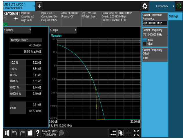
Plot 8-272. Peak To Average Power Ratio Plot (LTE B13_1C_10M_256QAM - Mid Channel_4T, Port 0)
