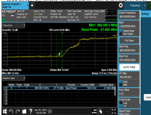
Plot 8-297. Band Edge Emission Summary Data Plot (DSS B(n)5_1C_10M(4:6 Ratio)_16QAM - Low Channel 2T, Port 1)
