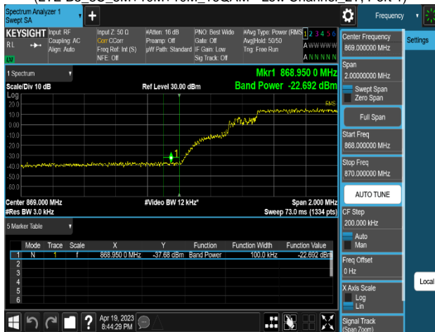
Plot 8-287. Band Edge Emission Summary Data Plot (DSS B(n)5_1C_10M(9:1 Ratio)_256QAM - Low Channel_2T, Port 1)
