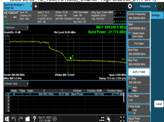
Plot 8-300. Band Edge Emission Summary Data Plot (DSS B(n)5_1C_10M(3:7 Ratio)_64QAM - High Channel 2T, Port 1)
