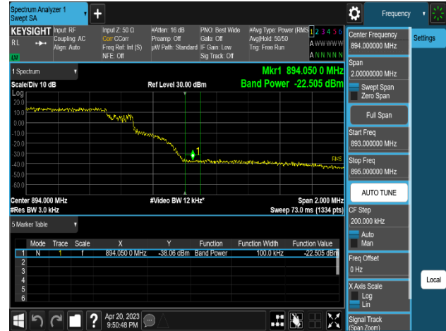
Plot 8-290. Band Edge Emission Summary Data Plot (DSS B(n)5_1C_10M(8:2 Ratio)_256QAM - High Channel 2T, Port 1)
