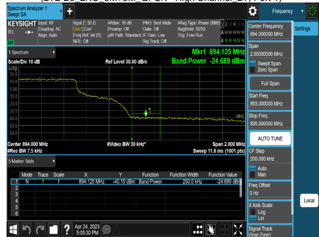
Plot 8-286. Band Edge Emission Summary Data Plot (LTE B5_3C_5M+10M+10M_16QAM - High Channel_2T, Port 1)
