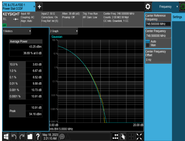
Plot 8-275. Peak To Average Power Ratio Plot (LTE B13_1C_5M+NB-IoT(IB)_QPSK - Low Channel_4T, Port 1)
