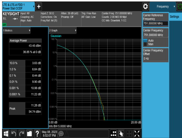
Plot 8-269. Peak To Average Power Ratio Plot (LTE B13_1C_5M_QPSK - Mid Channel_4T, Port 0)
