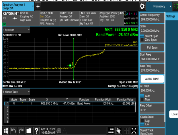
Plot 8-279. Band Edge Emission Summary Data Plot (LTE B5_1C_10M_QPSK - Low Channel_2T, Port 1)
