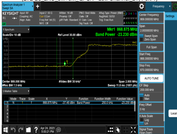
Plot 8-285. Band Edge Emission Summary Data Plot (LTE B5_3C_5M+10M+10M_16QAM - Low Channel_2T, Port 1)
