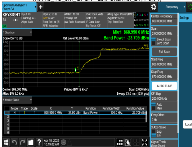
Plot 8-309. Band Edge Emission Summary Data Plot (NR n5_1C_10M_16QAM - Low Channel_2T, Port 0)
