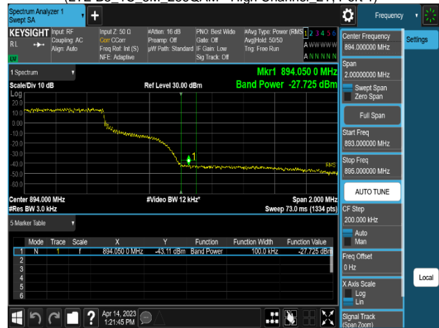
Plot 8-280. Band Edge Emission Summary Data Plot (LTE B5_1C_10M_256QAM - High Channel_2T, Port 1)
