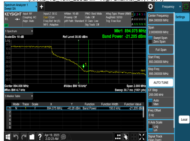
Plot 8-312. Band Edge Emission Summary Data Plot (NR n5_1C_15M_16QAM - High Channel_2T, Port 1)
