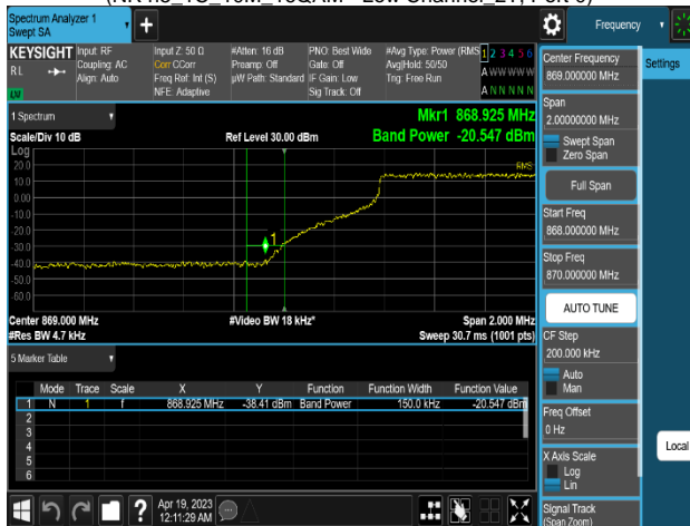
Plot 8-311. Band Edge Emission Summary Data Plot (NR n5_1C_15M_QPSK - Low Channel_2T, Port 1)
