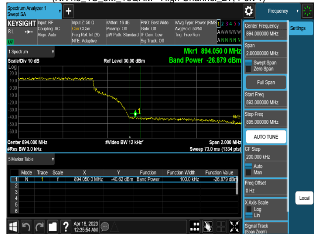
Plot 8-310. Band Edge Emission Summary Data Plot (NR n5_1C_10M_256QAM - High Channel_2T, Port 1)
