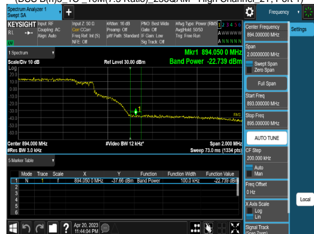
Plot 8-294. Band Edge Emission Summary Data Plot (DSS B(n)5_1C_10M(6:4 Ratio)_256QAM - High Channel 2T, Port 1)
