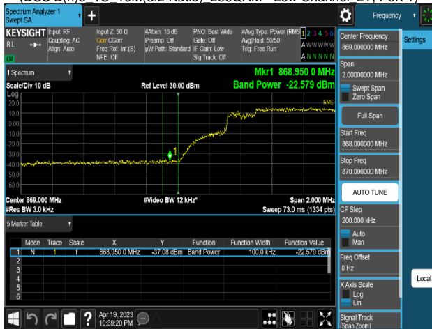
Plot 8-291. Band Edge Emission Summary Data Plot (DSS B(n)5_1C_10M(7:3 Ratio)_256QAM - Low Channel 2T, Port 1)
