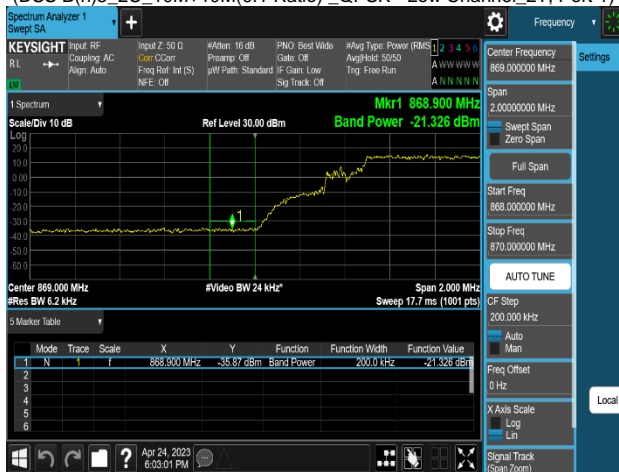
Plot 8-305. Band Edge Emission Summary Data Plot (DSS B(n)5_2NC_10M+10M(9:1 Ratio)_QPSK - Low Channel_2T, Port 1)
