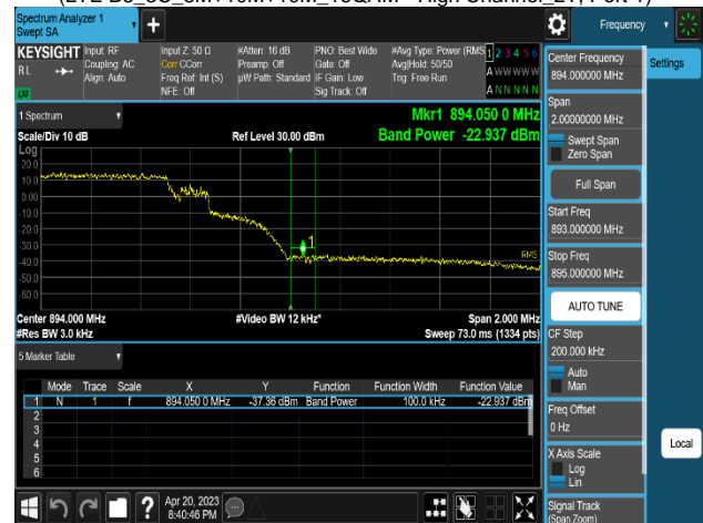
Plot 8-288. Band Edge Emission Summary Data Plot (DSS B(n)5_1C_10M(9:1 Ratio)_64QAM - High Channel_2T, Port 1)
