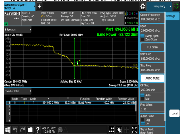
Plot 8-298. Band Edge Emission Summary Data Plot (DSS B(n)5_1C_10M(4:6 Ratio)_64QAM - High Channel 2T, Port 1)
