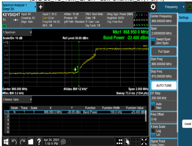
Plot 8-281. Band Edge Emission Summary Data Plot (LTE B5_2C_5M+5M_QPSK - Low Channel_2T, Port 1)
