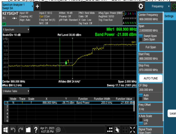
Plot 8-303. Band Edge Emission Summary Data Plot (DSS B(n)5_2C_10M+10M(9:1 Ratio)_QPSK - Low Channel_2T, Port 1)
