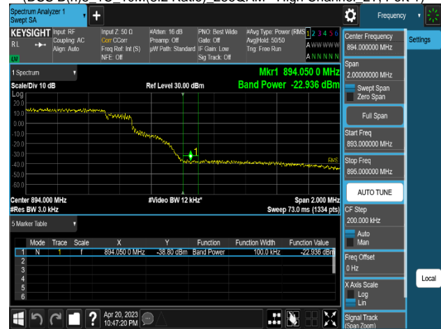
Plot 8-292. Band Edge Emission Summary Data Plot (DSS B(n)5_1C_10M(7:3 Ratio)_256QAM - High Channel 2T, Port 1)
