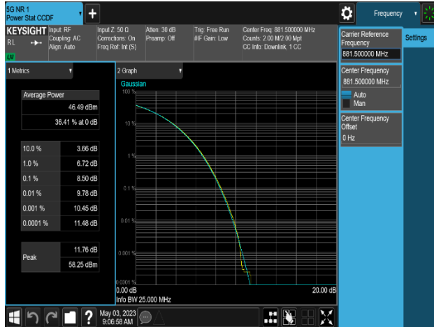
Plot 8-267. Peak To Average Power Ratio Plot (MSR 3C_DSS B(n)5_1C_10M+NR n5_1C_10M+LTE B5_1C_5M_QPSK - Mid Channel_4T, Port 0)
