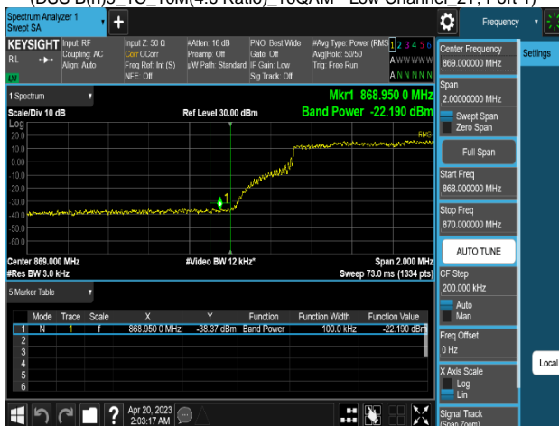
Plot 8-299. Band Edge Emission Summary Data Plot (DSS B(n)5_1C_10M(3:7 Ratio)_16QAM - Low Channel 2T, Port 1)
