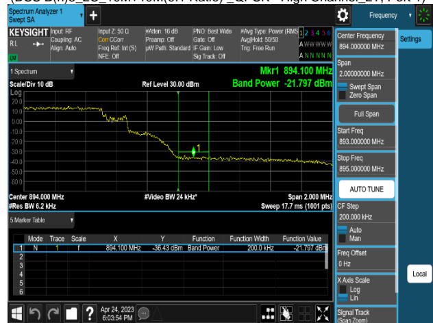
Plot 8-306. Band Edge Emission Summary Data Plot (DSS B(n)5_2NC_10M+10M(9:1 Ratio)_QPSK - High Channel_2T, Port 1)
