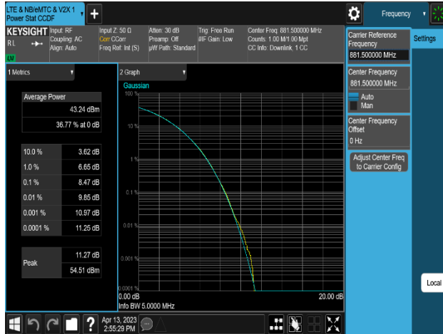
Plot 8-231. Peak To Average Power Ratio Plot (LTE B5_1C_5M_QPSK - Mid Channel_4T, Port 0)
