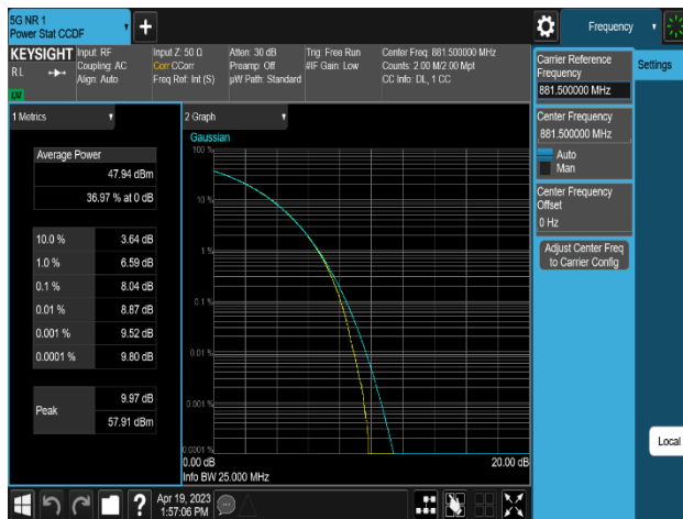
Plot 8-205. Peak To Average Power Ratio Plot (NR n5_2C_10M+15M_QPSK - Mid Channel_2T, Port 0)
