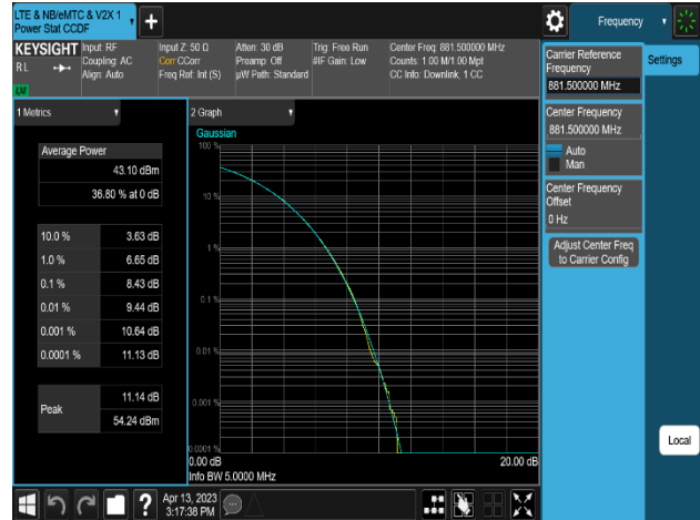
Plot 8-232. Peak To Average Power Ratio Plot (LTE B5_1C_5M_16QAM - Mid Channel_4T, Port 1)
