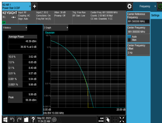
Plot 8-257. Peak To Average Power Ratio Plot (MSR 2C_NR n5_1C_5M+LTE B5_1C_5M_QPSK - Mid Channel_4T, Port 1)
