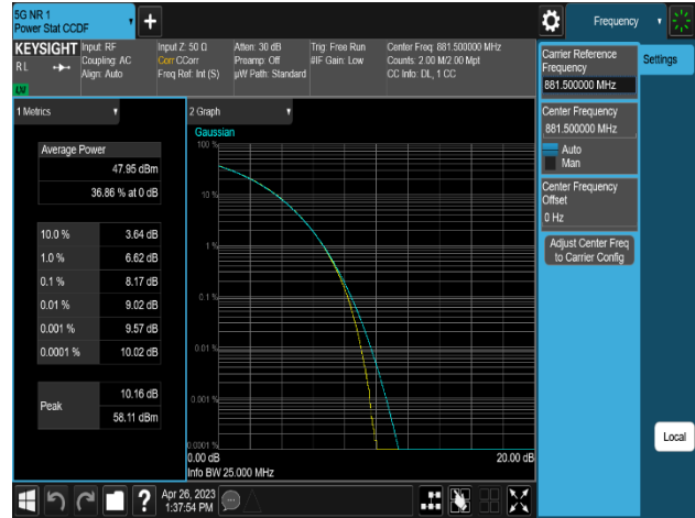
Plot 8-222. Peak To Average Power Ratio Plot (MSR 3C_DSS B(n)5_1C_10M+NR n5_1C_10M+LTE B5_1C_5M_16QAM - Mid Channel_2T, Port 0)
