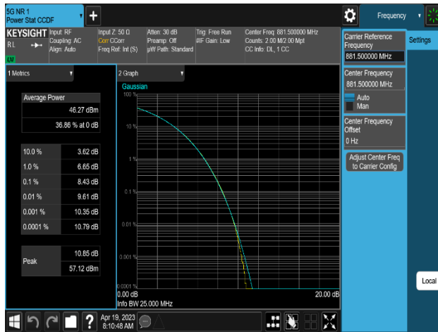
Plot 8-251. Peak To Average Power Ratio Plot (NR n5_2C_10M+15M_QPSK - Mid Channel_4T, Port 1)
