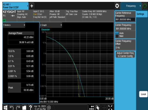
Plot 8-248. Peak To Average Power Ratio Plot (NR n5_1C_15M_64QAM - Mid Channel_4T, Port 1)
