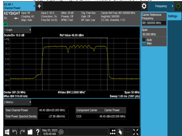
Plot 8-168. Conducted Average Output Power Plot (MSR 3C_DSS B(n)5_1C_10M+NR n5_1C_10M+LTE B5_1C_5M_4T_16QAM - Middle Channel, Port 0)
