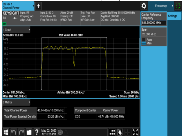
Plot 8-158. Conducted Average Output Power Plot (MSR 2C_NR n5_1C_5M+LTE B5_1C_5M_4T_16QAM - Middle Channel, Port 0)
