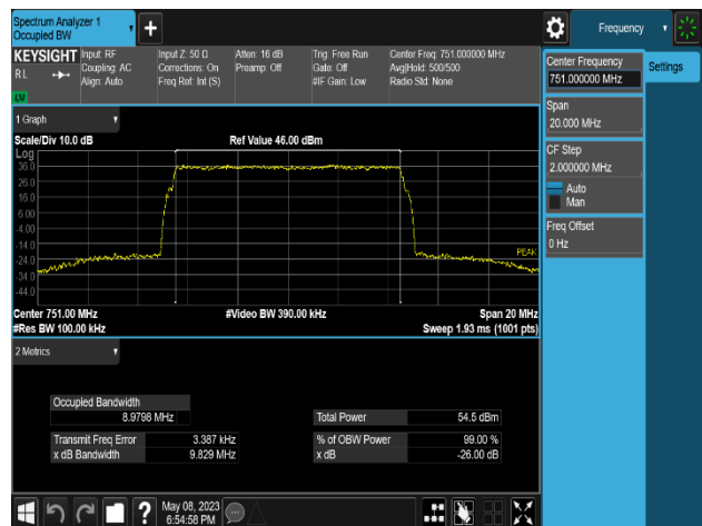
Plot 8-88. Occupied Bandwidth Plot (LTE B13_1C_10M_64QAM - Mid Channel_4T, Port 0)
