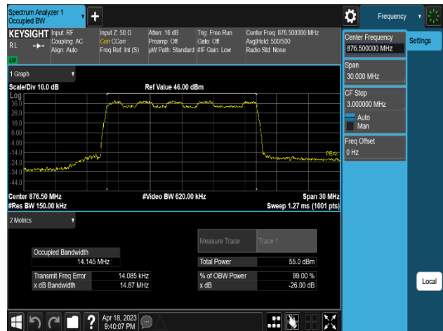
Plot 8-64. Occupied Bandwidth Plot (NR n5_1C_15M_16QAM - Low Channel_4T, Port 0)
