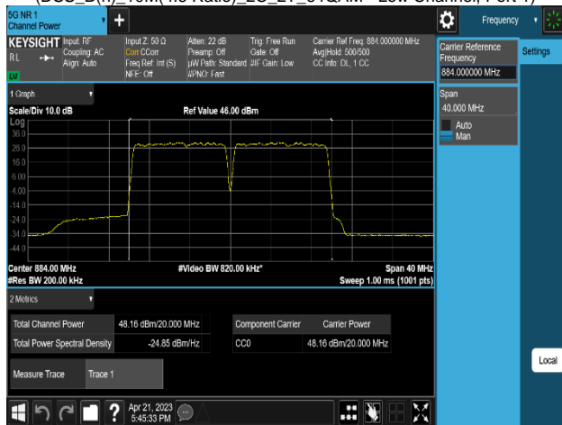
Plot 8-104. Conducted Average Output Power Plot (DSS_B(n)_2C_10M+10M_2T_QPSK - High Channel, Port 1)
