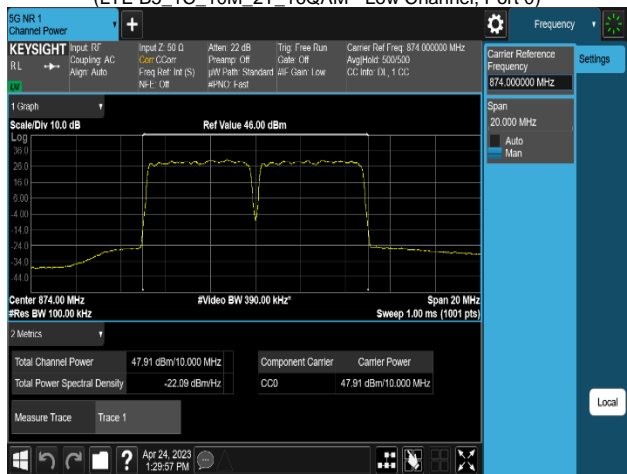
Plot 8-98. Conducted Average Output Power Plot (LTE B5_2C_5M+5M_2T_16QAM - Low Channel, Port 1)
