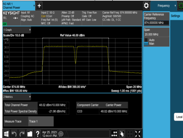
Plot 8-119. Conducted Average Output Power Plot (MSR 2C_NR n5_1C_5M+LTE B5_1C_5M_2T_QPSK - Low Channel, Port 1)
