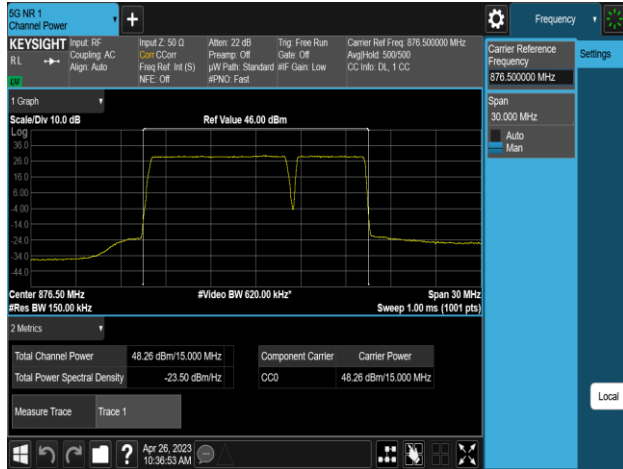
Plot 8-123. Conducted Average Output Power Plot (MSR 2C_DSS B(n)5_1C_10M+NR n5_1C_5M_2T_QPSK - Low Channel, Port 1)
