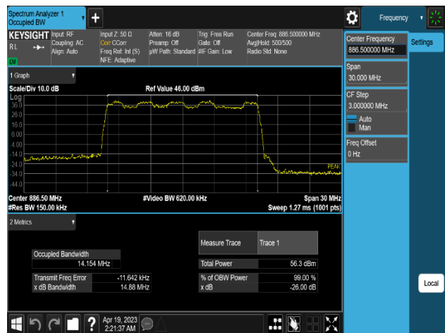
Plot 8-18. Occupied Bandwidth Plot (NR n5_1C_15M_16QAM - High Channel_2T, Port 1)
