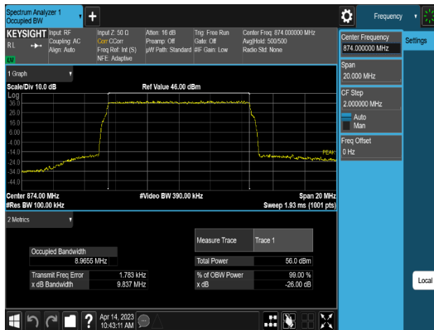
Plot 8-3. Occupied Bandwidth Plot (LTE B5_1C_10M_QPSK - Low Channel_2T, Port 1)
