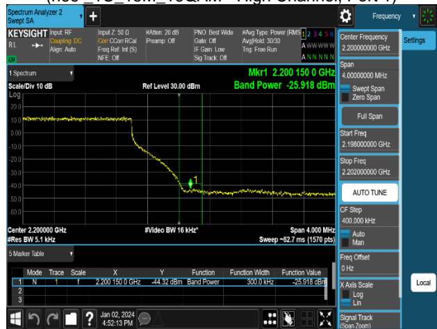
Plot 8-34. Band Edge Emission Plot (n66_1C_30M_QPSK - High Channel, Port 3)
