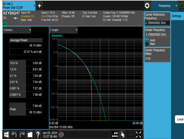
Plot 8-25. Peak To Average Power Ratio Plot (n66_1C_15M_QPSK - Mid Channel, Port 3)
