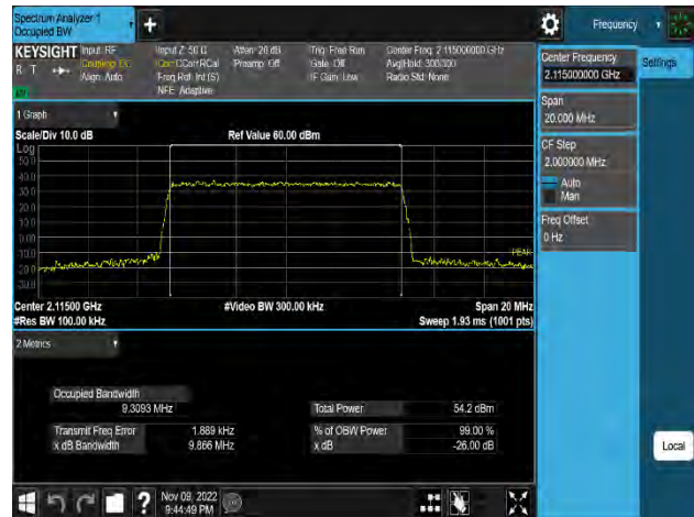
Plot 8-2. Occupied Bandwidth Plot (n66 1C 10M 256QAM - Low Channel, Port 0)
