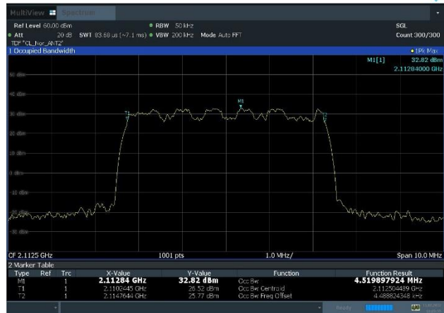
Plot 8-2. Occupied Bandwidth Plot (n66_1C_5M_16QAM - Low Channel, Port 2)
