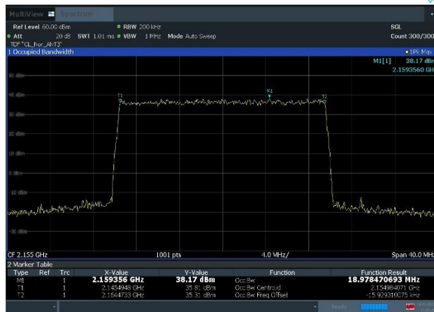
Plot 8-3. Occupied Bandwidth Plot (n66_1C_20M_QPSK - Mid Channel, Port 3)
