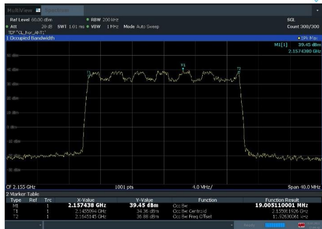
Plot 8-4. Occupied Bandwidth Plot (n66_1C_20M_16QAM - Mid Channel, Port 1)
