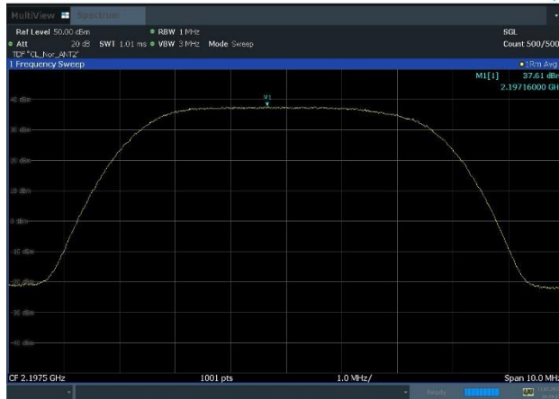
Plot 8-11. Power Spectral Density Plot (n66_1C_5M_16QAM - High Channel, Port 2)
