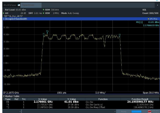
Plot 8-6. Occupied Bandwidth Plot (n66_2C_5M+20M_16QAM - High Channel, Port 3)
