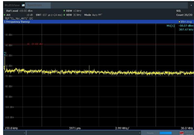
Plot 8-63. Conducted Spurious Emission Plot 150 kHz to 30 MHz (n66_2C_5M+20M_16QAM - Low Channel, Port 1)
