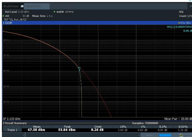
Plot 8-29. Peak To Average Power Ratio Plot (n66_2C_5M+20M_QPSK - Low Channel, Port 2)
