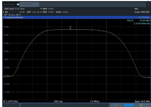
Plot 8-10. Power Spectral Density Plot (n66_1C_5M_16QAM - High Channel, Port 1)
