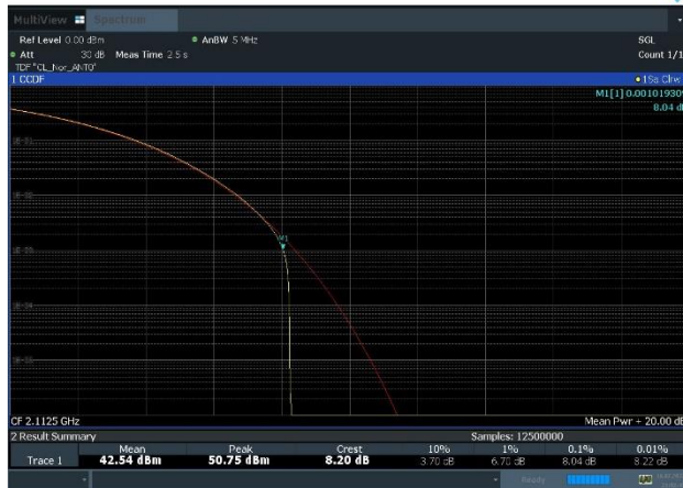
Plot 8-25. Peak To Average Power Ratio Plot (n66_1C_5M_QPSK - Low Channel, Port 0)
