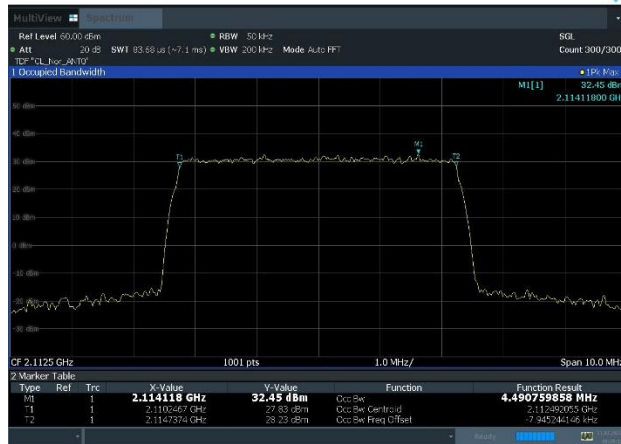
Plot 8-1. Occupied Bandwidth Plot (n66_1C_5M_QPSK - Low Channel, Port 0)
