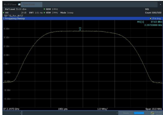
Plot 8-12. Power Spectral Density Plot (n66_1C_5M_16QAM - High Channel, Port 3)
