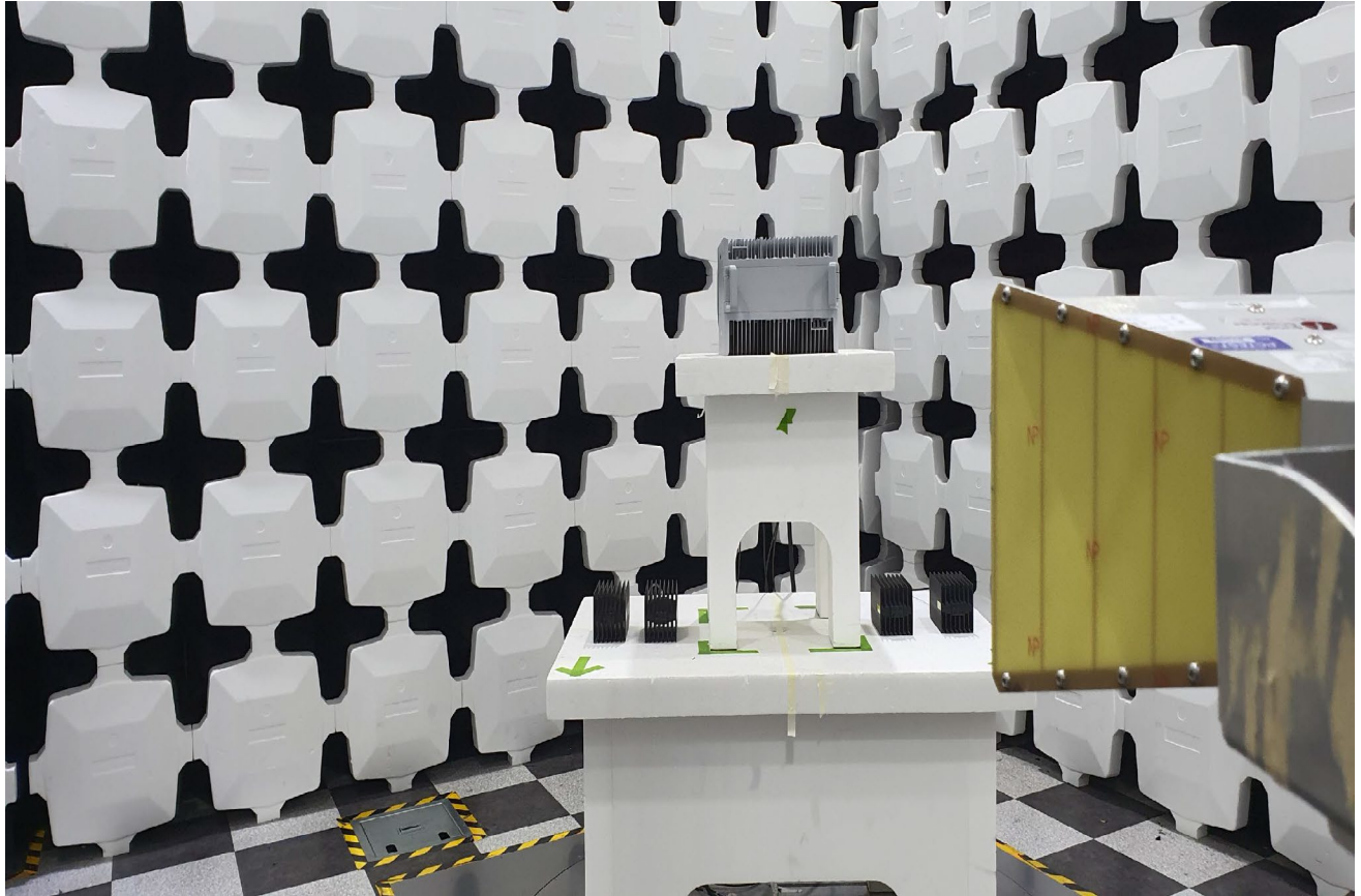
Above 1GHz Test Instrument & Measurement Setup > 1GHz
