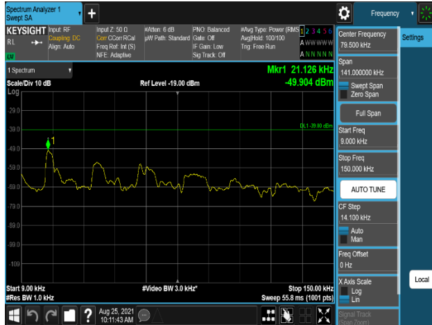
Plot 7-469. Conducted Spurious Emission Plot 9 kHz to 150 kHz (Multi Band_B5_5M+10M(DSS)_2C + B13_10M+NB-lot(GB)+NB-lot(IB)_3C_QPSK -- High Channel, Port 3)
