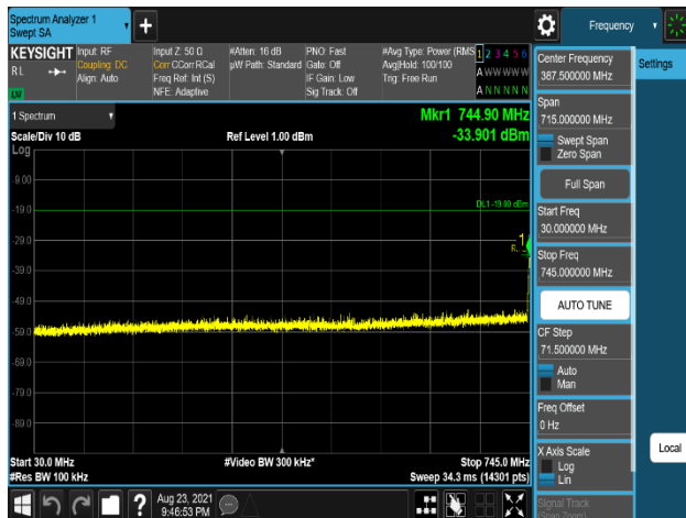
Plot 7-471. Conducted Spurious Emission Plot 30 MHz to 858 MHz (Multi Band_B5_10M(DSS)_1C+ B13_10M+NB-lot(GB)+NB-lot(IB)_3C_QPSK -- High Channel, Port 3)
