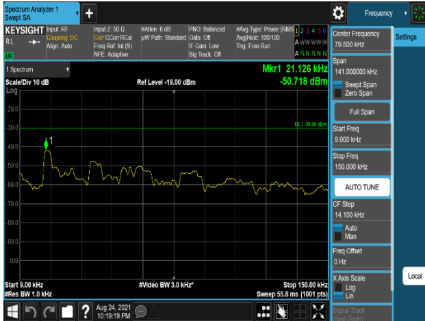
Plot 7-463. Conducted Spurious Emission Plot 9 kHz to 150 kHz (DSS_B5_10M_8:2)_1C_256QAM -- High Channel, Port 3)
