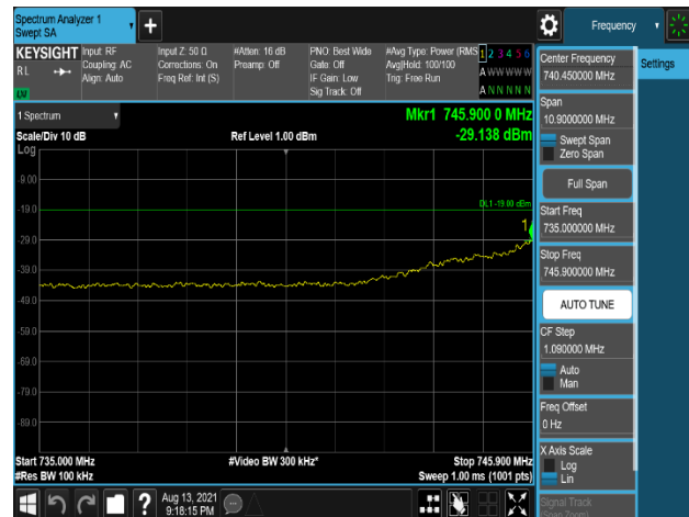
Plot 7-422. Conducted Spurious Emission Plot 735 MHz to 745.9 MHz (LTE_B13_10M+High_NB-lot(IB)+High_NB-lot(IB)_1C_QPSK - Port 3)
