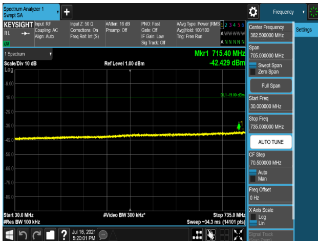
Plot 7-427. Conducted Spurious Emission Plot 30 MHz to 735 MHz (LTE_B13_10M+Low_NB-lot(GB)+High_NB-lot(GB)_3C_QPSK - Port 2)
