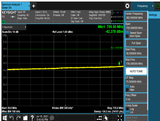
Plot 7-391. Conducted Spurious Emission Plot 30 MHz to 735 MHz (LTE_B13_10M_1C_16QAM - Port 2)
