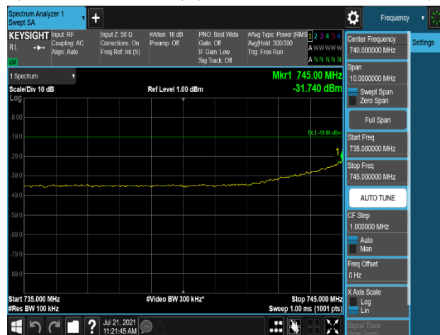
Plot 7-404. Conducted Spurious Emission Plot 735 MHz to 745.9 MHz (LTE_B13_10M+ NB-IoT(IB)_1C_QPSK - Low Channel, Port 3)
