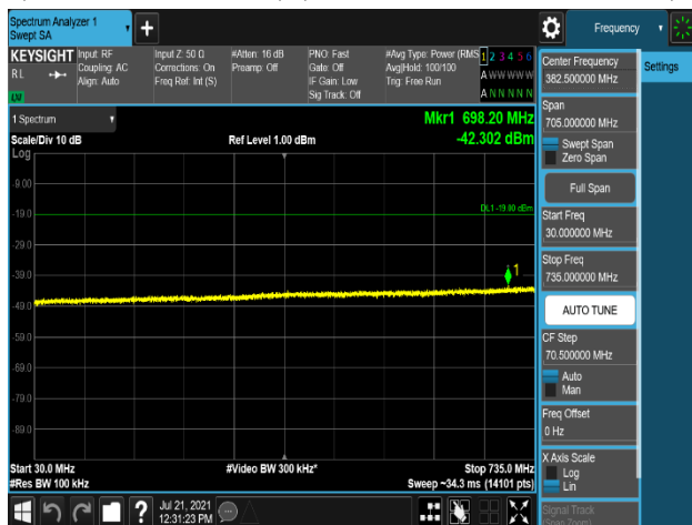
Plot 7-403. Conducted Spurious Emission Plot 30 MHz to 735 MHz (LTE_B13_10M+ NB-IoT(IB)_1C_QPSK - High Channel, Port 0)
