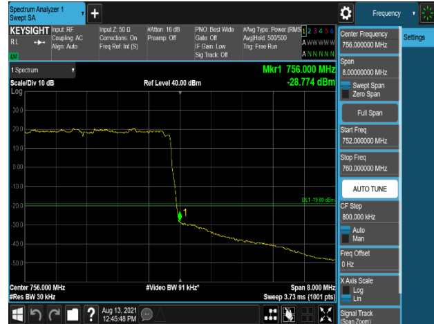
Plot 7-310. Band Edge Emission (756MHz to 756.1MHz) Plot (LTE_B13_5M_1C_16QAM - High Channel, Port 3)
