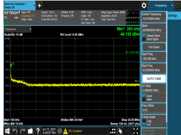
Plot 7-342. Conducted Spurious Emission Plot 150 kHz to 30 MHz (LTE_B5_5M_1C_256QAM - Low Channel, Port 2)
