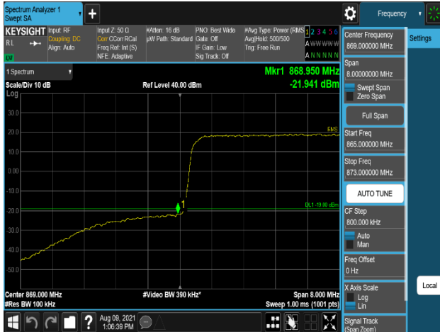
Plot 7-337. Band Edge Emission (868MHz to 869MHz) Plot (DSS_B5_10M+5M_2C_QPSK - Low Channel, Port 2)
