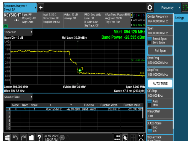
Plot 7-304. Band Edge Emission (894MHz to 895MHz) Integration method Plot (B2 5M+10M+10M 3C 16QAM - Low Channel, Port 2)
