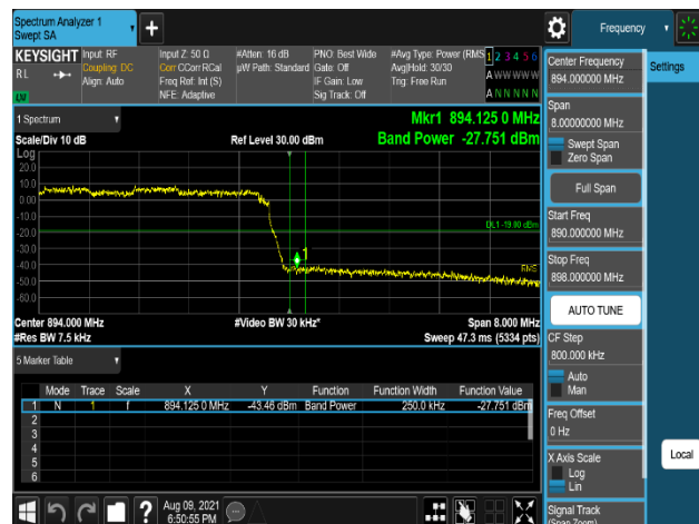
Plot 7-336. Band Edge Emission (894MHz to 895MHz) Integration method Plot (DSS_B5_10M+10M+5M_3C_16QAM - High Channel, Port 2)
