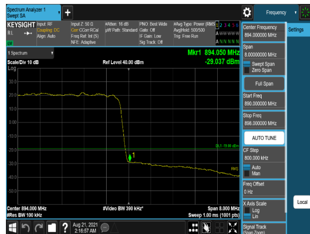
Plot 7-330. Band Edge Emission (984MHz to 895MHz) Plot (DSS_B5_10M_5:5)_1C_64QAM - High Channel, Port 0)
