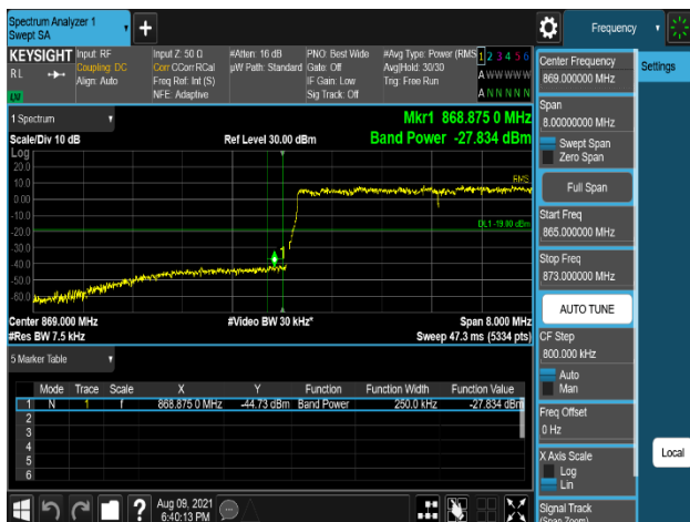
Plot 7-335. Band Edge Emission (868MHz to 869MHz) Integration method Plot (DSS_B5_10M+10M+5M_3C_16QAM - Low Channel, Port 2)
