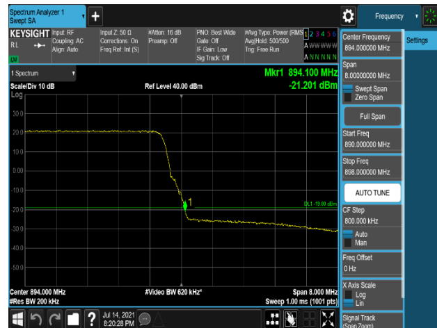
Plot 7-302. Band Edge Emission (894MHz to 895MHz) Plot (LTE_B5_10M+10M_2C_QPSK - High Channel, Port 0)
