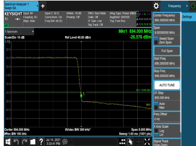
Plot 7-300. Band Edge Emission (894MHz to 895MHz) Plot (LTE_B5_5M+5M_2C_64QAM - High Channel, Port 2)
