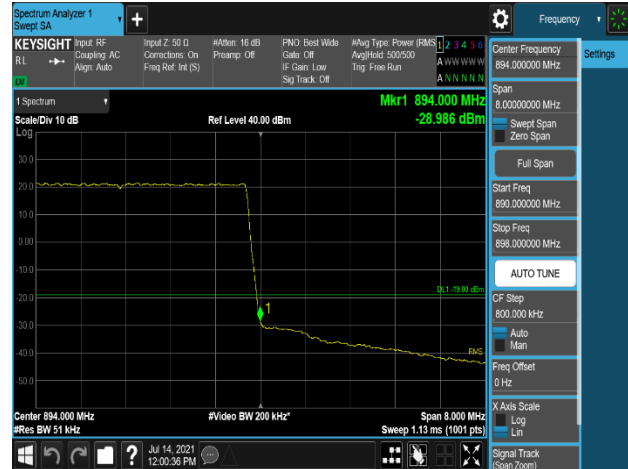
Plot 7-296. Band Edge Emission (894MHz to 895MHz) Plot (LTE_B5_5M_1C_256QAM - High Channel, Port 1)
