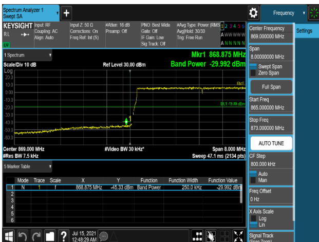
Plot 7-303. Band Edge Emission (868MHz to 869MHz) Integration method Plot (B2 5M+10M+10M 3C QPSK - Low Channel, Port 0)
