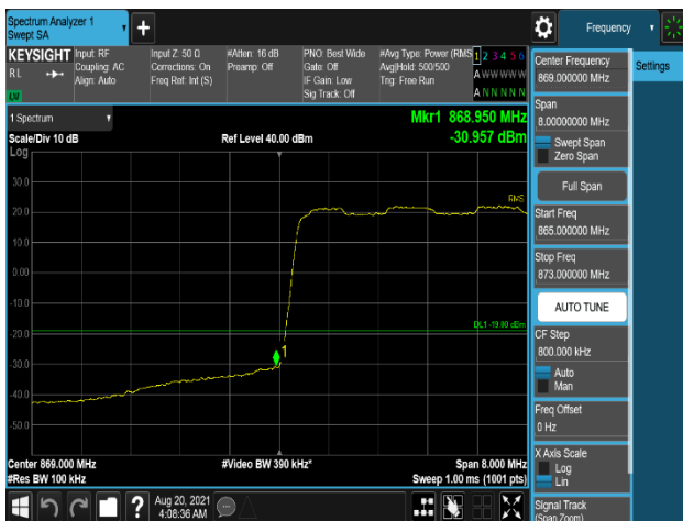
Plot 7-329. Band Edge Emission (868MHz to 869MHz) Plot (DSS_B5_10M_5:5)_1C_16QAM - Low Channel, Port 0)
