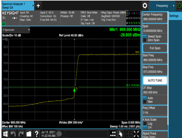
Plot 7-299. Band Edge Emission (868MHz to 869MHz) Plot (LTE_B5_5M+5M_2C_QPSK - Low Channel, Port 0)
