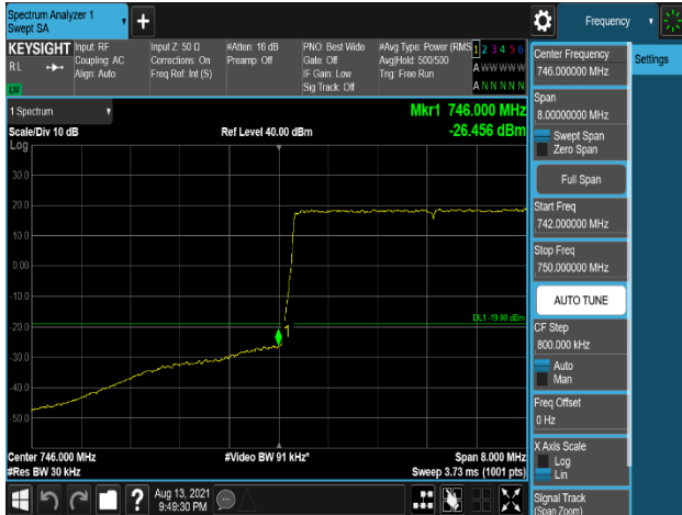
Plot 7-309. Band Edge Emission (745.9MHz to 746MHz) Plot (LTE_B13_5M_1C_64QAM - Low Channel, Port 1)
