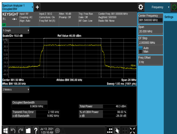
Plot 7-17. Occupied Bandwidth Plot (LTE_B5_10M_1C_QPSK - Mid Channel, Port 1)
