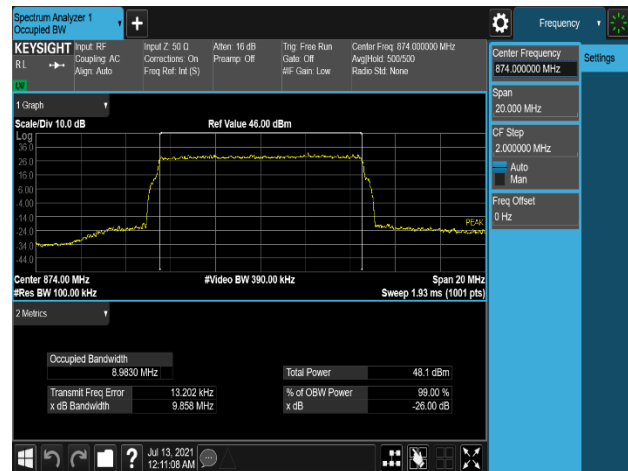
Plot 7-16. Occupied Bandwidth Plot (LTE_B5_10M_1C_256QAM - Low Channel, Port 0)
