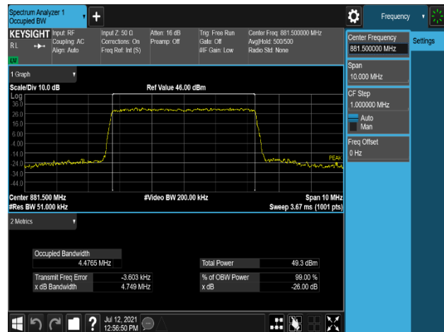
Plot 7-6. Occupied Bandwidth Plot (LTE_B5_5M_1C_16QAM - Mid Channel, Port 0)
