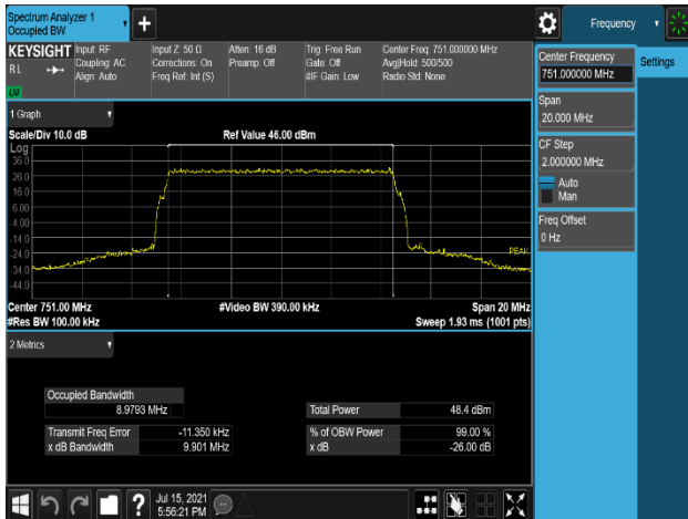
Plot 7-67. Occupied Bandwidth Plot (LTE_B13_10M_1C_64QAM - Port 0)
