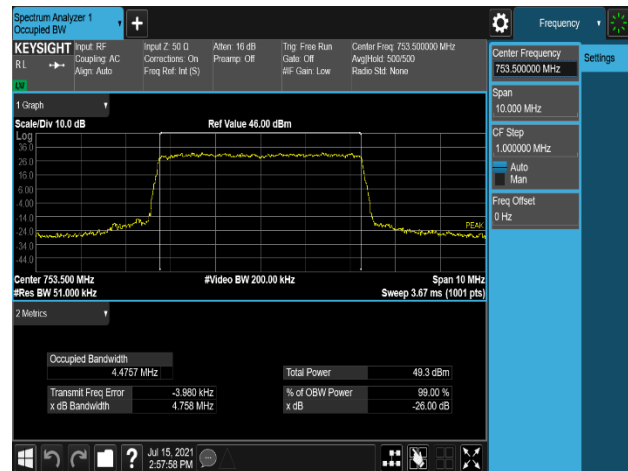
Plot 7-62. Occupied Bandwidth Plot (LTE_B13_5M_1C_16QAM - High Channel, Port 1)
