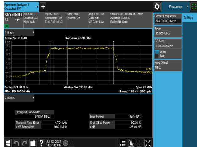
Plot 7-14. Occupied Bandwidth Plot (LTE_B5_10M_1C_16QAM - Low Channel, Port 0)
