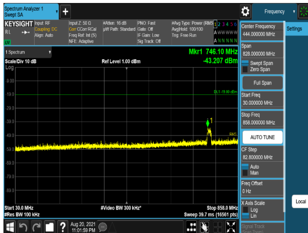
Plot 7-465. Conducted Spurious Emission Plot 30 MHz to 858 MHz (DSS_B5_10M_8:2)_1C_256QAM -- High Channel, Port 3)
