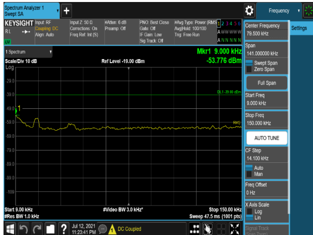
Plot 7-347. Conducted Spurious Emission Plot 9 kHz to 150 kHz (LTE_B5_10M_1C_QPSK - Low Channel, Port 0)
