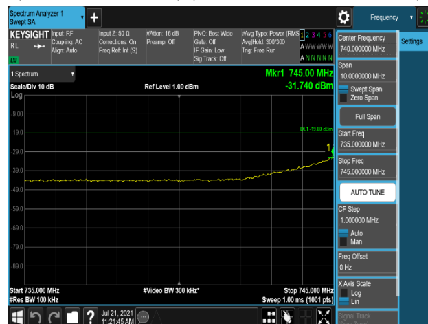
Plot 7-404. Conducted Spurious Emission Plot 735 MHz to 745.9 MHz (LTE_B13_10M+ NB-IoT(IB)_1C_QPSK - Low Channel, Port 3)
