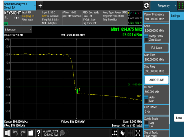
Plot 7-332. Band Edge Emission (984MHz to 895MHz) Plot (DSS_B5_10M+5M_2C_64QAM - High Channel, Port 2)
