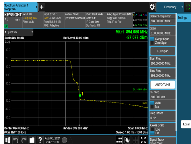
Plot 7-340. Band Edge Emission (984MHz to 895MHz) Plot (DSS_B5_10M+10M_2C_64QAM - High Channel, Port 2)
