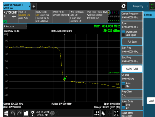
Plot 7-330. Band Edge Emission (894MHz to 895MHz) Plot (DSS_B5_10M_5:5_1C_64QAM - High Channel, Port 0)
