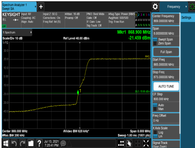
Plot 7-301. Band Edge Emission (868MHz to 869MHz) Plot (LTE_B5_10M+10M_2C_64QAM - Low Channel, Port 1)
