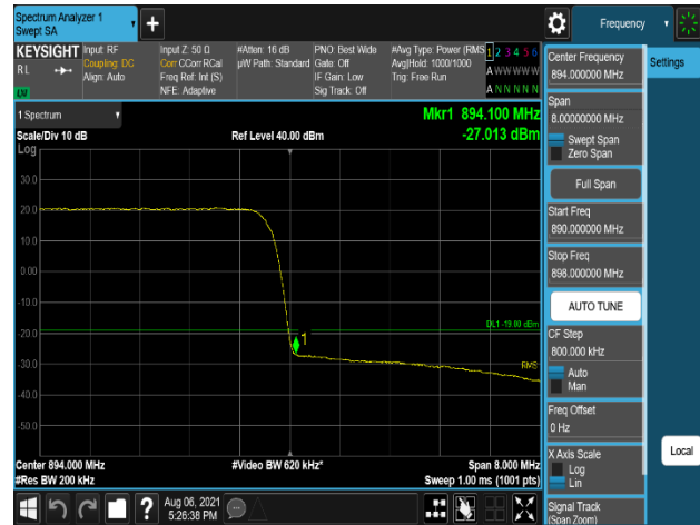
Plot 7-334. Band Edge Emission (984MHz to 895MHz) Plot (DSS_B5_10M+10M_2C_64QAM - High Channel, Port 0)
