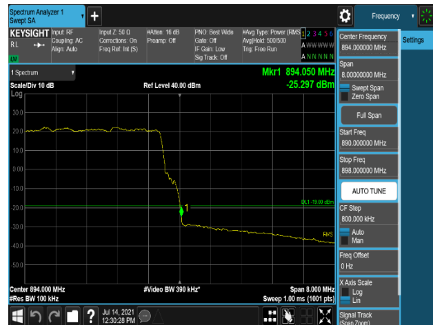
Plot 7-298. Band Edge Emission (894MHz to 895MHz) Plot (LTE_B5_10M_1C_16QAM - High Channel, Port 2)
