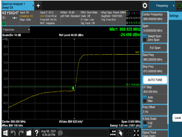
Plot 7-331. Band Edge Emission (868MHz to 869MHz) Plot (DSS_B5_10M+5M_2C_QPSK - Low Channel, Port 2)
