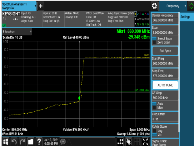
Plot 7-295. Band Edge Emission (868MHz to 869MHz) Plot (LTE_B5_5M_1C_256QAM - Low Channel, Port 1)
