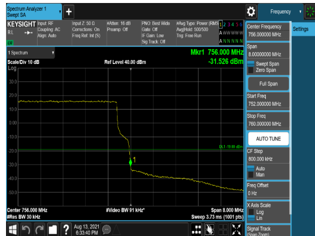
Plot 7-312. Band Edge Emission (756MHz to 757MHz) Plot (LTE_B5_10M_1C_256QAM - High Channel, Port 3)
