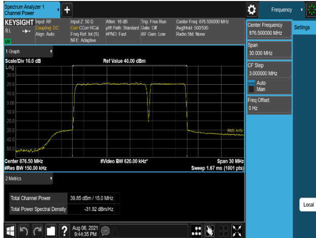
Plot 7-238. Conducted Average Output Power Plot (DSS_B5_10M+5M_2C_64QAM - Low Channel, Port 0)
