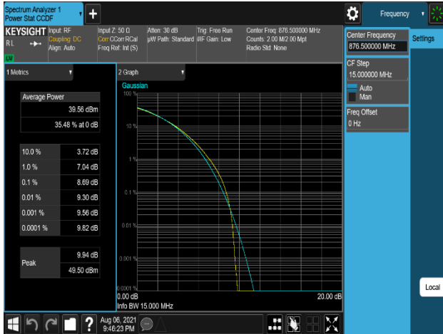
Plot 7-285. Peak To Average Power Ratio Plot (DSS_B5_10M+5M_2C_64QAM - Low Channel, Port 3)
