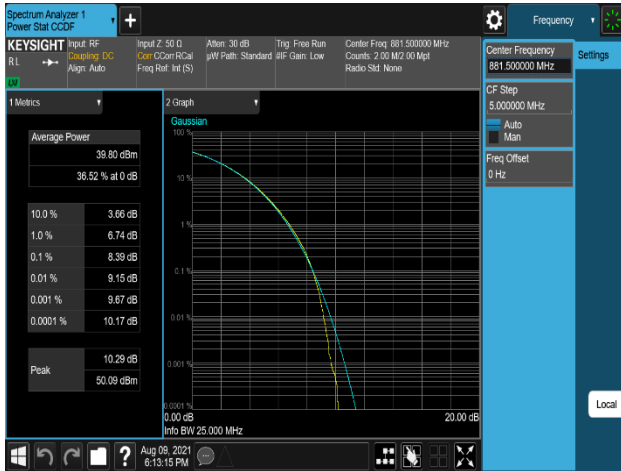
Plot 7-291. Peak To Average Power Ratio Plot (DSS_B5_10M+10M+5M_3C_QPSK - Port 3)
