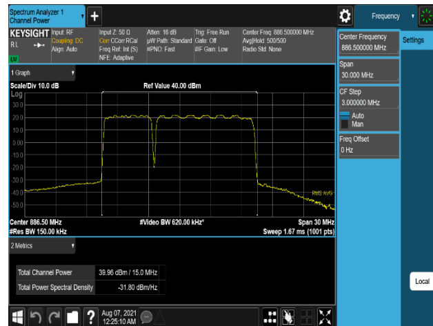
Plot 7-247. Conducted Average Output Power Plot (DSS_B5_10M+5M_2C_16QAM - High Channel, Port 1)
