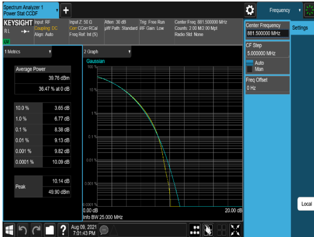
Plot 7-293. Peak To Average Power Ratio Plot (DSS_B5_10M+10M+5M_3C_64QAM - Port 3)
