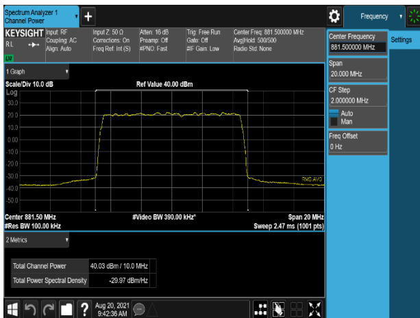
Plot 7-232. Conducted Average Output Power Plot (DSS_B5_10M_9:1)_1C_64QAM - Mid Channel, Port 2)
