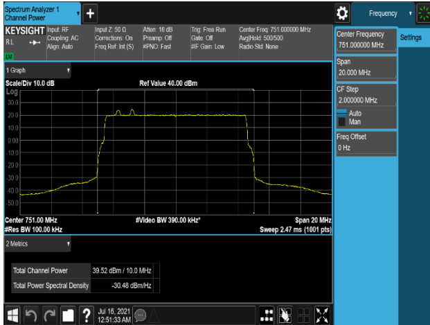
Plot 7-204. Conducted Average Output Power Plot (LTE_B13_10M+Low_NB-lot(IB)+Low_NB-lot(IB)_1C - Port 2)
