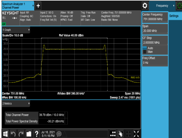
Plot 7-210. Conducted Average Output Power Plot (LTE_B13_10M+Low_NB-lot(GB)+High_NB-lot(GB)_3C - Port 0)
