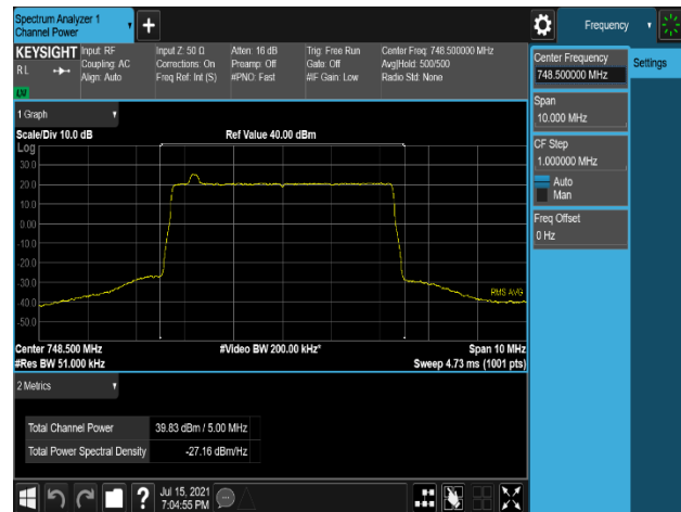
Plot 7-189. Conducted Average Output Power Plot (LTE_B13_5M+NB-lot(IB)_1C_QPSK - Low Channel, Port 3)
