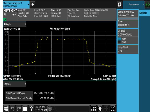
Plot 7-205. Conducted Average Output Power Plot (LTE_B13_10M+Low_NB-lot(IB)+Low_NB-lot(IB)_1C - Port 3)
