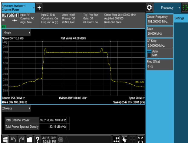
Plot 7-214. Conducted Average Output Power Plot (LTE_B13_10M+Low_NB-lot(GB)+High_NB-lot(IB)_2C - Port 0)
