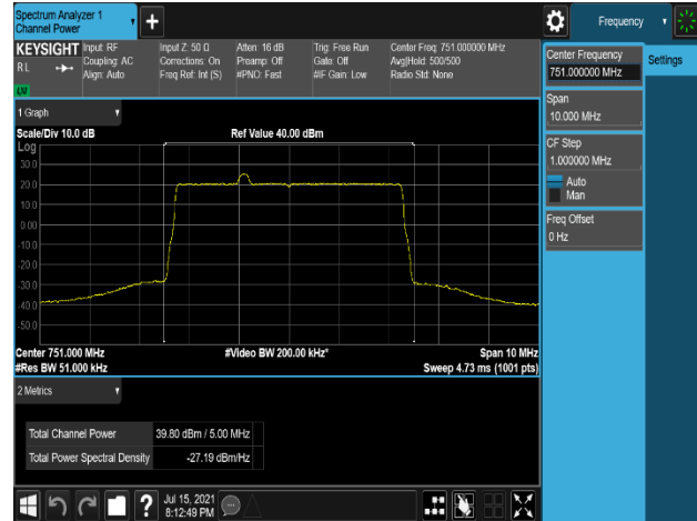
Plot 7-193. Conducted Average Output Power Plot (LTE_B13_5M+NB-IoT(IB)_1C_QPSK - Mid Channel, Port 3)
