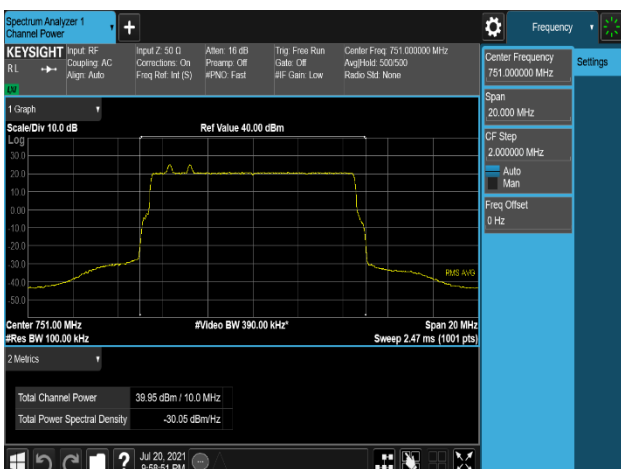
Plot 7-202. Conducted Average Output Power Plot (LTE_B13_10M+Low_NB-lot(IB)+Low_NB-lot(IB)_1C - Port 0)
