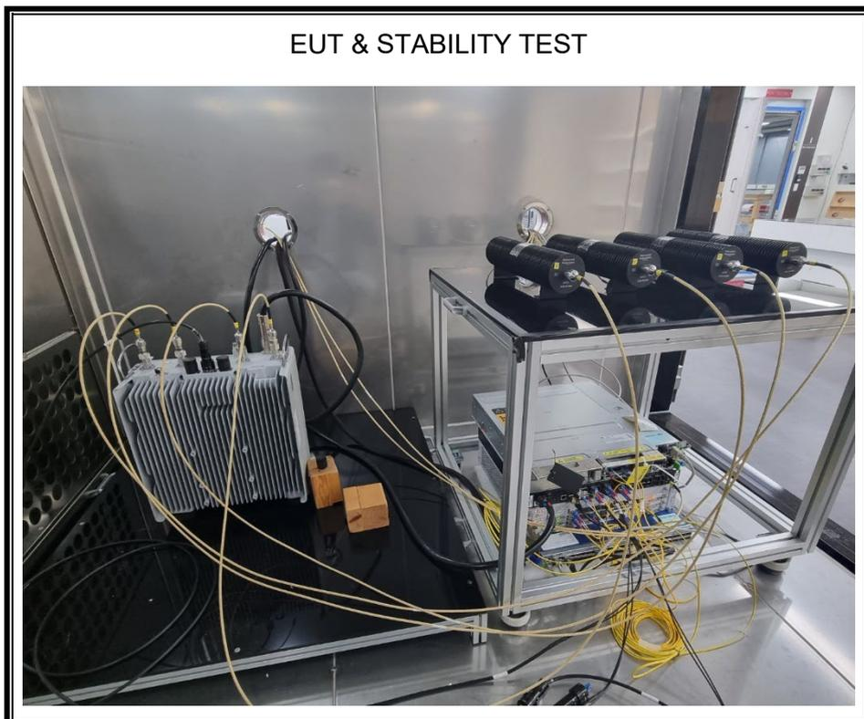
2) RADIATED RF MEASUREMENT SETUP
