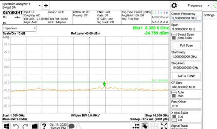
**5G NR, Single carrier 20 MHz, High Channel, 16QAM
