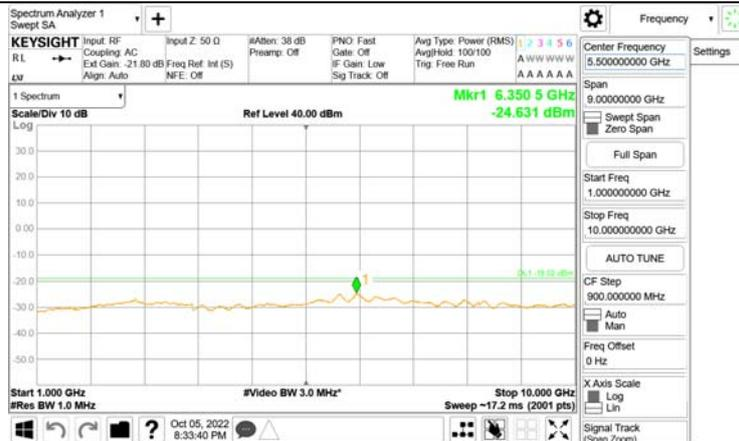
LTE, Single carrier 20 MHz, Low Channel, 16QAM
