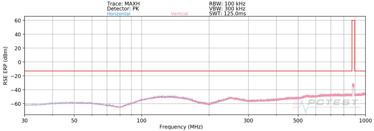
**Plot 7-913. Radiated spurious emission\_30 MHz to 1000 MHz
