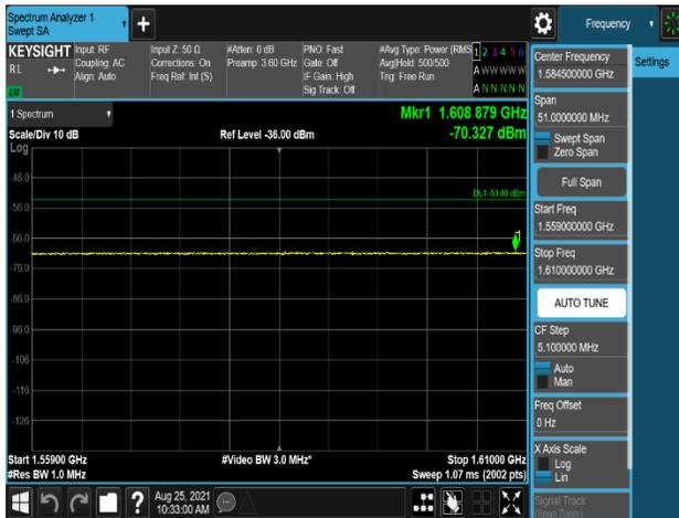
**Plot 7-867. Conducted Spurious Emission Plot 1559 MHz to 1610 MHz (B13\_5M+NB-lot(GB)\_1C\_2T\_QPSK – Middle channel - Port 1)**
