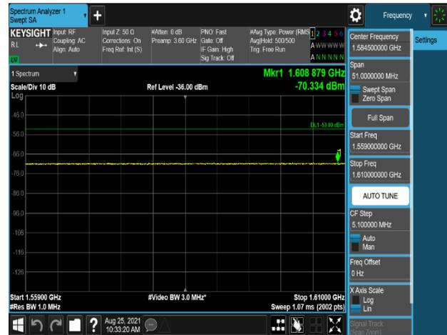
**Plot 7-868. Conducted Spurious Emission Plot 1559 MHz to 1610 MHz (B13\_5M+NB-lot(GB)\_1C\_2T\_QPSK – High channel - Port 0)**
