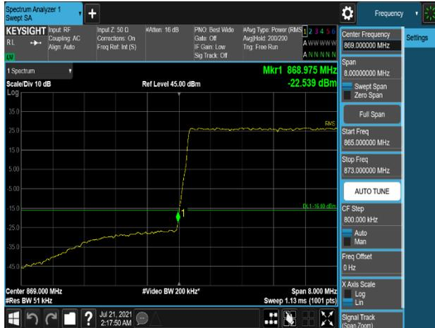
Plot 7-593. Band Edge Emission (868MHz to 869MHz) Plot (B5\_5M+5M\_2C\_256QAM\_Non-contiguous Low Channel, Port 1)
