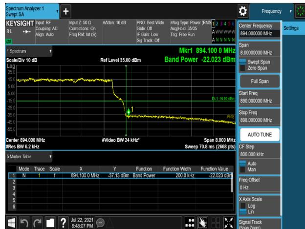
Plot 7 860. Band Edge Emission (894MHz to 895MHz) Plot (B5\_10M+10M\_2C\_16QAM\_Non-contiguous - High Channel, Port 0)
