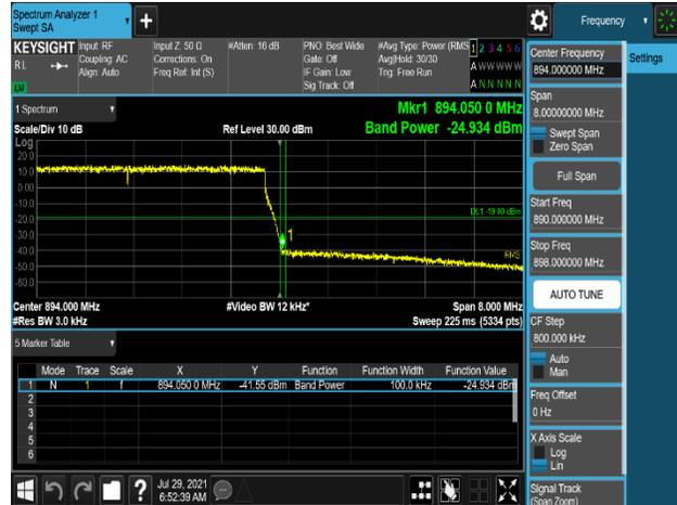
Plot 7-586. Band Edge Emission (894MHz to 895MHz) Plot (B5\_5M+5M\_2C\_64QAM - High Channel, Port 3)
