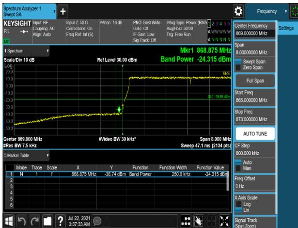
Plot 7-591. Band Edge Emission (868MHz to 869MHz) Plot (B2\_5M+10M+10M\_3C\_64QAM - Low Channel, Port 3)
