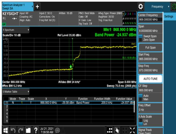
Plot 7-583. Band Edge Emission (868MHz to 869MHz) Plot (B5\_10M+10M\_2C\_16QAM - Low Channel, Port 1)
