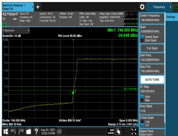
Plot 7-607. Band Edge Emission (745.9MHz to 746MHz) Plot (B13\_5M+5M\_2C\_QPSK - Low Channel, Port 1)
