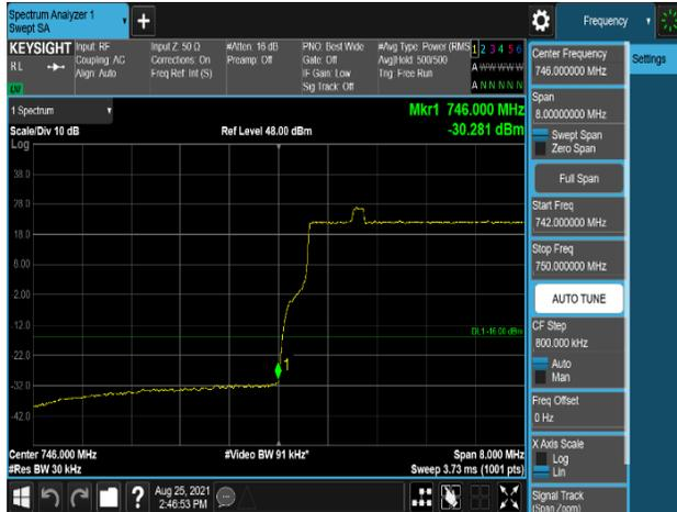
Plot 7-615. Band Edge Emission (745.9MHz to 746MHz) Plot (B13\_10M+Low\_NB-lot(IB)+High\_NB-lot(IB)\_3C – Port 0)
