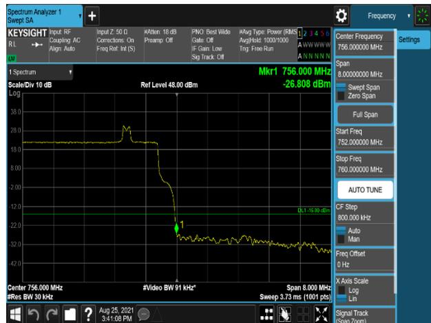
Plot 7-630. Band Edge Emission (756MHz to 756.1MHz) Plot (B13\_10M+Low\_NB-lot(IB)+Low\_NB-lot(IB)\_1C – Port 1)
