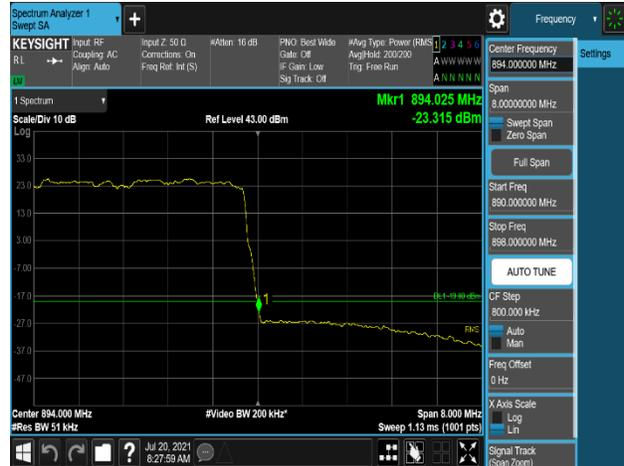
Plot 7 860. Band Edge Emission (894MHz to 895MHz) Plot
