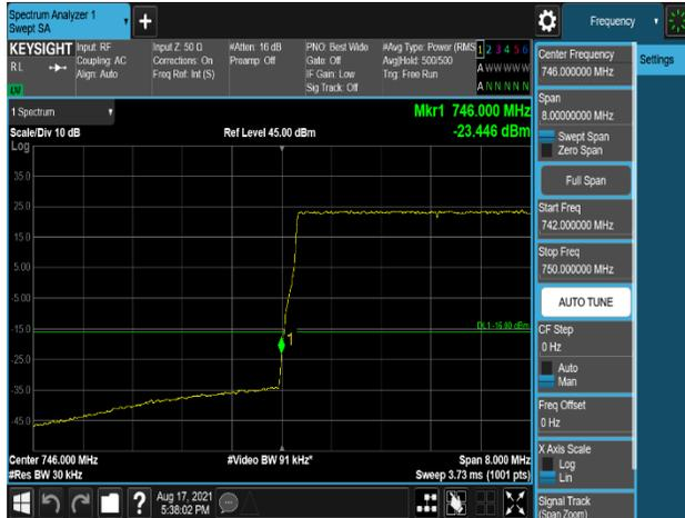
Plot 7-597. Band Edge Emission (745.9MHz to 746MHz) Plot (B13\_5M\_1C\_QPSK - Low Channel, Port 1)
