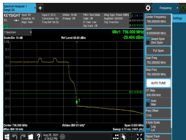
Plot 7-620. Band Edge Emission (756MHz to 756.1MHz) Plot (B13\_10M+High\_NB-lot(IB)+High\_NB-lot(IB)\_1C – Port 1)
