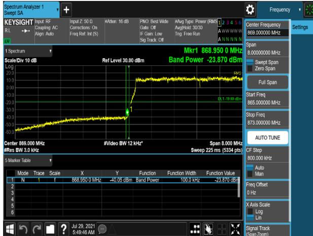
Plot 7-585. Band Edge Emission (868MHz to 869MHz) Plot (B5\_5M+5M\_2C\_16QAM - Low Channel, Port 3)
