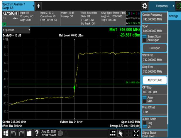
Plot 7-605. Band Edge Emission (745.9MHz to 746MHz) Plot (B13\_5M+5M\_2C\_16QAM - Low Channel, Port 1)
