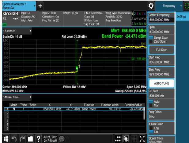
Plot 7-581. Band Edge Emission (868MHz to 869MHz) Plot (B5\_5M+5M\_2C\_16QAM - Low Channel, Port 1)
