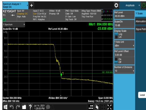
Plot 7-580. Band Edge Emission (894MHz to 895MHz) Plot (B5\_10M\_1C\_QPSK - High Channel, Port 3)
