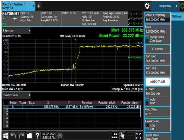
Plot 7-589. Band Edge Emission (868MHz to 869MHz) Plot (B2\_5M+10M+10M\_3C\_16QAM - Low Channel, Port 0)
