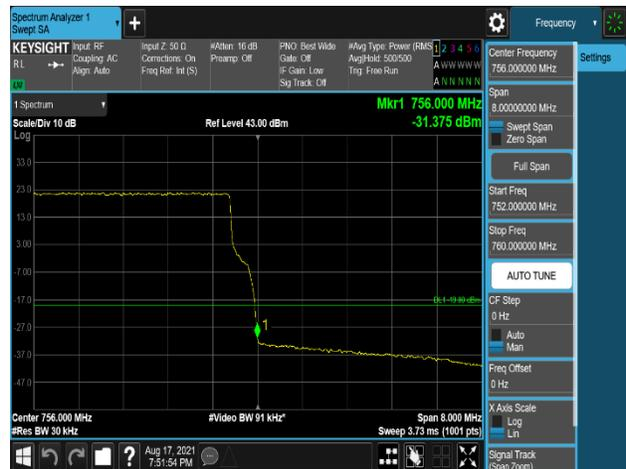
Plot 7-604. Band Edge Emission (756MHz to 756.1MHz) Plot (B13\_10M\_1C\_64QAM - High Channel, Port 1)
