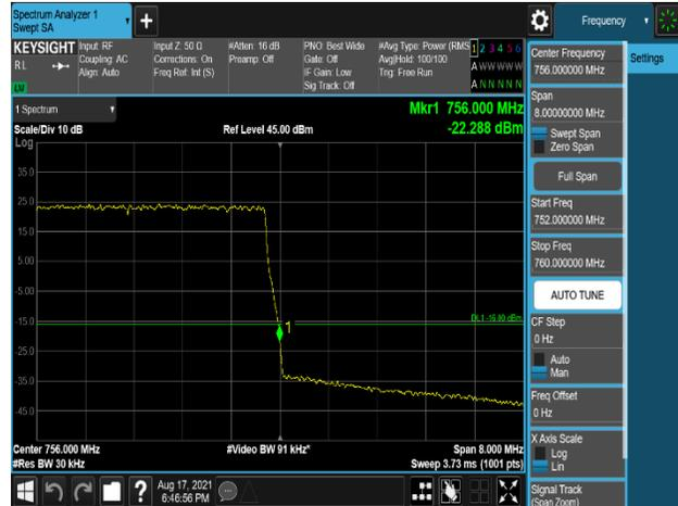
Plot 7-598. Band Edge Emission (756MHz to 756.1MHz) Plot (B13\_5M\_1C\_256QAM - High Channel, Port 1)
