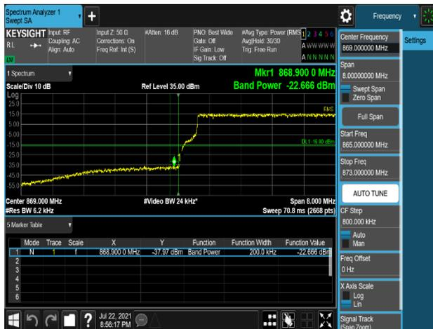
Plot 7-594. Band Edge Emission (868MHz to 869MHz) Plot (B5\_10M+10M\_2C\_64QAM\_Non-contiguous - Low Channel, Port 0)
