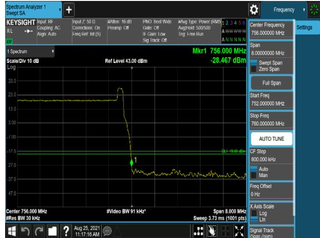
Plot 7-634. Band Edge Emission (756MHz to 756.1MHz) Plot (B13\_10M+Low\_NB-lot(IB)+High\_NB-lot(IB)\_1C – Port 2)
