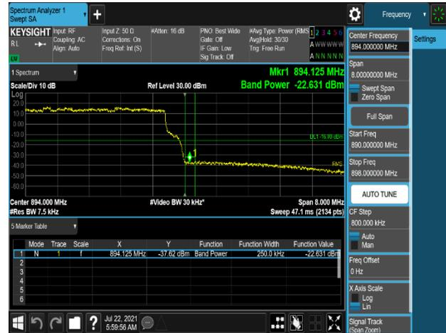
Plot 7-590. Band Edge Emission (894MHz to 895MHz) Plot (B2\_5M+10M+10M\_3C\_16QAM - High Channel, Port 0)
