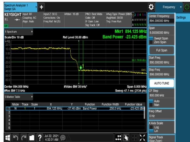
Plot 7-592. Band Edge Emission (894MHz to 895MHz) Plot (B2\_5M+10M+10M\_3C\_16QAM - High Channel, Port 3)
