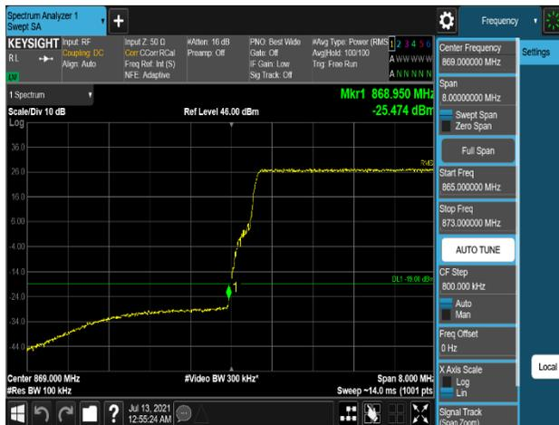
Plot 7-579. Band Edge Emission (868MHz to 869MHz) Plot (B5\_10M\_1C\_256QAM - Low Channel, Port 1)
