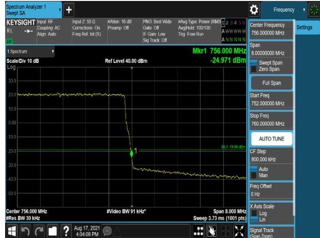
Plot 7-602. Band Edge Emission (756MHz to 756.1MHz) Plot (B13\_5M\_1C\_64QAM - High Channel, Port 3)
