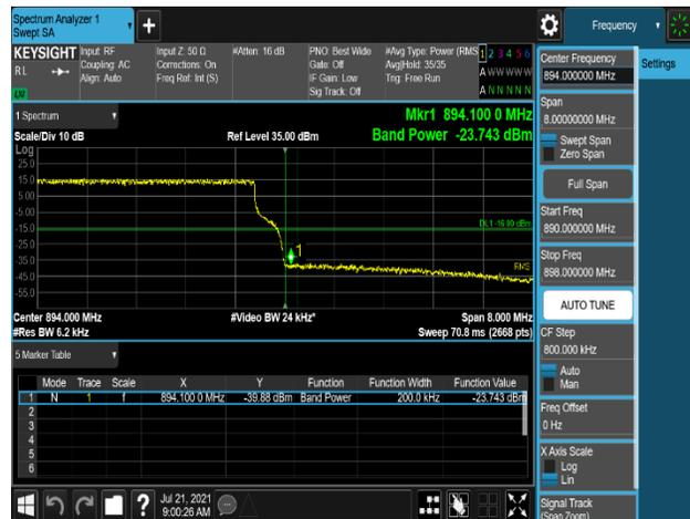
Plot 7-584. Band Edge Emission (894MHz to 895MHz) Plot (B5\_10M+10M\_2C\_256QAM - High Channel, Port 0)
