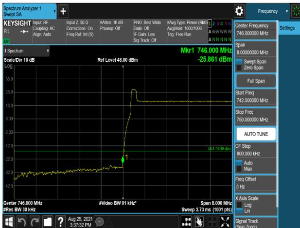
Plot 7-629. Band Edge Emission (745.9MHz to 746MHz) Plot (B13\_10M+Low\_NB-lot(IB)+Low\_NB-lot(IB)\_1C – Port 0)
