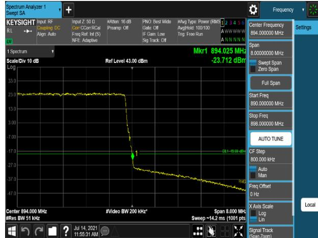
Plot 7-578. Band Edge Emission (894MHz to 895MHz) Plot (B5\_5M\_1C\_64QAM - High Channel, Port 2)
