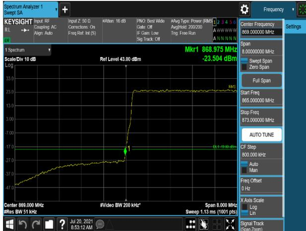
Plot 7-595. Band Edge Emission (868MHz to 869MHz) Plot
