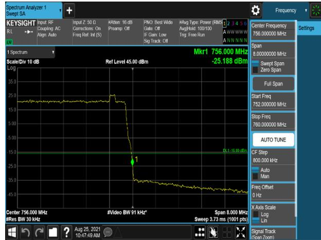
Plot 7-610. Band Edge Emission (756MHz to 756.1MHz) Plot (B13\_5M+NB-lot(IB)\_2C – High Channel, Port 1)
