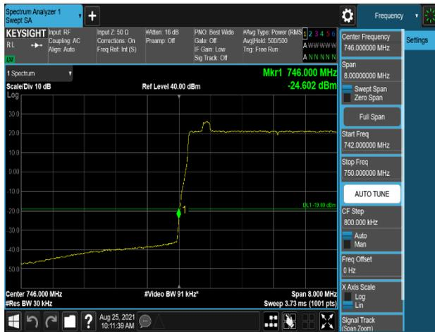
Plot 7-611. Band Edge Emission (745.9MHz to 746MHz) Plot (B13\_5M+NB-IoT(IB)\_2C – Port 1)
