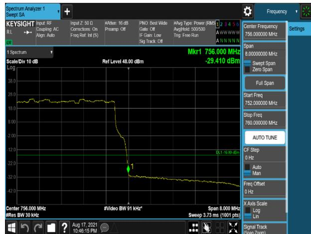
Plot 7-600. Band Edge Emission (756MHz to 756.1MHz) Plot (B13\_10M\_1C\_16QAM - High Channel, Port 1)
