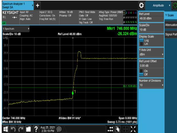
Plot 7-627. Band Edge Emission (745.9MHz to 746MHz) Plot (B13\_10M+Low\_NB-lot(IB)+High\_NB-lot(IB)\_1C – Port 0)
