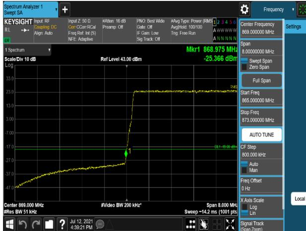
Plot 7-577. Band Edge Emission (868MHz to 869MHz) Plot (B5\_5M\_1C\_QPSK - Low Channel, Port 2)
