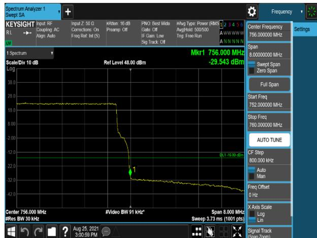
Plot 7-618. Band Edge Emission (756MHz to 756.1MHz) Plot (B13\_10M+Low\_NB-lot(IB)+Low\_NB-lot(IB)\_3C – Port 1)
