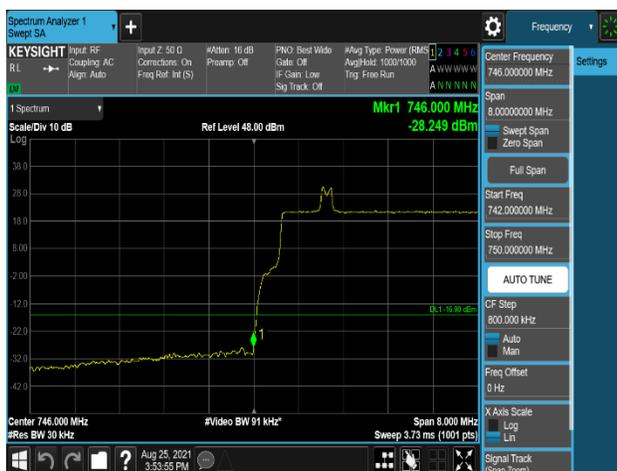
Plot 7-631. Band Edge Emission (745.9MHz to 746MHz) Plot (B13\_10M+High\_NB-lot(IB)+High\_NB-lot(IB)\_1C – Port 0)
