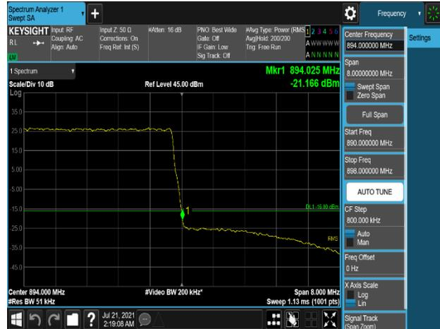
Plot 7 860. Band Edge Emission (894MHz to 895MHz) Plot (B5\_5M+5M\_2C\_256QAM\_Non-contiguous High Channel, Port 1)
