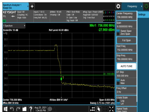
Plot 7-638. Band Edge Emission (756MHz to 756.1MHz) Plot (B13\_10M+High\_NB-lot(IB)+High\_NB-lot(IB)\_1C – Port 2)
