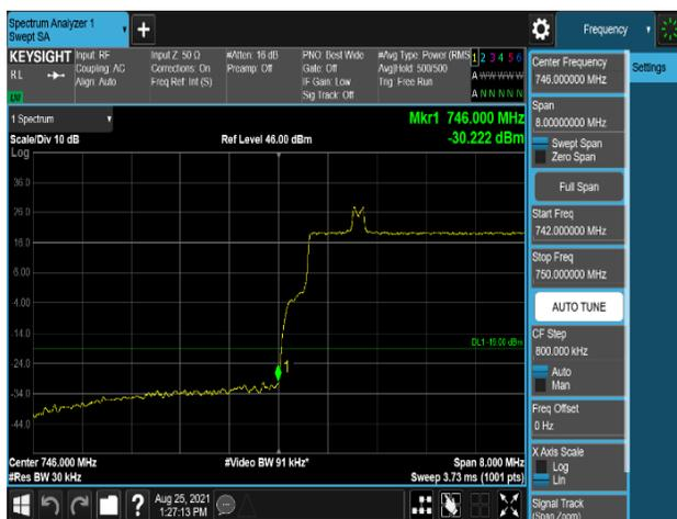
Plot 7-637. Band Edge Emission (745.9MHz to 746MHz) Plot (B13\_10M+High\_NB-lot(IB)+High\_NB-lot(IB)\_1C – Port 2)
