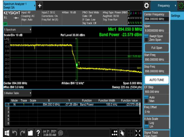
Plot 7-582. Band Edge Emission (894MHz to 895MHz) Plot (B5\_5M+5M\_2C\_QPSK - High Channel, Port 1)
