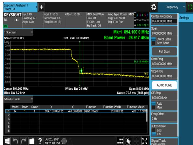
Plot 7-588. Band Edge Emission (894MHz to 895MHz) Plot (B5\_10M+10M\_2C\_QPSK - High Channel, Port 3)
