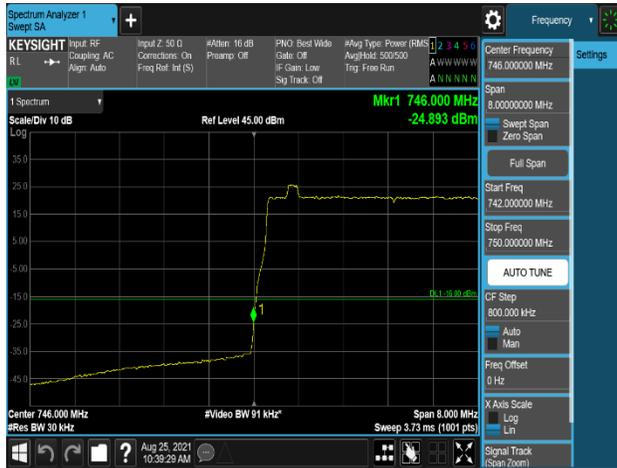
Plot 7-609. Band Edge Emission (745.9MHz to 746MHz) Plot (B13\_5M+NB-lot(IB)\_2C – Low Channel, Port 1)
