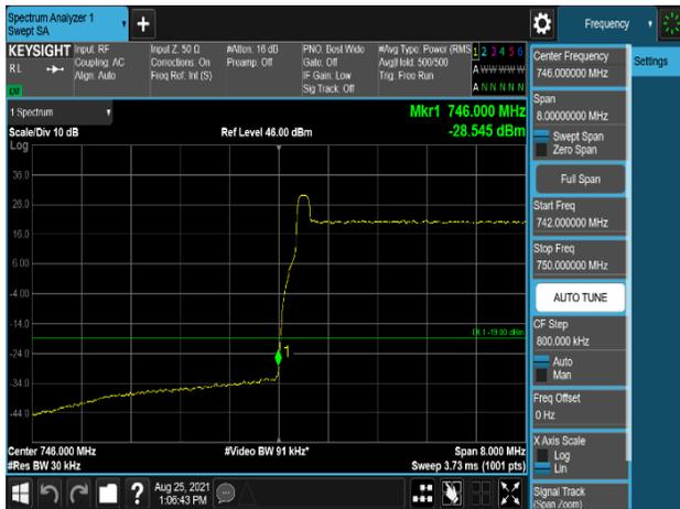
Plot 7-635. Band Edge Emission (745.9MHz to 746MHz) Plot (B13\_10M+Low\_NB-lot(IB)+Low\_NB-lot(IB)\_1C – Port 1)
