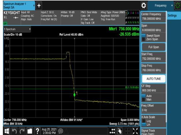
Plot 7-628. Band Edge Emission (756MHz to 756.1MHz) Plot (B13\_10M+Low\_NB-lot(IB)+High\_NB-lot(IB)\_1C – Port 1)
