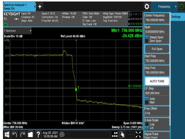
Plot 7-613. Band Edge Emission (745.9MHz to 746MHz) Plot (B13\_5M+NB-IoT(IB)\_2C – Port 1)
