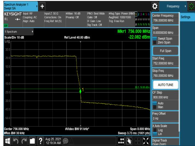
Plot 7-606. Band Edge Emission (756MHz to 756.1MHz) Plot (B13\_5M+5M\_2C\_256QAM - High Channel, Port 1)
