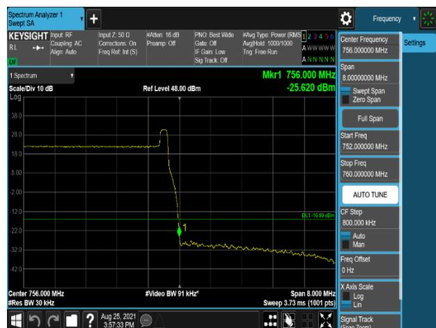
Plot 7-632. Band Edge Emission (756MHz to 756.1MHz) Plot (B13\_10M+High\_NB-lot(IB)+High\_NB-lot(IB)\_1C – Port 1)
