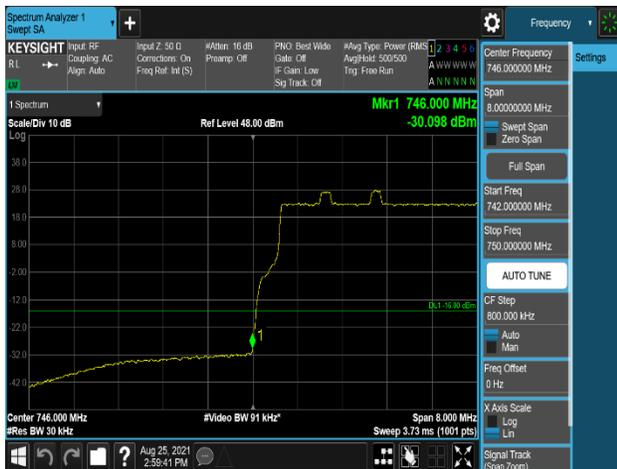
Plot 7-617. Band Edge Emission (745.9MHz to 746MHz) Plot (B13\_10M+Low\_NB-lot(IB)+Low\_NB-lot(IB)\_3C – Port 1)
