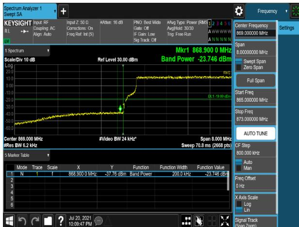
Plot 7-587. Band Edge Emission (868MHz to 869MHz) Plot (B5\_10M+10M\_2C\_64QAM - Low Channel, Port 3)
