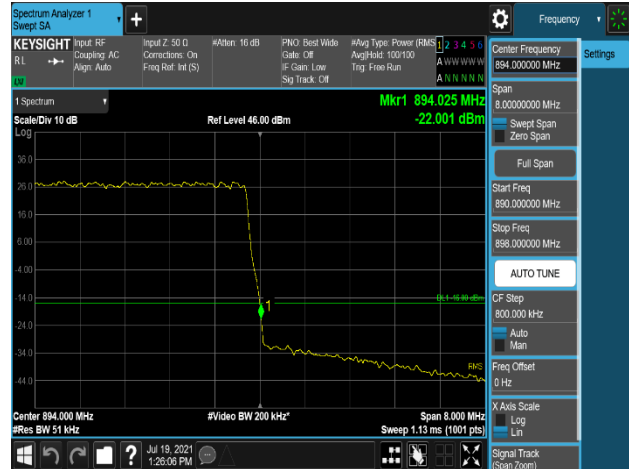
Plot 7-574. Band Edge Emission (894MHz to 895MHz) Plot (B5_5M_1C_64QAM - High Channel, Port 0)
