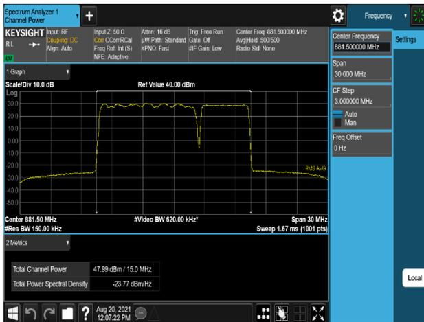
Plot 7-447. Conducted Average Output Power Plot (B5\_10M(DSS)+5M\_2C\_64QAM - Mid Channel, Port 0)
