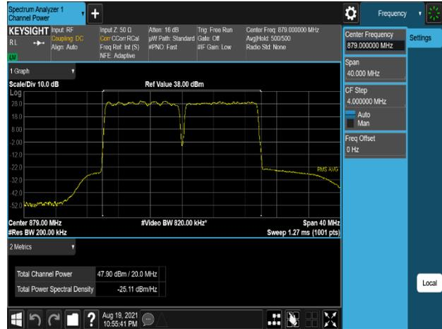
Plot 7-452. Conducted Average Output Power Plot (B5\_10M(DSS)+10M\_2C\_16QAM - Low Channel, Port 1)
