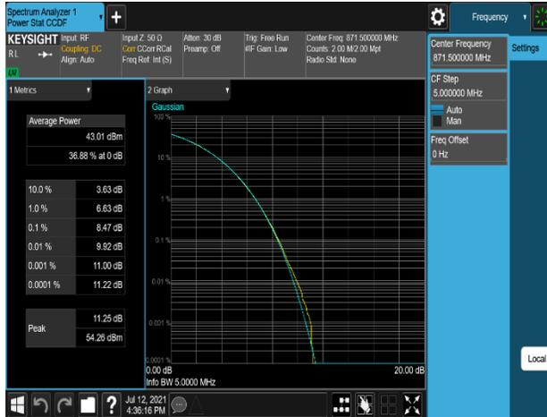
Plot 7-469. Peak To Average Power Ratio Plot (B5\_5M\_1C\_QPSK - Low Channel, Port 1)
