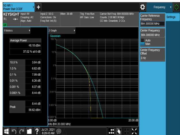
Plot 7-480. Peak To Average Power Ratio Plot (B5\_10M+10M\_2C\_16QAM - High Channel, Port 0)
