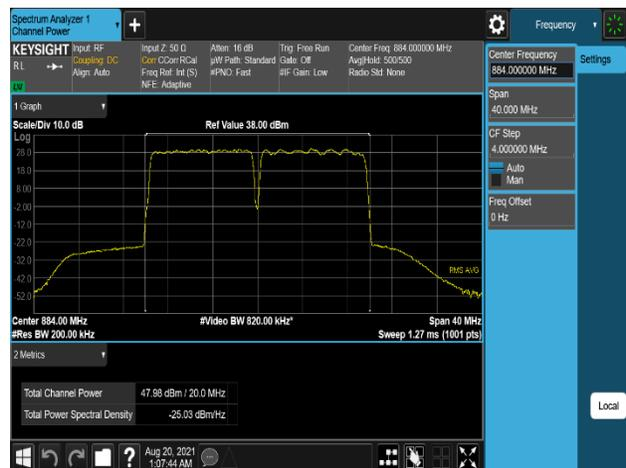
Plot 7-456. Conducted Average Output Power Plot (B5\_10M(DSS)+10M\_2C\_16QAM - High Channel, Port 1)
