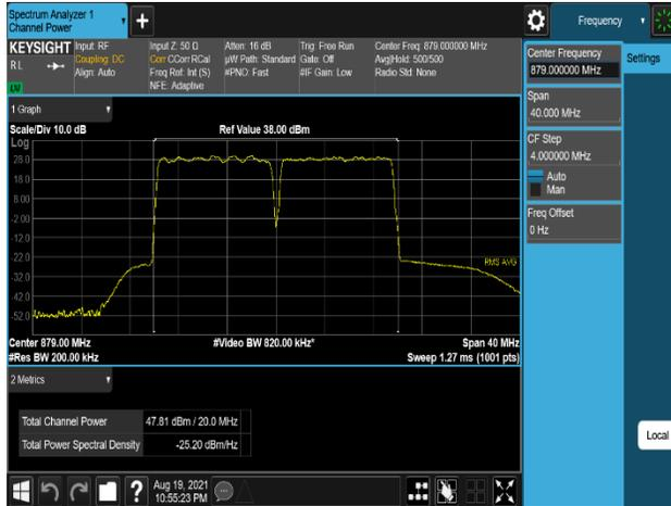
Plot 7-451. Conducted Average Output Power Plot (B5\_10M(DSS)+10M\_2C\_16QAM - Low Channel, Port 0)
