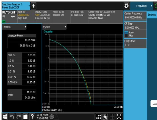
Plot 7-471. Peak To Average Power Ratio Plot (B5\_5M\_1C\_QPSK - High Channel, Port 1)
