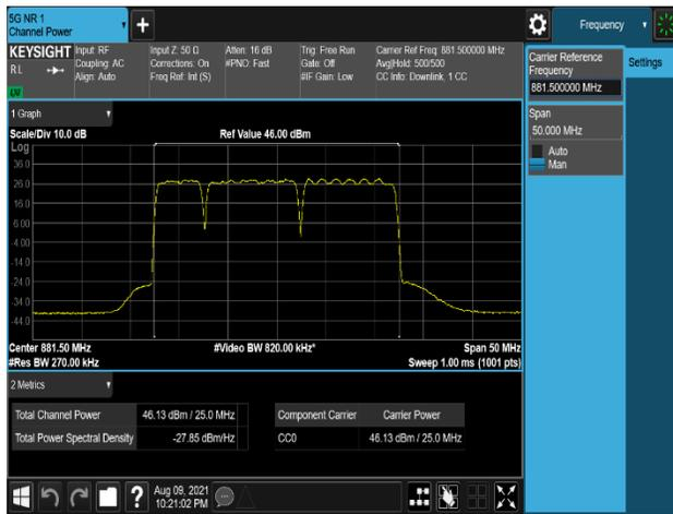
**Plot 7-457. Conducted Average Output Power Plot (B5\_10M(DSS)+10M+5M\_3C\_16QAM - Port 0)**
