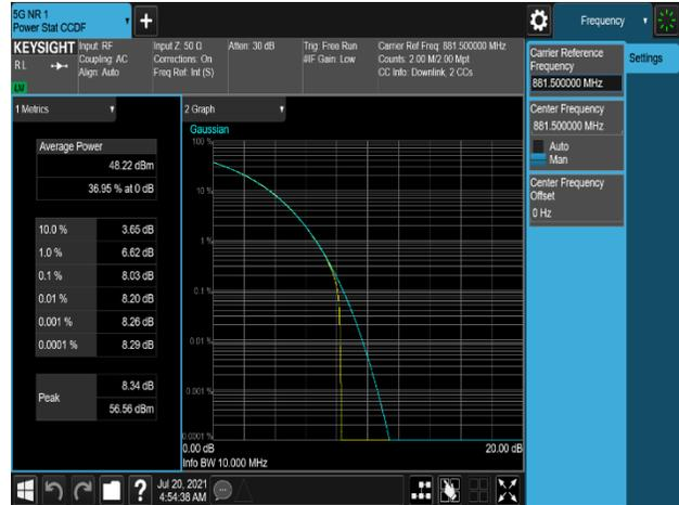
Plot 7-476. Peak To Average Power Ratio Plot (B5\_5M+5M\_2C\_QPSK - Mid Channel, Port 0)
