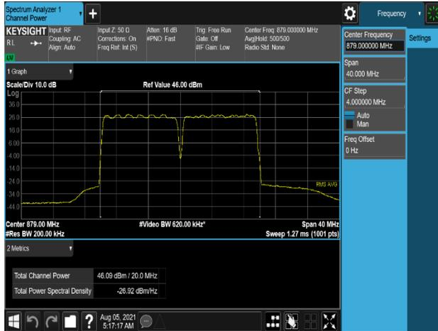
Plot 7-433. Conducted Average Output Power Plot (B5\_10M(DSS)+10M\_2C\_16QAM - Low Channel, Port 0)
