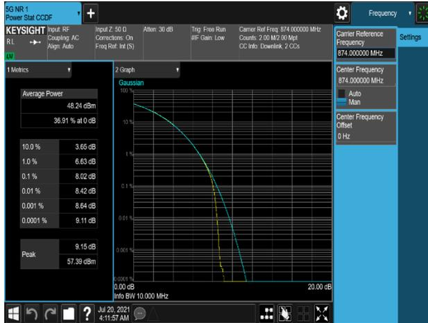
Plot 7-475. Peak To Average Power Ratio Plot (B5\_5M+5M\_2C\_QPSK - Low Channel, Port 1)
