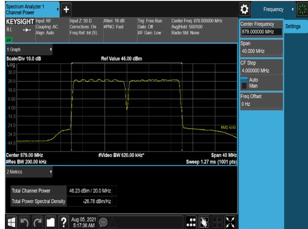
Plot 7-434. Conducted Average Output Power Plot (B5\_10M(DSS)+10M\_2C\_16QAM - Low Channel, Port 1)
