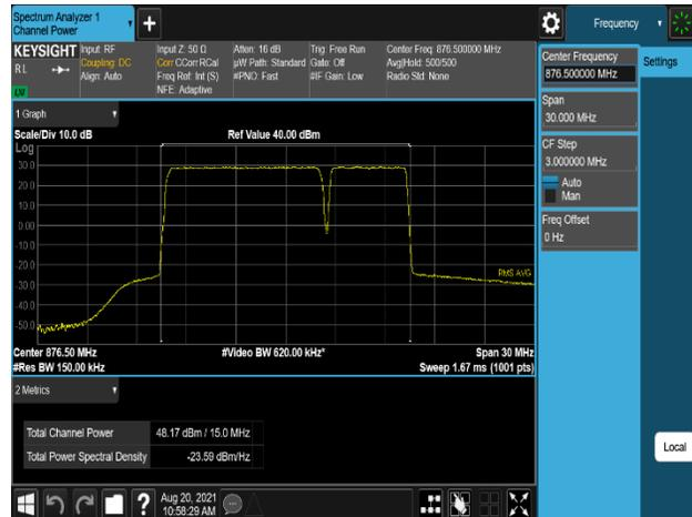
Plot 7-446. Conducted Average Output Power Plot (B5\_10M(DSS)+5M\_2C\_QPSK - Low Channel, Port 1)
