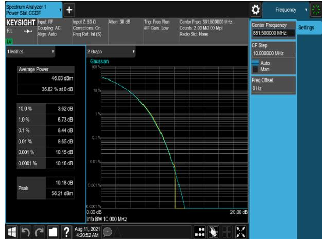
Plot 7-500. Peak To Average Power Ratio Plot (B5\_10M(DSS)\_1C\_256QAM - Middle Channel, Port 0)
