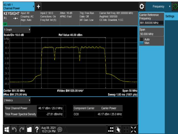
**Plot 7-458. Conducted Average Output Power Plot (B5\_10M(DSS)+10M+5M\_3C\_16QAM - Port 1)**
