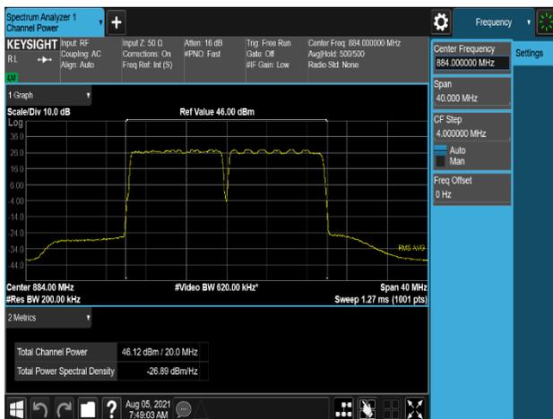
Plot 7-443. Conducted Average Output Power Plot (B5\_10M(DSS)+10M\_2C\_16QAM - High Channel, Port 2)
