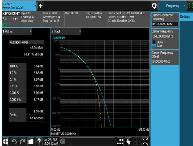
Plot 7-487. Peak To Average Power Ratio Plot (B5\_5M+10M+10M\_3C\_16QAM - Low Channel, Port 0)
