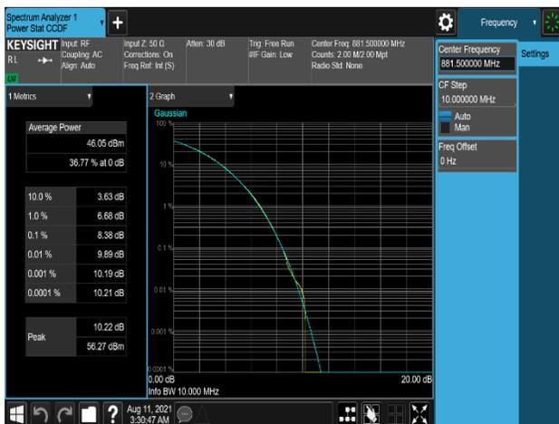
Plot 7-497. Peak To Average Power Ratio Plot (B5\_10M(DSS)\_1C\_QPSK - Middle Channel, Port 0)
