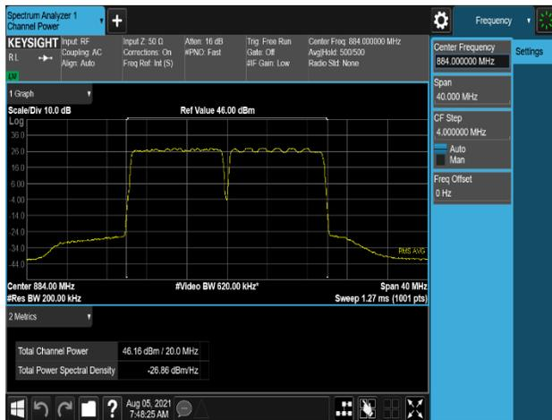
Plot 7-441. Conducted Average Output Power Plot (B5\_10M(DSS)+10M\_2C\_16QAM - High Channel, Port 0)
