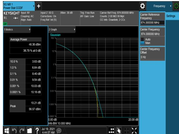
Plot 7-482. Peak To Average Power Ratio Plot (B5\_5M+5M\_2C\_QPSK - Mid Channel, Port 0)
