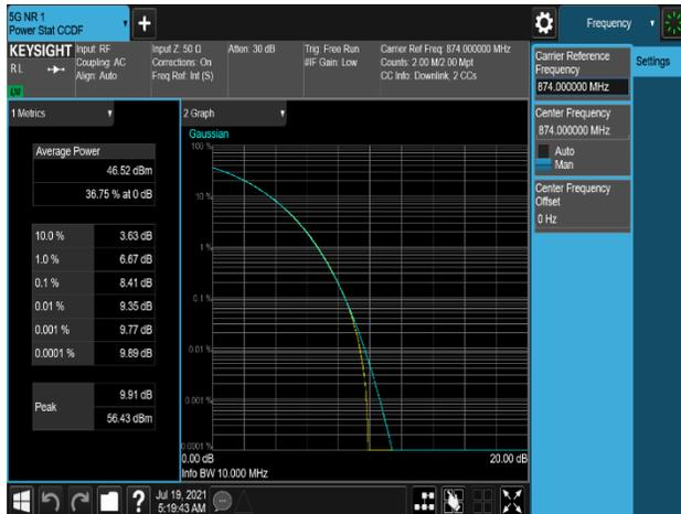
Plot 7-481. Peak To Average Power Ratio Plot (B5\_5M+5M\_2C\_64QAM - Low Channel, Port 1)
