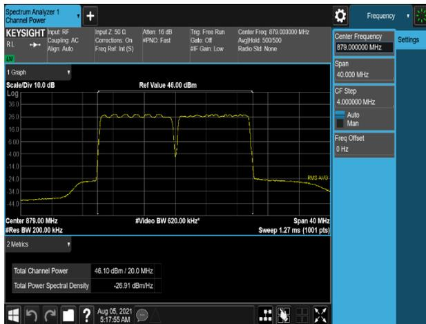
Plot 7-435. Conducted Average Output Power Plot (B5\_10M(DSS)+10M\_2C\_16QAM - Low Channel, Port 2)
