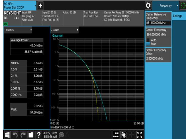
Plot 7-488. Peak To Average Power Ratio Plot (B5\_5M+10M+10M\_3C\_16QAM - Low Channel, Port 1)
