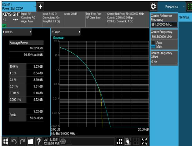
Plot 7-465. Peak To Average Power Ratio Plot (B5\_5M\_1C\_QPSK - High Channel, Port 1)
