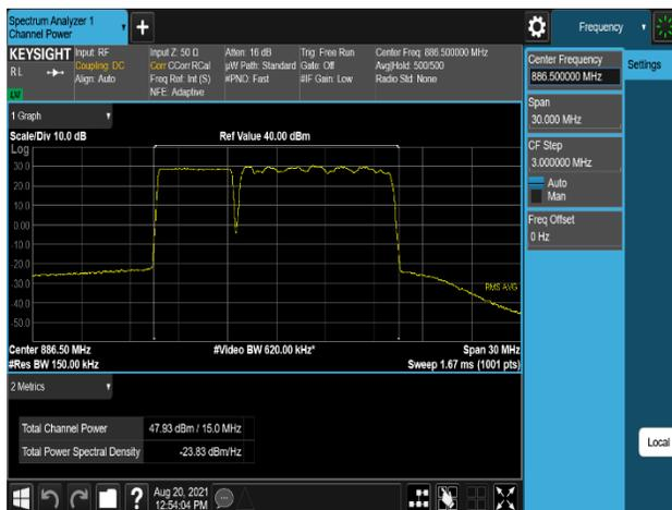
Plot 7-449. Conducted Average Output Power Plot (B5\_10M(DSS)+5M\_2C\_64QAM - High Channel, Port 0)
