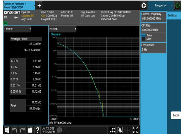
Plot 7-470. Peak To Average Power Ratio Plot (B5\_5M\_1C\_QPSK - Mid Channel, Port 0)
