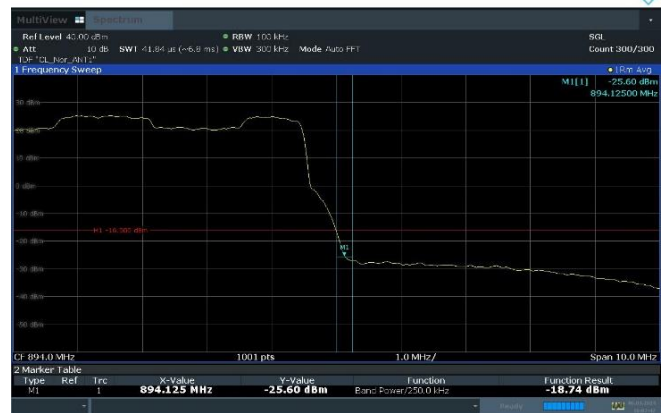
Plot 8-14. Band Edge Emission Summary Data Plot (n5_1C_25M_16QAM - High Edge_2T, Port 0)
