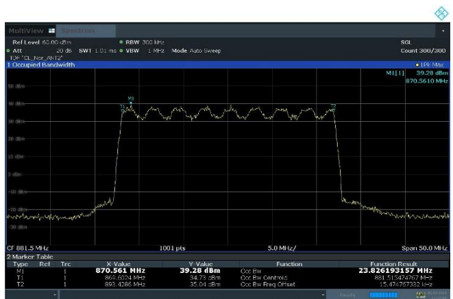
Plot 8-4. Occupied Bandwidth Plot (n5_1C_25M_4T_16QAM - Mid Channel, Port 2)
