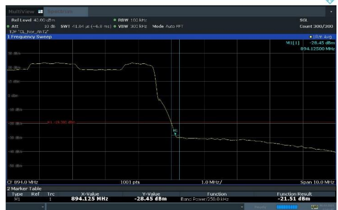
Plot 8-16. Band Edge Emission Summary Data Plot (n5_1C_25M_16QAM - High Edge_4T, Port 2)
