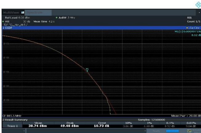
Plot 8-11. Peak To Average Power Ratio Plot (n5_1C_25M_2T_16QAM - Mid Channel, Port 1)
