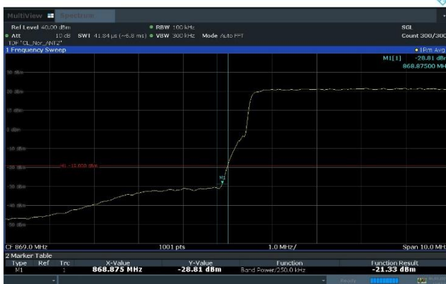
Plot 8-15. Band Edge Emission Summary Data Plot (n5_1C_25M_QPSK - Low Edge_4T, Port 2)
