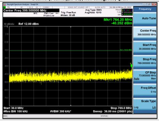
Antenna 2 / Low Edge - 100 MHz ~ Low Edge / (4 Port)(B5 DSS 10 MHz 1 Carrier + 5G NR n5 5 MHz 1 Carrier) + LTE B5 5 MHz 1 Carrier [3 Carrier](2C+1C) / Non-Contiguous / 256QAM
