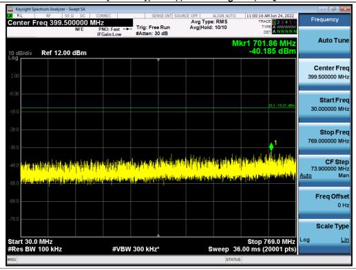
Antenna 0 / Low Edge - 100 MHz ~ Low Edge / (2 Port)(B5 DSS 10 MHz 1 Carrier + 5G NR n5 5 MHz 1 Carrier) + LTE B5 5 MHz 1 Carrier [3 Carrier](2C+1C) / Non-Contiguous / 16QAM
