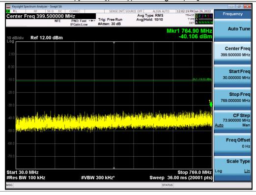
Antenna 2 / Low Edge - 100 MHz ~ Low Edge / (4 Port)B5 LTE 5 MHz 1 Carrier + (5G NR n5 5 MHz 1 Carrier + B5 DSS 10 MHz 1 Carrier) [3 Carrier](1C+2C) / Non-Contiguous / 16QAM
