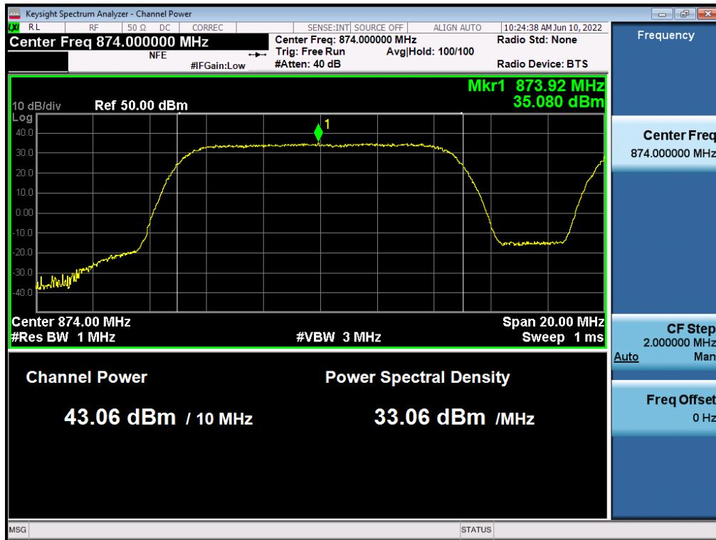
**Antenna 3 / (4 Port)B5 DSS 10 MHz 1 Carrier + 5G NR n5 10 MHz 1 Carrier [2 Carrier] / Non-Contiguous / 5G NR n5 10 MHz / 16QAM / High**
