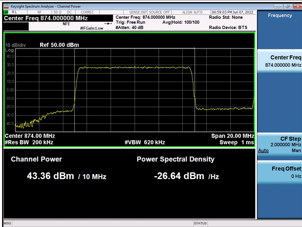
**Antenna 3 / (4 Port)5G NR n5 10 MHz 1 Carrier + 5G NR n5 10 MHz 1 Carrier [2 Carrier] / Non-Contiguous / 5G NR n5 10 MHz / QPSK / High**
