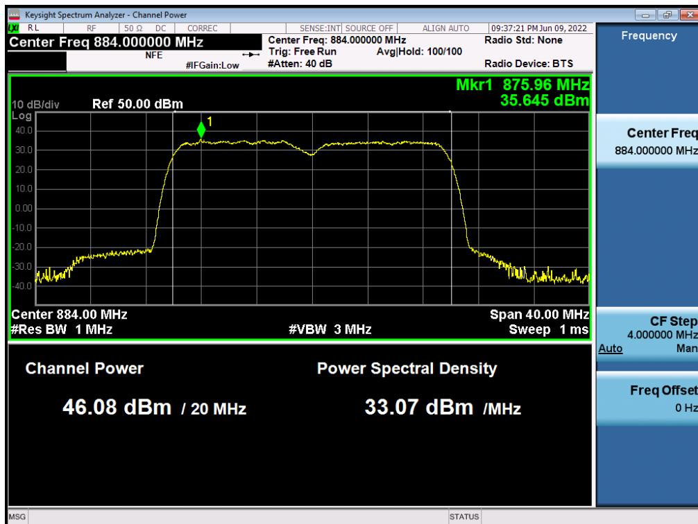
**Antenna 1 / (2 Port)5G NR n5 10 MHz 1 Carrier + 5G NR n5 10 MHz 1 Carrier + LTE B5 5 MHz 1 Carrier [3 Carrier] / Contiguous / 16QAM / Middle**
