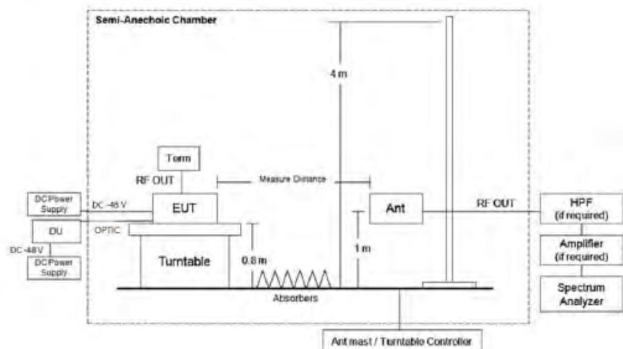
※ EUT position is adopted by placement of floor-standing refer to section 5.5.2.3.2 of ANSI C63.26-2015
