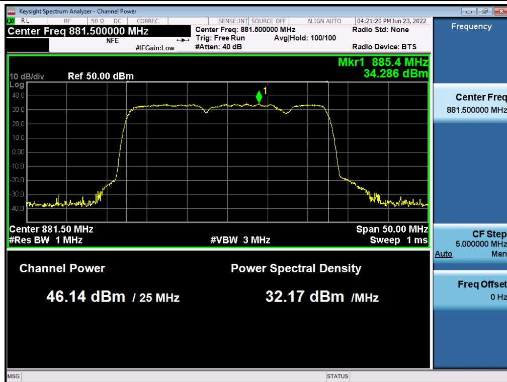
**Antenna 1 / (2 Port)5G NR n5 5 MHz 1 Carrier + 5G NR n5 5 MHz 1 Carrier [2 Carrier] / Non-Contiguous / 5G NR n5 5 MHz / QPSK / Low**
