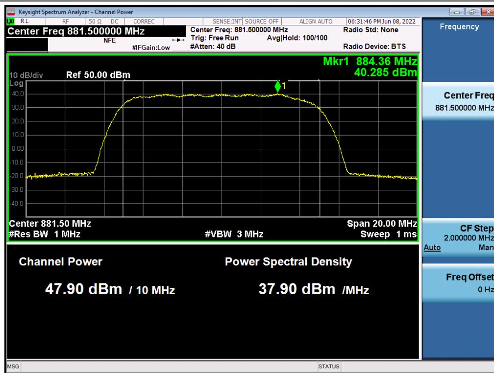
**Antenna 1 / (4 Port)5G NR n5 5 MHz 1 Carrier / 16QAM / Low**
