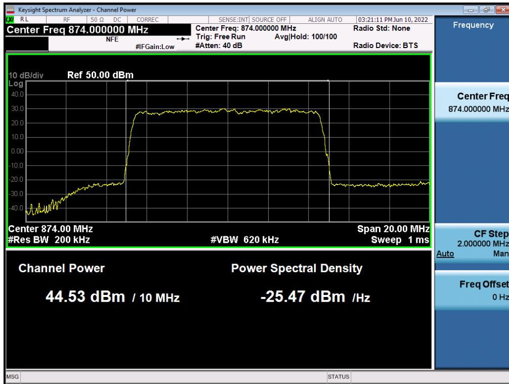
**Antenna 3 / (4 Port)B5 DSS 10 MHz 1 Carrier + 5G NR n5 5 MHz 1 Carrier [2 Carrier] / Non-Contiguous / 5G NR n5 5 MHz / 16QAM / High**
