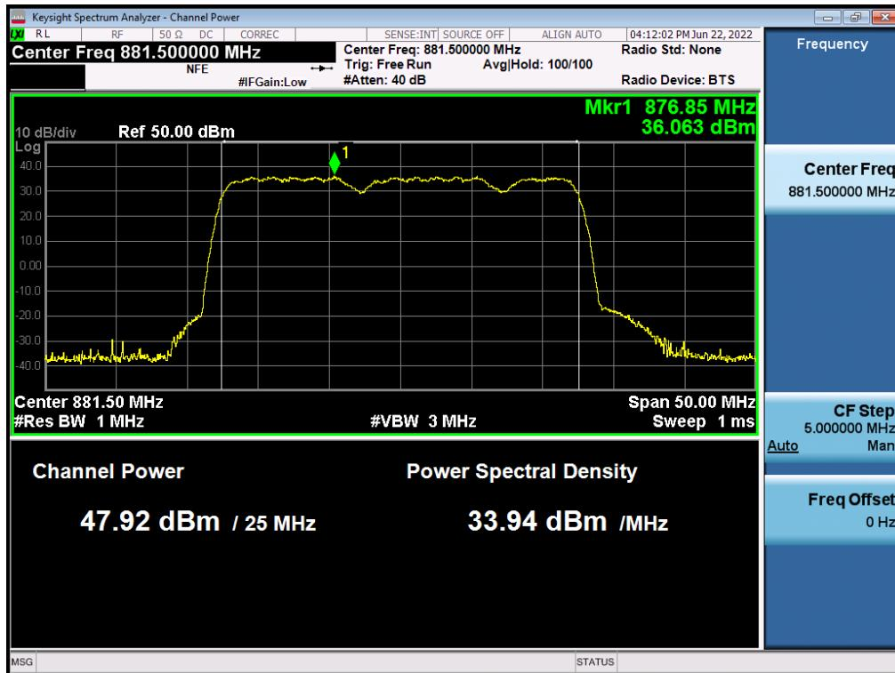
**Antenna 1 / (2 Port)B5 DSS 10 MHz 1 Carrier + 5G NR n5 5 MHz 1 Carrier + LTE B5 5 MHz 1 Carrier [3 Carrier] / Contiguous / 64QAM / Low**
