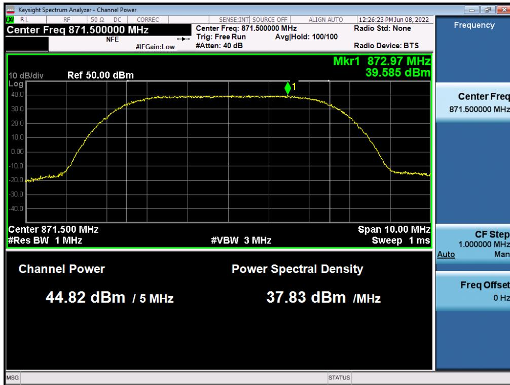
**Antenna 1 / (2 Port)5G NR n5 5 MHz 1 Carrier + 5G NR n5 5 MHz 1 Carrier [2 Carrier] / Non-Contiguous / 5G NR n5 5 MHz / QPSK / High**
