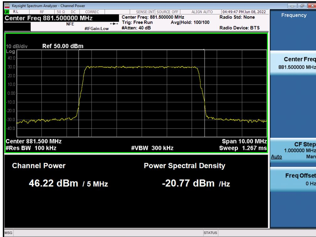
**Antenna 1 / (2 Port)5G NR n5 10 MHz 1 Carrier / 64QAM / Low**
