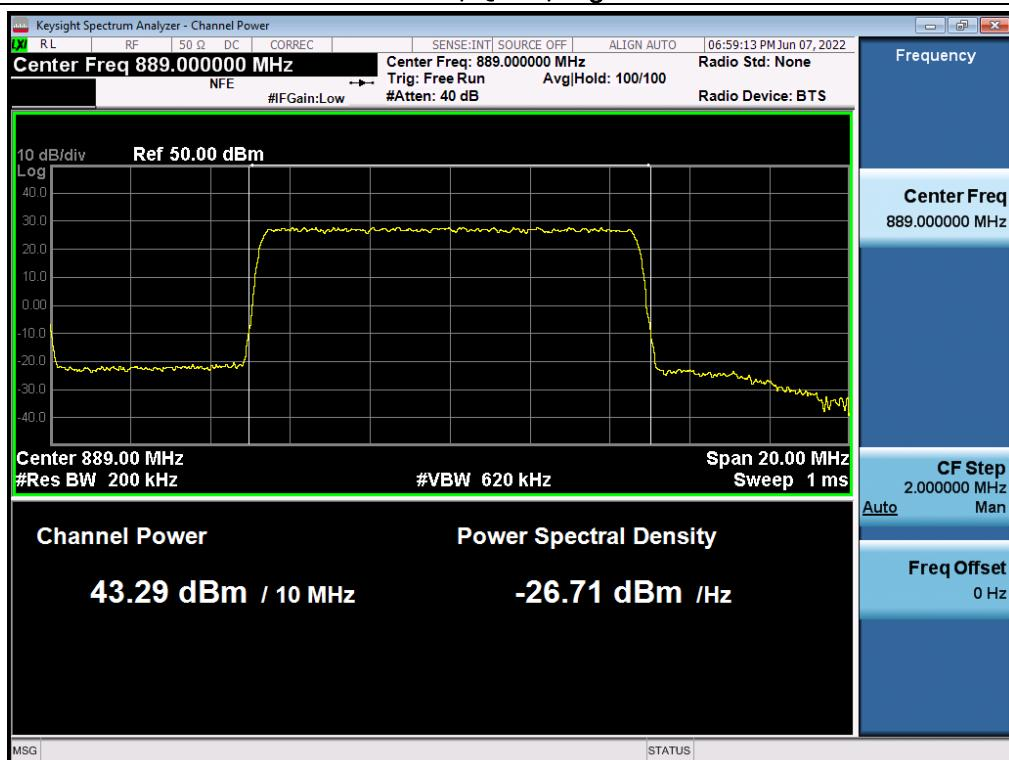
**Antenna 2 / (4 Port)B5 DSS 10 MHz 1 Carrier + B5 DSS 10 MHz 1 Carrier [2 Carrier] / Non-Contiguous / B5 DSS 10 MHz / 16QAM / Low**
