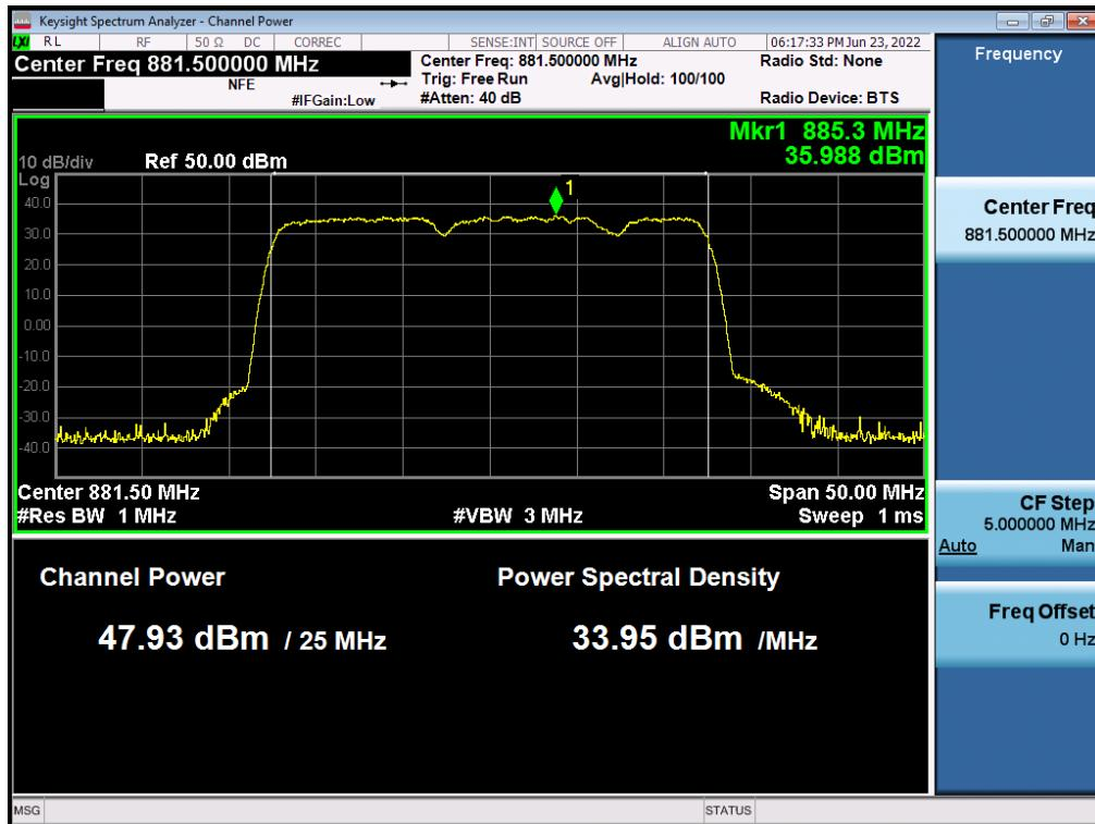
**Antenna 1 / (4 Port)5G NR n5 10 MHz 1 Carrier + 5G NR n5 10 MHz 1 Carrier + LTE B5 5 MHz 1 Carrier [3 Carrier] / Contiguous / 16QAM / Middle**
