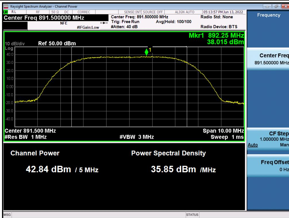
**Antenna 3 / (4 Port)B5 DSS 10 MHz 1 Carrier + 5G NR n5 5 MHz 1 Carrier [2 Carrier] / Non-Contiguous / B5 DSS 10 MHz / 16QAM / Low**
