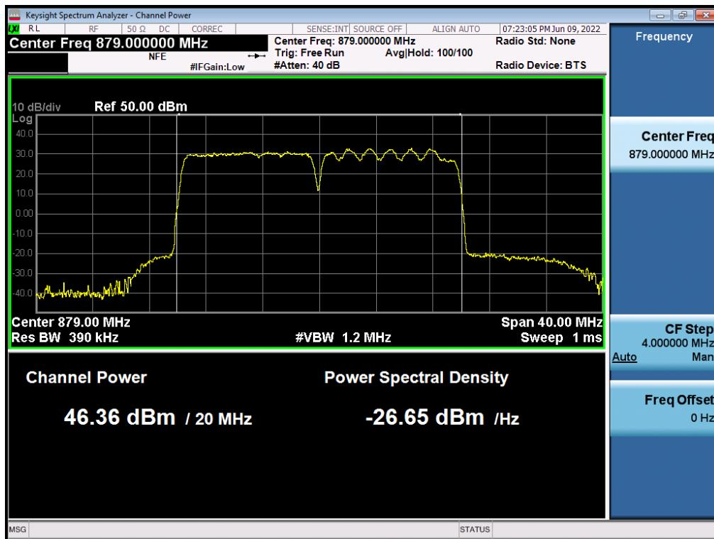
**Antenna 1 / (2 Port)5G NR n5 10 MHz 1 Carrier + 5G NR n5 10 MHz 1 Carrier + LTE B5 5 MHz 1 Carrier [3 Carrier] / Contiguous / 256QAM / Middle**
