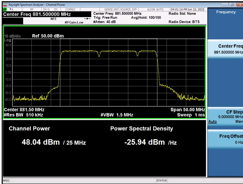
**Antenna 1 / (2 Port)B5 DSS 10 MHz 1 Carrier + 5G NR n5 5 MHz 1 Carrier + LTE B5 5 MHz 1 Carrier [3 Carrier] / Contiguous / 256QAM / Low**
