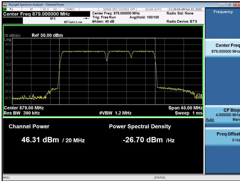
**Antenna 3 / (4 Port)B5 DSS 10 MHz 1 Carrier + 5G NR n5 10 MHz 1 Carrier + LTE B5 5 MHz 1 Carrier [3 Carrier] / Contiguous / 16QAM / Middle**
