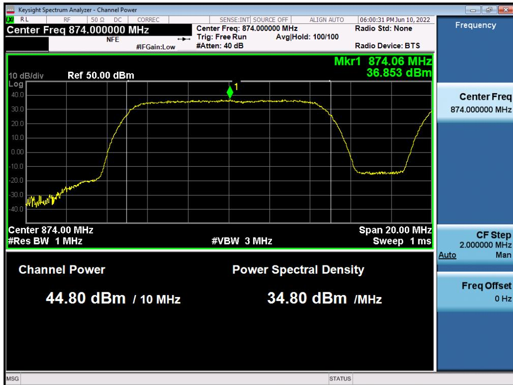
**Antenna 1 / (2 Port)B5 DSS 10 MHz 1 Carrier + 5G NR n5 10 MHz 1 Carrier [2 Carrier] / Non-Contiguous / 5G NR n5 10 MHz / 16QAM / High**
