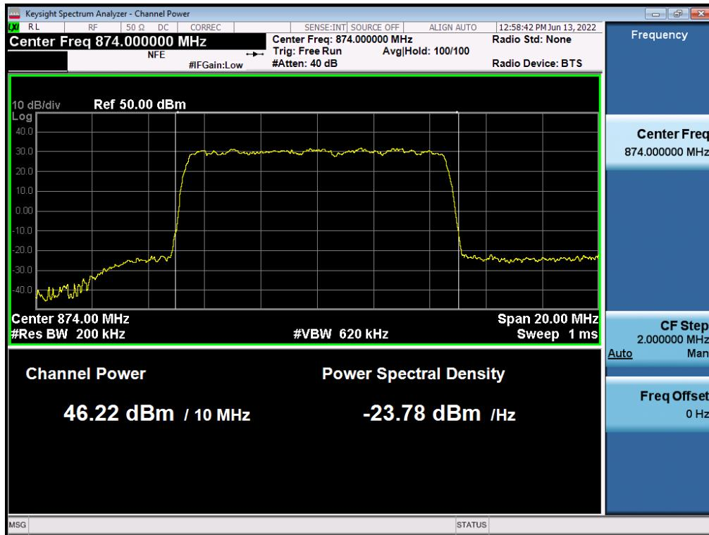
**Antenna 1 / (2 Port)B5 DSS 10 MHz 1 Carrier + 5G NR n5 5 MHz 1 Carrier [2 Carrier] / Non-Contiguous / 5G NR n5 5 MHz / 16QAM / High**
