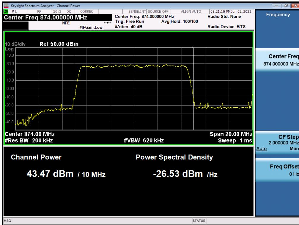
**Antenna 2 / (4 Port)B5 DSS 10 MHz 1 Carrier + B5 DSS 10 MHz 1 Carrier [2 Carrier] / Non-Contiguous / B5 DSS 10 MHz / 16QAM / High**
