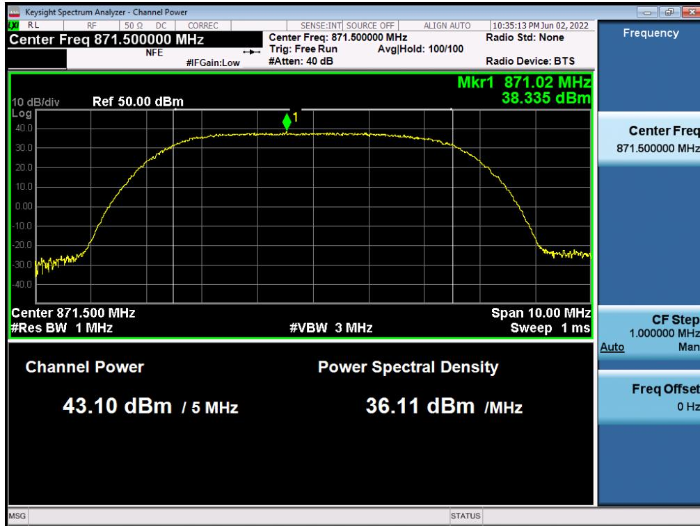
**Antenna 3 / (4 Port)5G NR n5 10 MHz 1 Carrier / 16QAM / Low**
