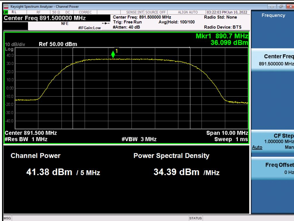
**Antenna 3 / (4 Port)B5 DSS 10 MHz 1 Carrier + 5G NR n5 10 MHz 1 Carrier [2 Carrier] / Non-Contiguous / B5 DSS 10 MHz / 16QAM / Low**
