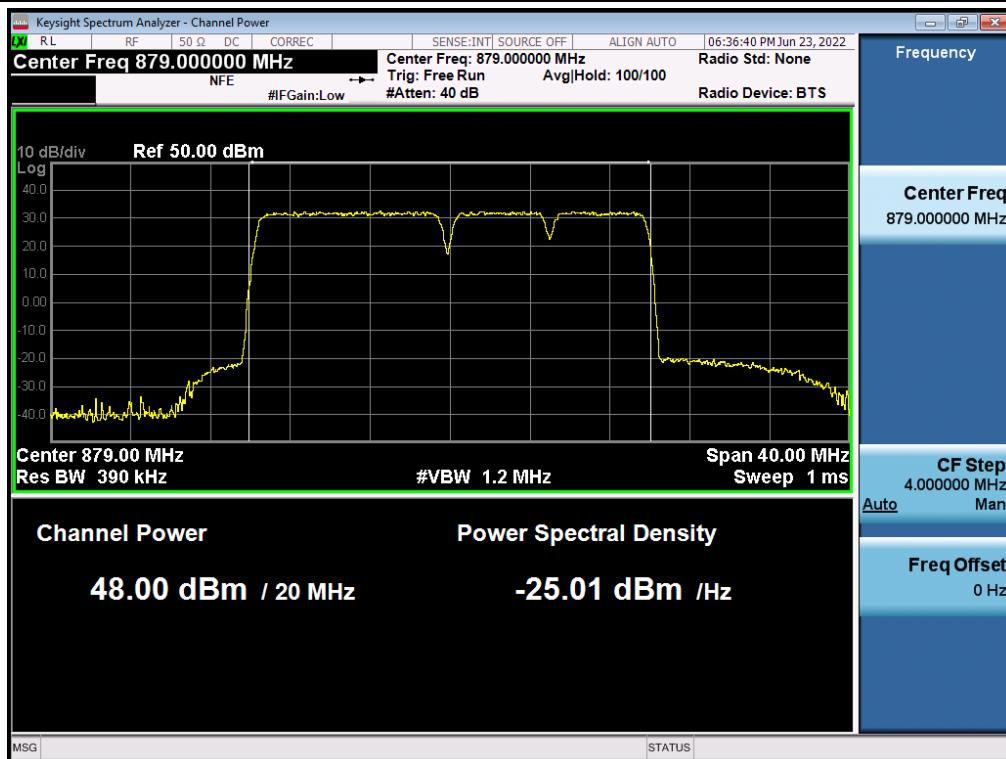
**Antenna 1 / (2 Port)B5 DSS 10 MHz 1 Carrier + 5G NR n5 10 MHz 1 Carrier + LTE B5 5 MHz 1 Carrier [3 Carrier] / Contiguous / 64QAM / Middle**
