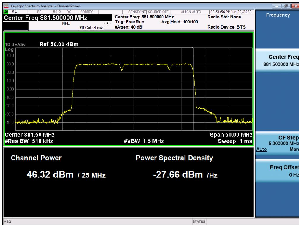
**Antenna 0 / (4 Port)B5 DSS 10 MHz 1 Carrier + 5G NR n5 5 MHz 1 Carrier + LTE B5 5 MHz 1 Carrier [3 Carrier] / Contiguous / 64QAM / Low**
