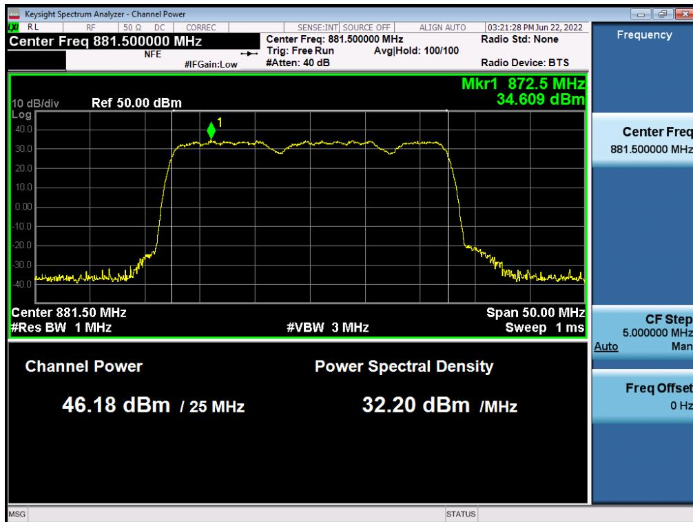
**Antenna 3 / (4 Port)B5 DSS 10 MHz 1 Carrier + 5G NR n5 5 MHz 1 Carrier + LTE B5 5 MHz 1 Carrier [3 Carrier] / Contiguous / 16QAM / Low**
