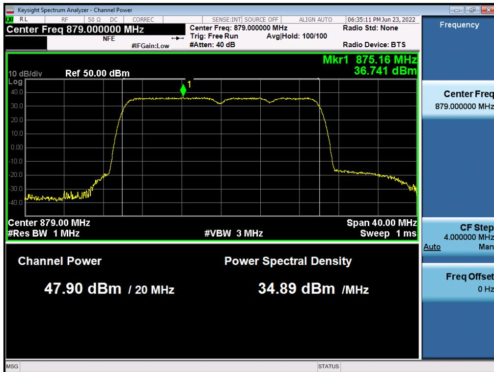
**Antenna 1 / (2 Port)B5 DSS 10 MHz 1 Carrier + 5G NR n5 10 MHz 1 Carrier + LTE B5 5 MHz 1 Carrier [3 Carrier] / Contiguous / 16QAM / Middle**
