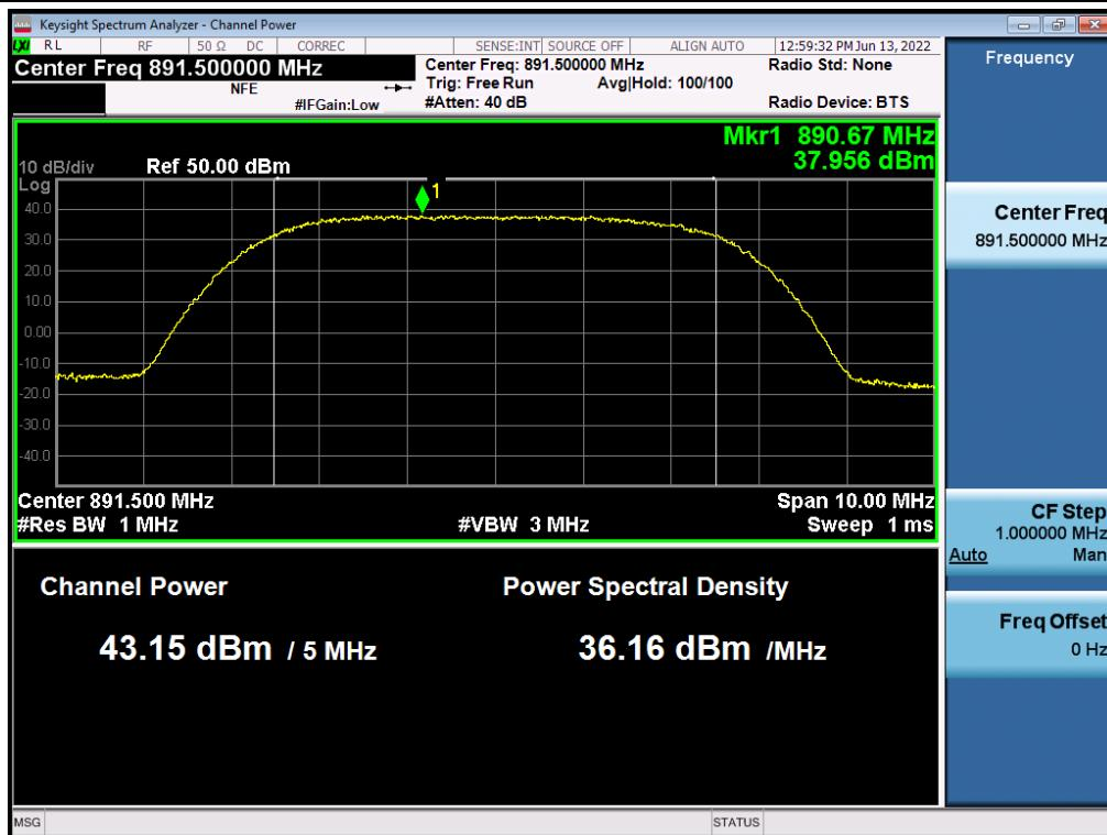
**Antenna 1 / (2 Port)B5 DSS 10 MHz 1 Carrier + 5G NR n5 10 MHz 1 Carrier [2 Carrier] / Non-Contiguous / B5 DSS 10 MHz / 16QAM / Low**
