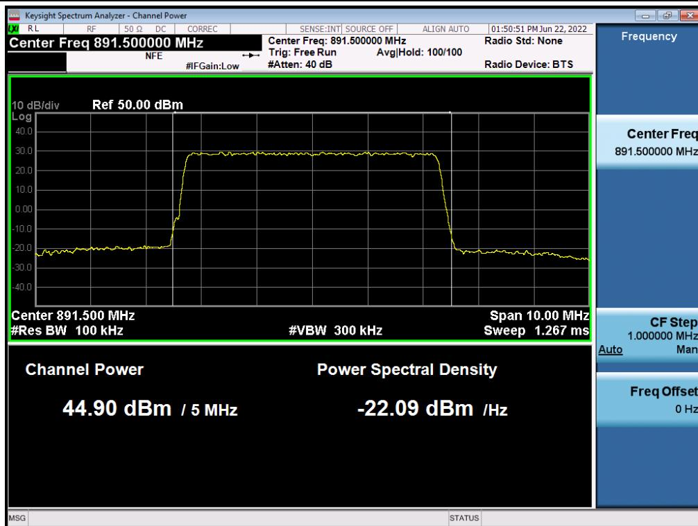
**Antenna 1 / (2 Port)B5 DSS 10 MHz 1 Carrier + 5G NR n5 5 MHz 1 Carrier [2 Carrier] / Non-Contiguous / B5 DSS 10 MHz / 16QAM / Low**
