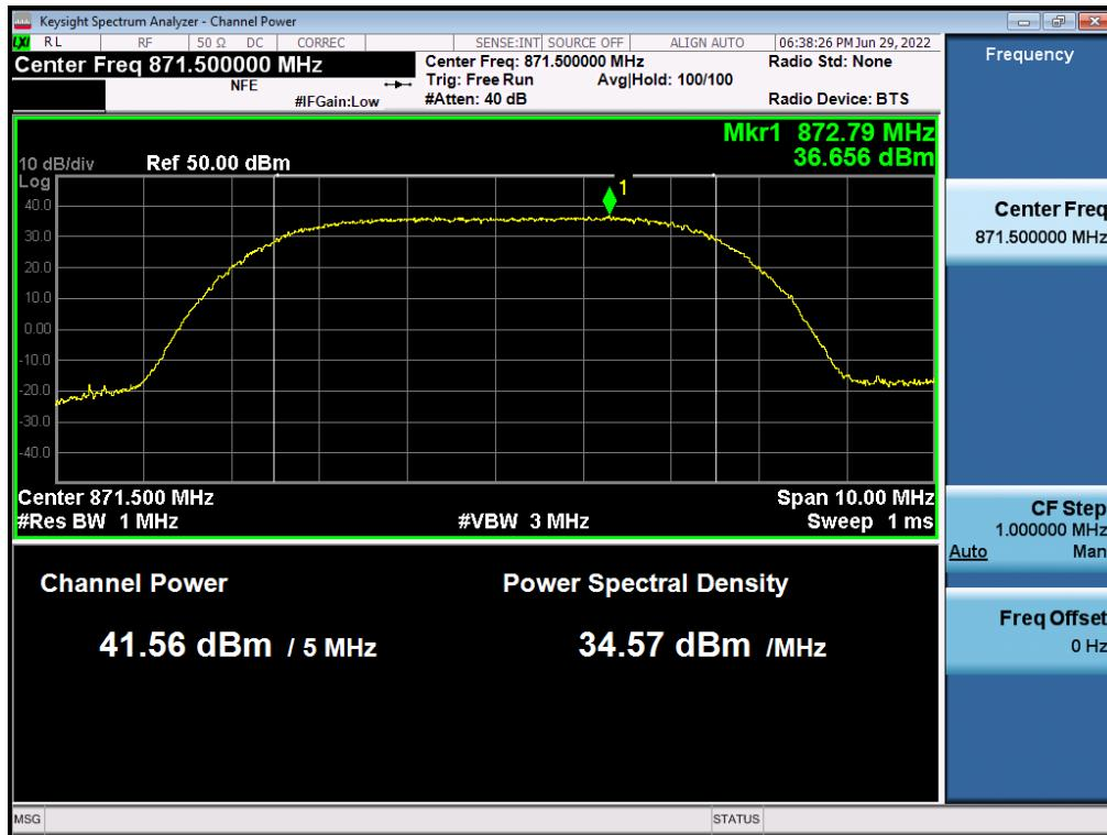
**Antenna 0 / (2 Port)B5 LTE B5 5 MHz 1 Carrier + (5G NR n5 5 MHz 1 Carrier + B5 DSS 10 MHz 1 Carrier) [3 Carrier](1C+2C)
