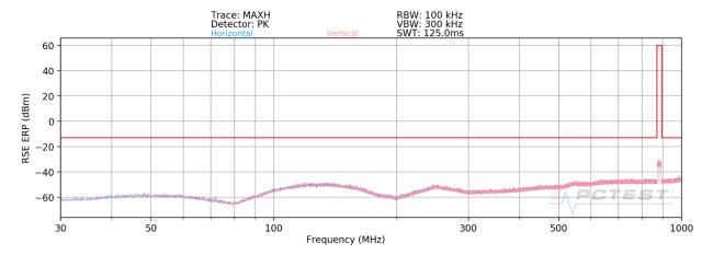
Plot 7-913. Radiated spurious emission\_30 MHz to 1000 MHz (DSS\_B5\_10M+10M\_2C\_Mid Channel)
